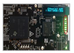
6 Observe that the message 'EtherCAT APP' appears on the OLED display. Also observe the LEDs for the pattern shown in the picture above to confirm that EtherCAT application has started.
