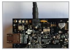
**5** Apply +24V to the K2G ICE with either a bench power supply or with a +24V power supply purchased separately.
