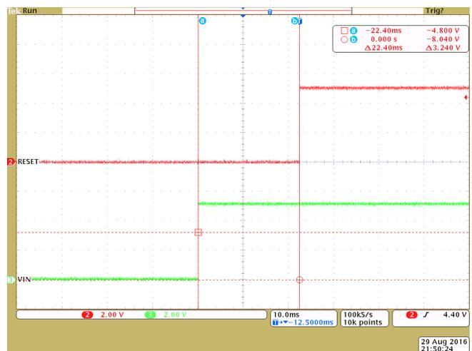
**Figure 10. Delay Time TPS3813I50-Q1**
