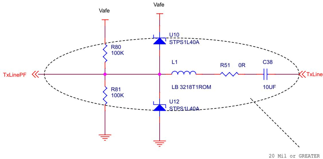
Figure 3. AFE2 (Passive TX Filter) Schematic
