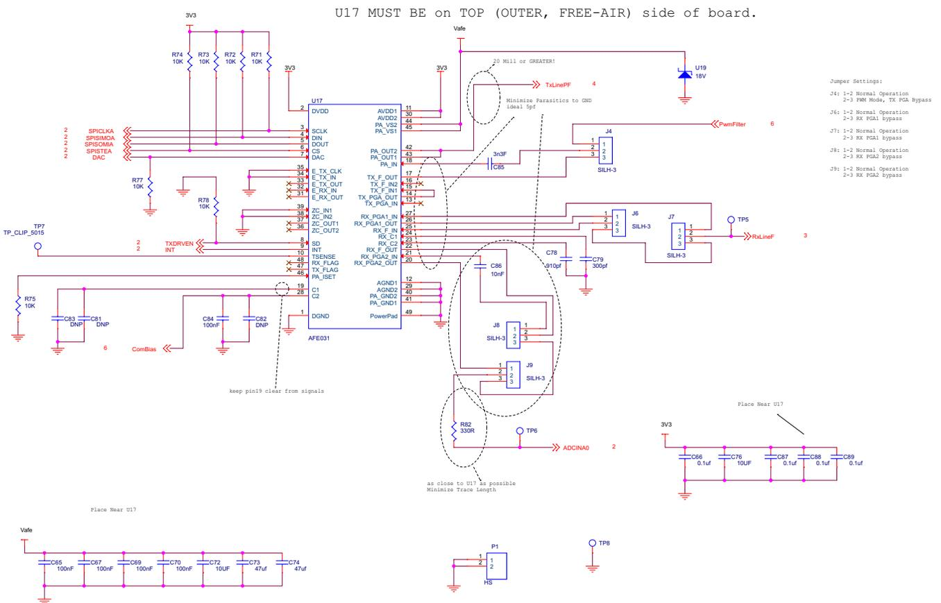
Figure 4. AFE031 Schematic
