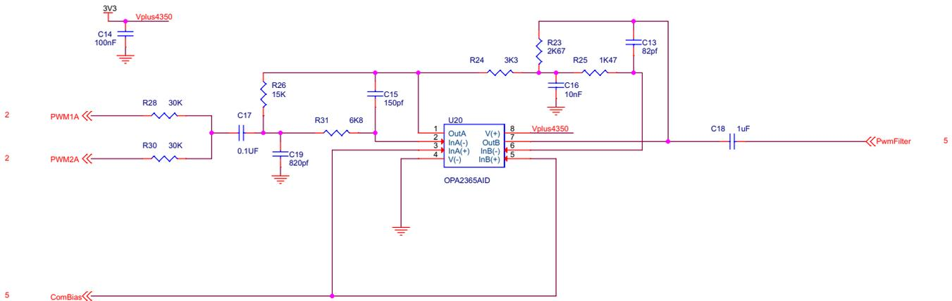
**Figure 5. PWM Filter Schematic**
