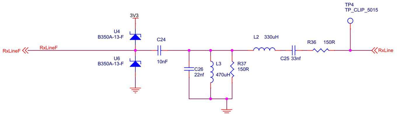
Figure 2. AFE1 (Passive RX Filter) Schematic
