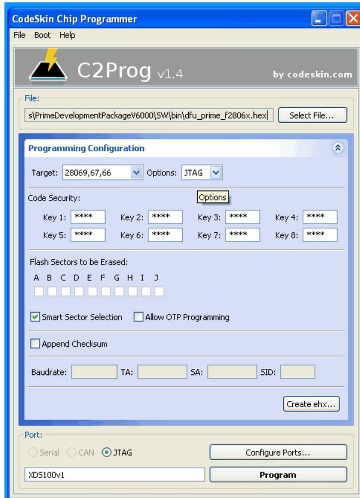
**Figure 4. Programming Configuration Using XDS100**
