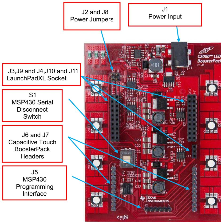
Figure 9. LED BoosterPack Jumper, Connector, and Switch Locations
