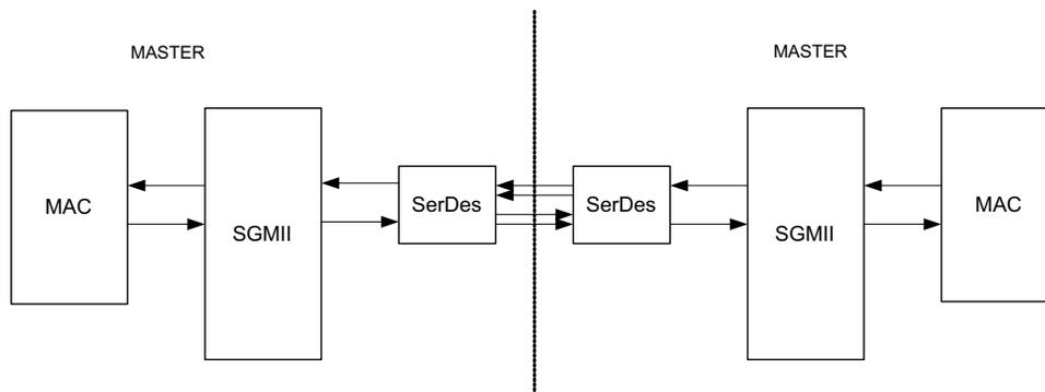
When connecting two SGMII devices with forced link, both SGMII devices must be configured as masters.
