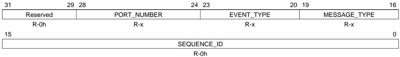
Legend: R = Read only; R/W = Read/Write; - n = value after reset; -x, value is indeterminate — see the device-specific data manual
