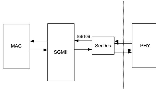
To connect with an external PHY, the PHY will be the master, and the SGMII module needs to be configured in slave mode. The procedure for setting the SGMII in slave mode is shown below:
