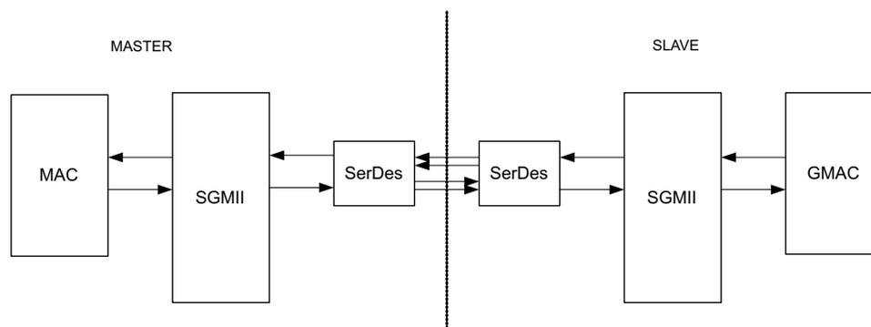
When connecting two SGMII devices with auto-negotiation, one SGMII device must be configured as the master, and the other SGMII device must be configured as the slave.
