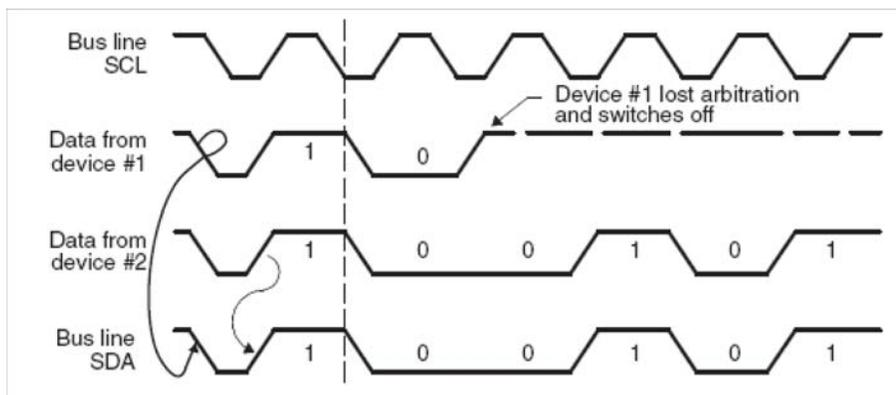
The first master-transmitter, which drives SDA high, is overruled by another master-transmitter that drives SDA low. The arbitration procedure gives priority to the device that transmits the serial data stream with the lowest binary value. Should two or more devices send identical first bytes, arbitration continues on the subsequent bytes.
