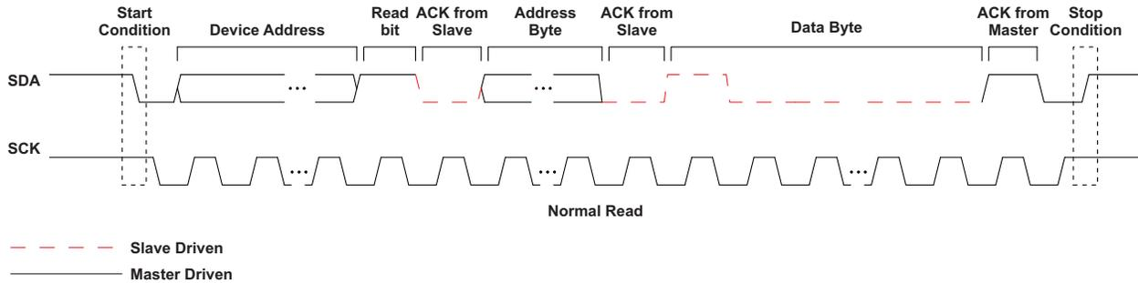
If a reset to the master device occurs during the data transfer of a read cycle, there is the possibility of the bus ending in a state that will prevent any master from regaining control. Consider the situation shown in Figure A-3.
