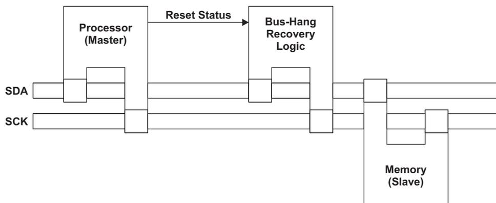
The bus-hang recovery logic needs to have knowledge of the reset status of the processor either through a RESETSTAT or a GPIO signal as well as the ability to monitor and drive the SDA and SCK signals. This logic may be a state machine in a programmable logic device or a software-driven solution in a microcontroller or processor using GPIO pins, but it must meet the open-collector driver requirements for the SDA and SCK signals to ensure the proper operation of the  $I^2C$ .
