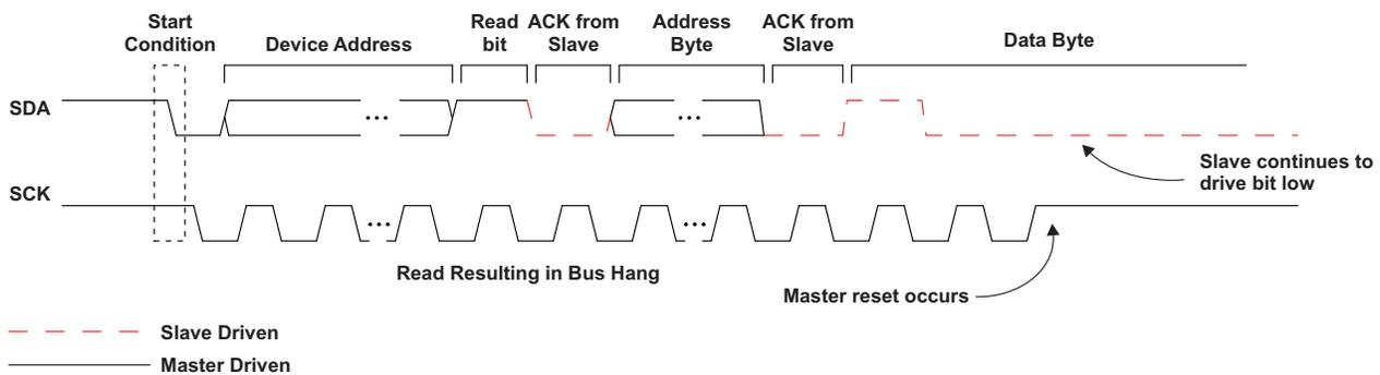
The master initiates a read in the normal fashion but a reset occurs while the SCK is high and the slave is driving the SDA low. The slave device will continue to drive SDA low waiting for the master to provide the next clock however the master has been reset and is no longer attempting to complete the read cycle. In addition, if the master attempts to access the bus after its reset has been released it will fail to arbitrate for control.
