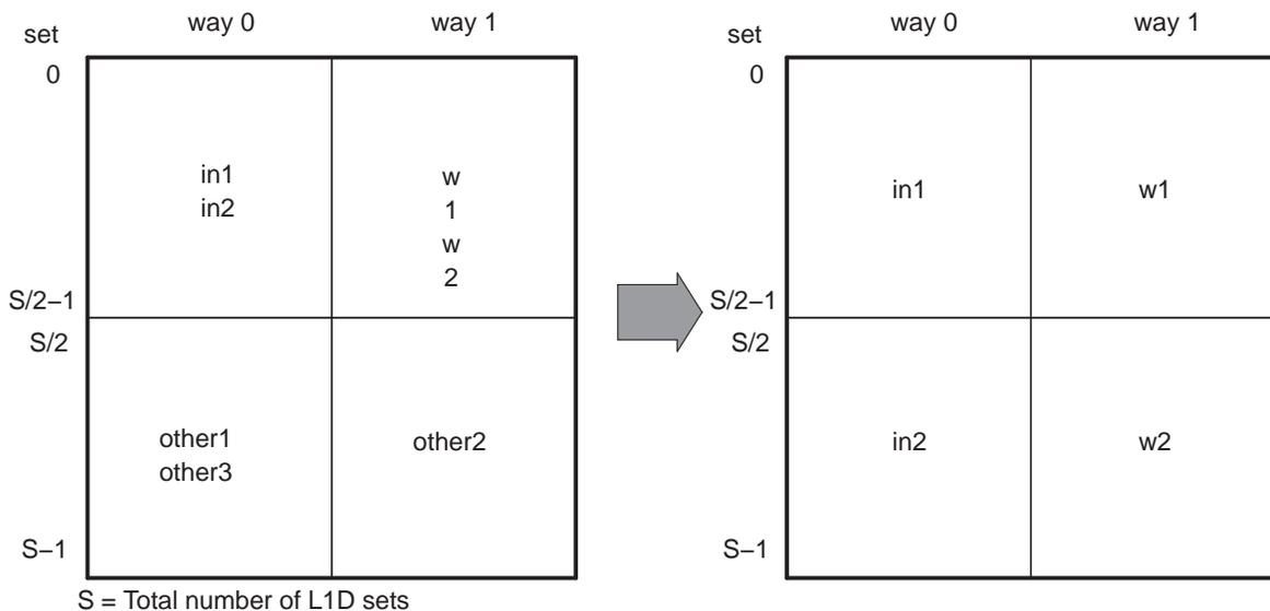
The first call to dotprod allocates in1 and w1 into L1D, as shown in Figure 3-6. This causes S compulsory misses, where S is the total number of sets. The second call causes in1 and w1 to be evicted and replaced with in2 and w2, which causes another S misses. The third call reuses w2, but replaces in2 with in1 resulting in S/2 misses. Finally, the last call again causes S misses, because in1 and w2 are replaced with in2 and w1.
