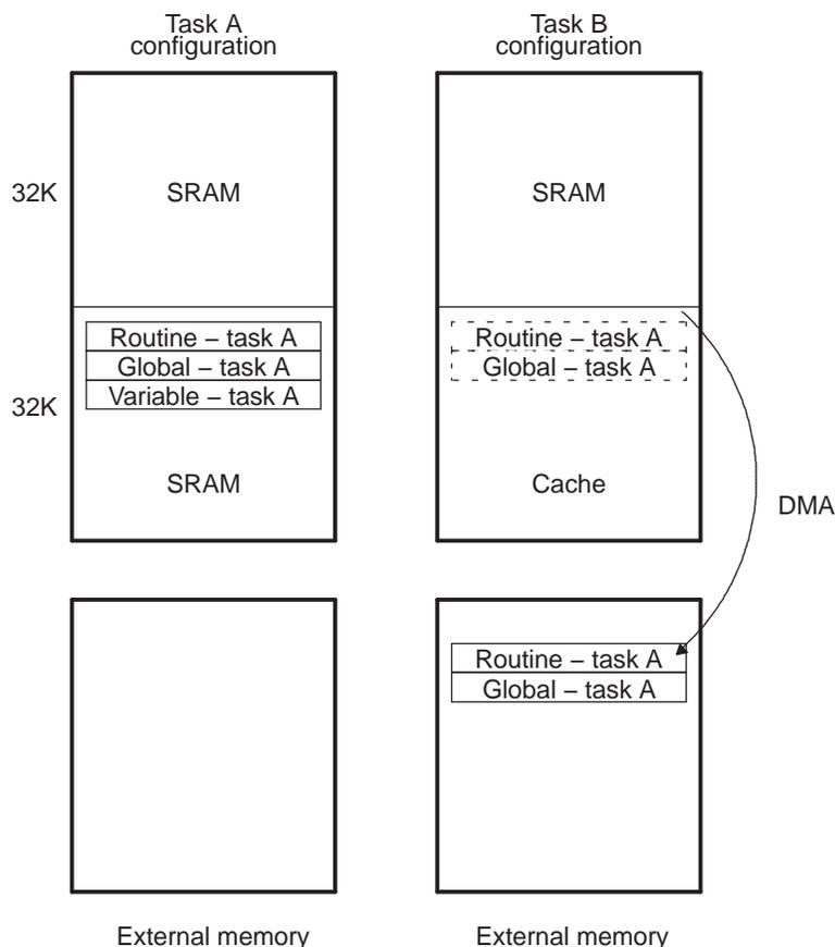
To switch back to task A configuration, L2 cache line frames located in the 32K byte segment that is to be switched to SRAM have to be written back to external memory and invalidated. Since it is not known which external memory addresses are cached in these line frames, all of L2 is writeback–invalidated. This is automatically done by the cache controller when the cache size is switched. Code and global variables can then be copied back to their original location.
