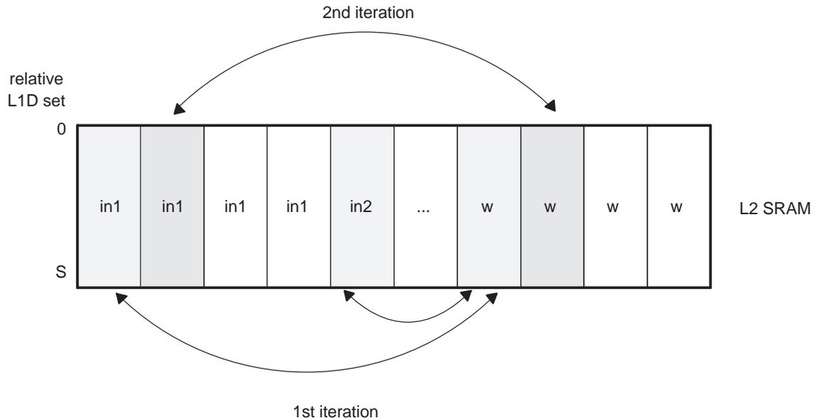
We can further reduce the number of read miss stalls by exploiting miss pipelining. The touch loop is used to allocate `w[ ]` once at the start of the iteration; then before each call of `dotprod`, the required input array is allocated:
