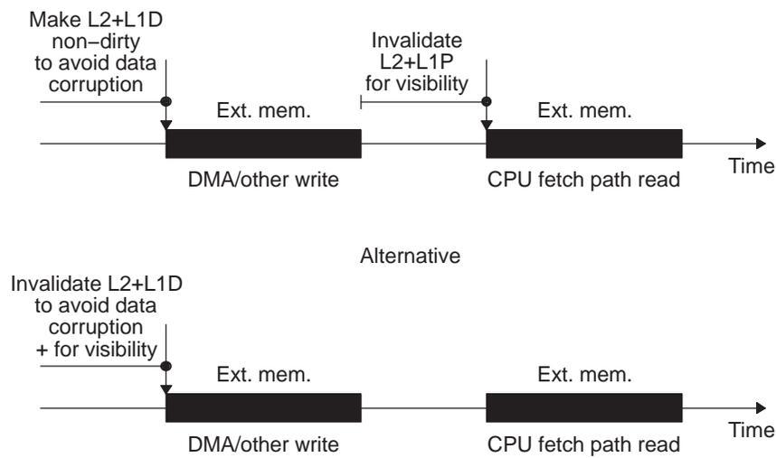
**Figure A-3. External Memory: CPU Write, DMA Read (Data)**
