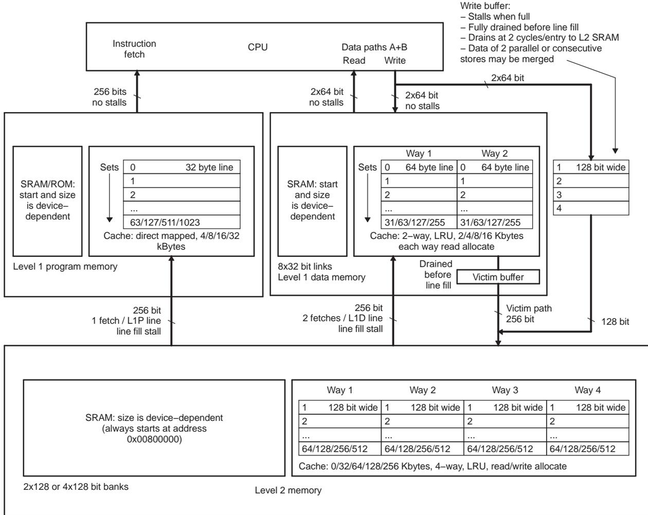
Table 3-1 and Table 3-2 list the actual stall cycles for two different device configurations. One configuration is for devices that have an L2 with 0 wait-states and 2 × 128-bit banks. The other configuration is for devices that have an L2 with 1 wait-state and 4 × 128-bit banks. See your device-specific data manual to determine the L2 type for a particular device.
