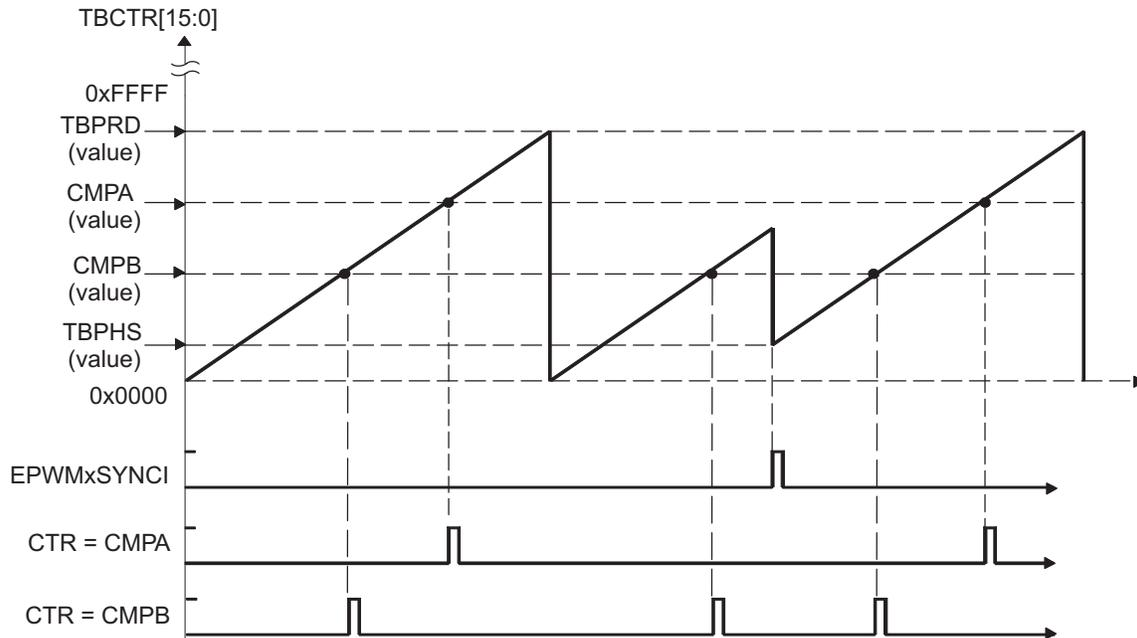
NOTE: An EPWMxSYNCl external synchronization event can cause a discontinuity in the TBCTR count sequence. This can lead to a compare event being skipped. This skipping is considered normal operation and must be taken into account.
