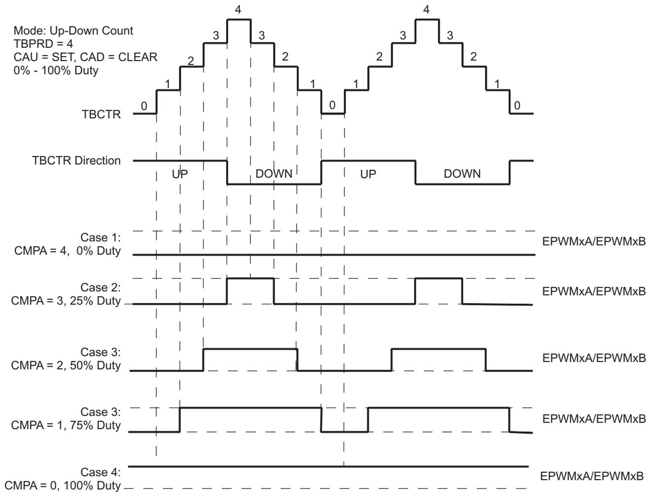
The PWM waveforms in [Figure 24](#) through [Figure 29](#) show some common action-qualifier configurations. The C-code samples in [Example 2](#) through [Example 7](#) shows how to configure an ePWM module for each case. Some conventions used in the figures and examples are as follows:
