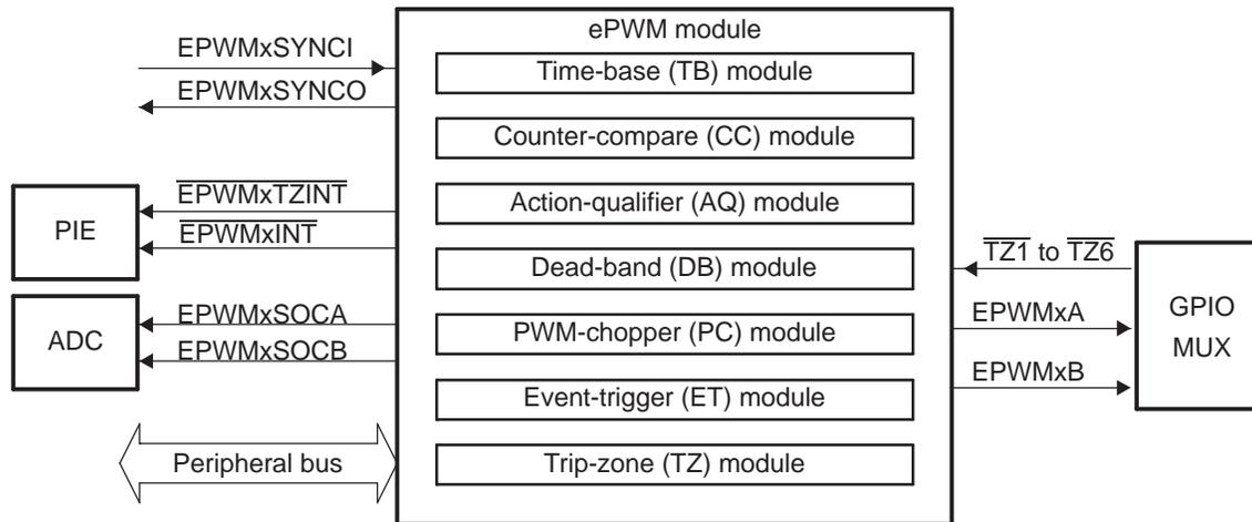
Figure 3 shows more internal details of a single ePWM module. The main signals used by the ePWM module are:
