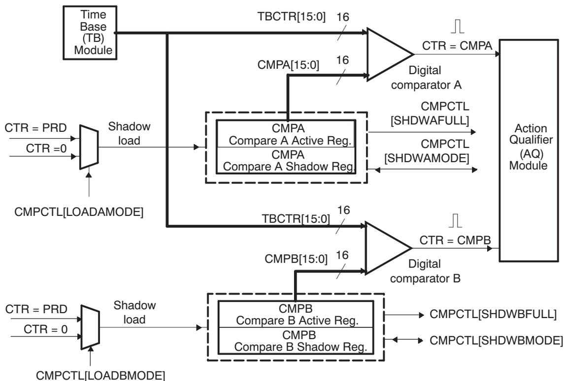
The key signals associated with the counter-compare submodule are described in [Table 6](#).
