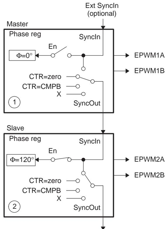
Figure 58 shows the associated timing waveforms for this configuration. Here, TBPRD = 600 for both master and slave. For the slave, TBPHS = 200 (i.e.,  $200/600 \times 360^\circ = 120^\circ$ ). Whenever the master generates a SyncIn pulse (CTR = PRD), the value of TBPHS = 200 is loaded into the slave TBCTR register so the slave time-base is always leading the master's time-base by 120°.
