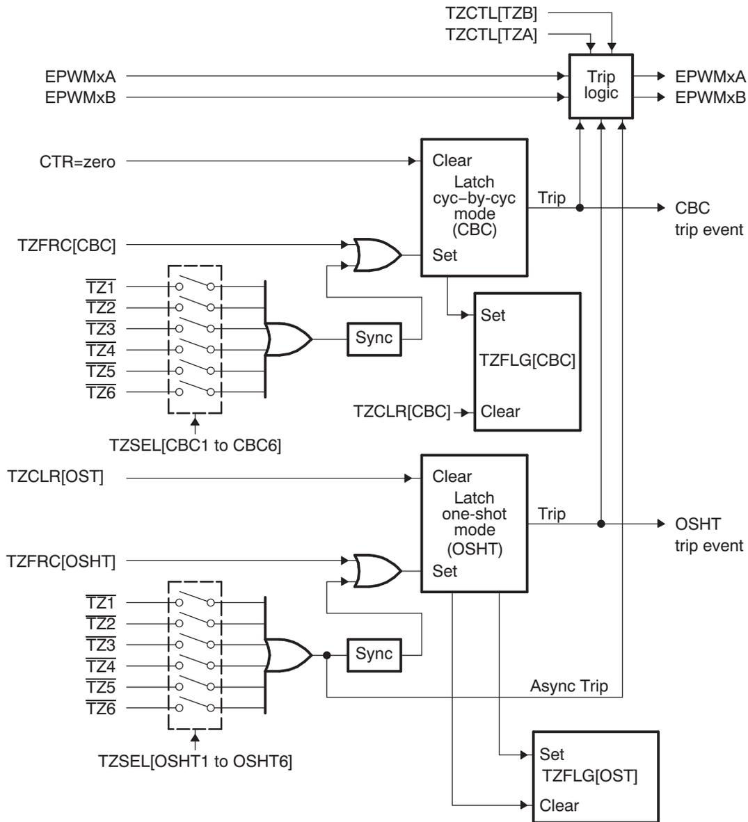
Figure 40. Trip-Zone Submodule Interrupt Logic
