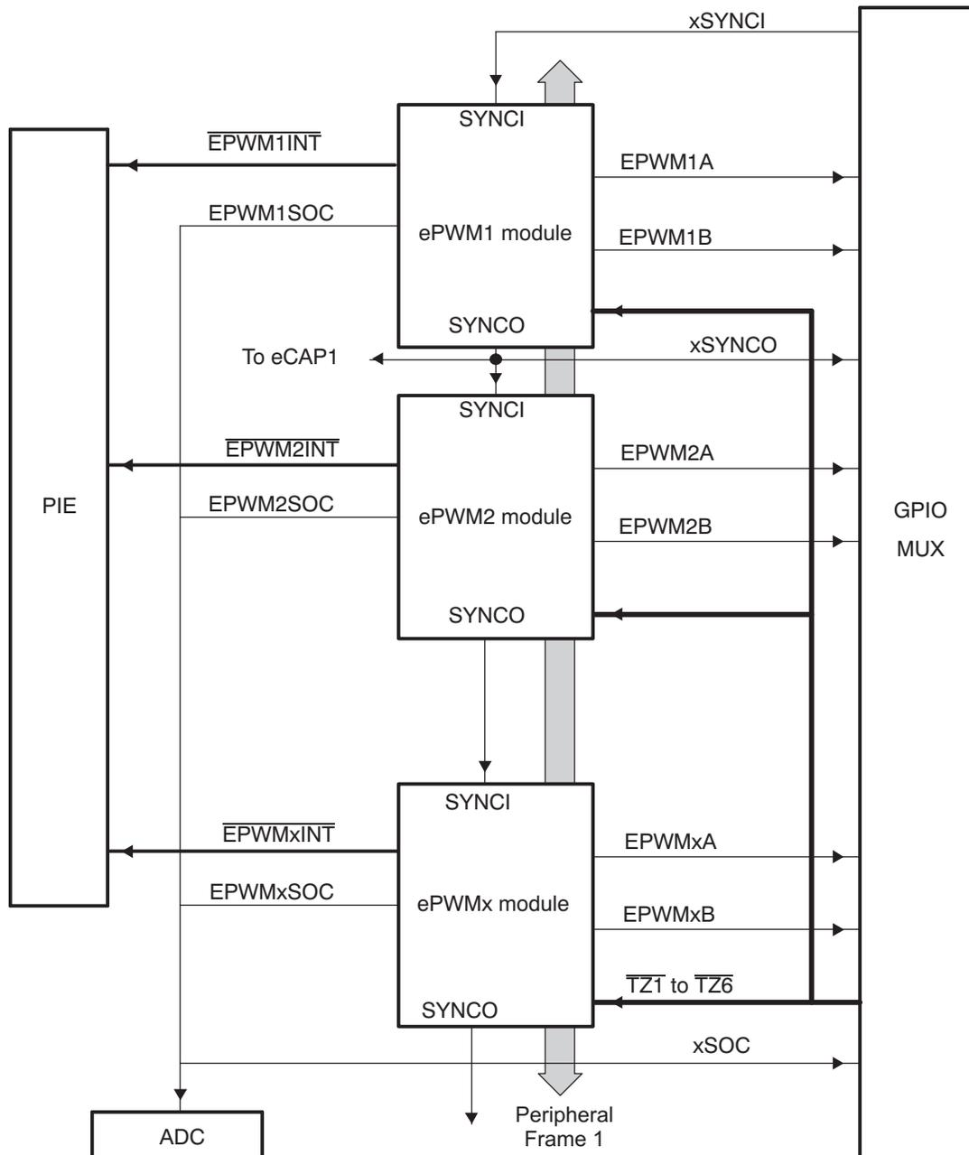
The order in which the ePWM modules are connected may differ from what is shown in Figure 1. See Section 2.2.3.2 for the synchronization scheme for a particular device. Each ePWM module consists of seven submodules and is connected within a system via the signals shown in Figure 2.
