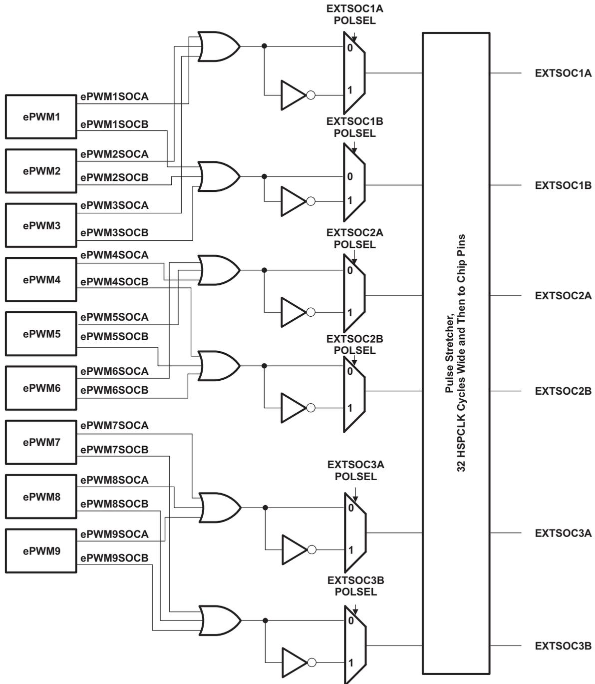
The event-trigger submodule monitors various event conditions (the left side inputs to event-trigger submodule shown in Figure 43) and can be configured to prescale these events before issuing an Interrupt request or an ADC start of conversion. The event-trigger prescaling logic can issue Interrupt requests and ADC start of conversion at:
