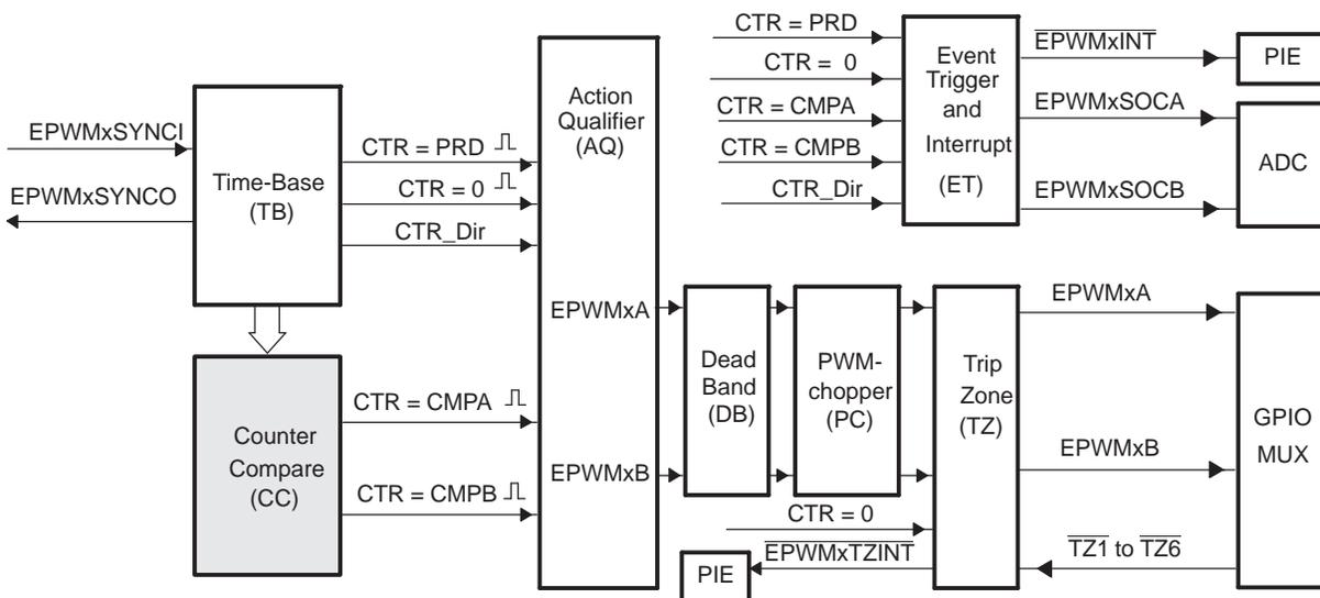
Figure 15 shows the basic structure of the counter-compare submodule.
