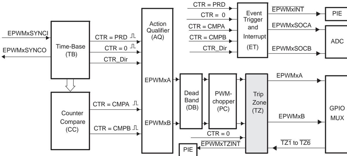
Each ePWM module is connected to six  $\overline{\text{TZn}}$  signals ( $\overline{\text{TZ1}}$  to  $\overline{\text{TZ6}}$ ) that are sourced from the GPIO MUX. These signals indicate external fault or trip conditions, and the ePWM outputs can be programmed to respond accordingly when faults occur.
