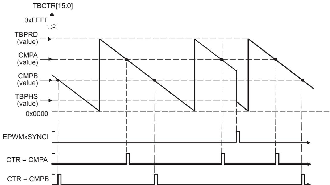
**Figure 18. Counter-Compare Events In Up-Down-Count Mode, TBCTL[PHSDIR = 0] Count Down On Synchronization Event**
