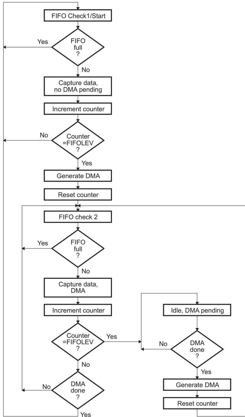
Figure 1-11. FIFO Operation During Card Write Diagram
