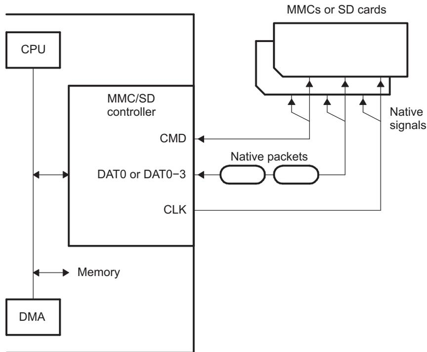
Figure 1-3. MMC Configuration and SD Configuration Diagram
