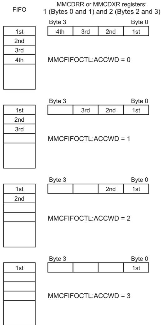
**Figure 1-9. Big-Endian Access to MMCDXR/MMCDRR1 and 2 From the CPU or the DMA**
