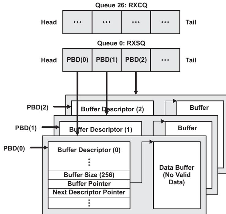
Figure 21. Receive USB Data Flow Example (Initialization)
