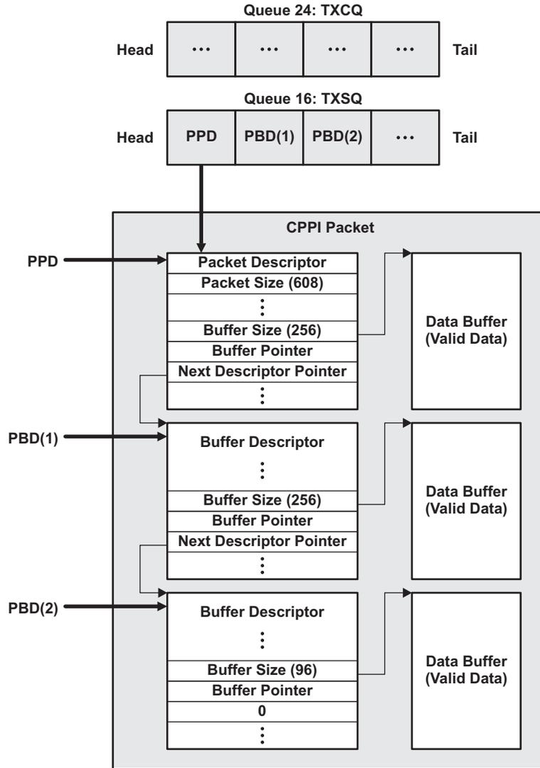
Figure 18. Transmit USB Data Flow Example (Initialization)
