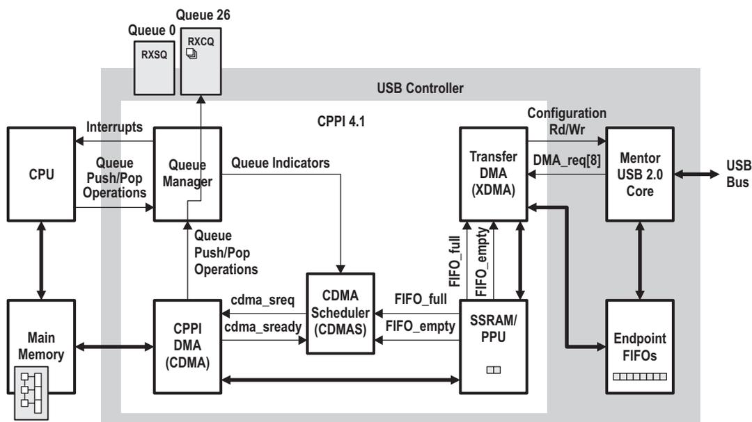
Step 4 (CDMA completes the packet transfer for Receive):
