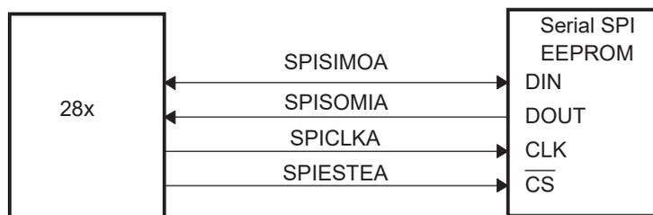
The SPI-A loader uses following pins:
