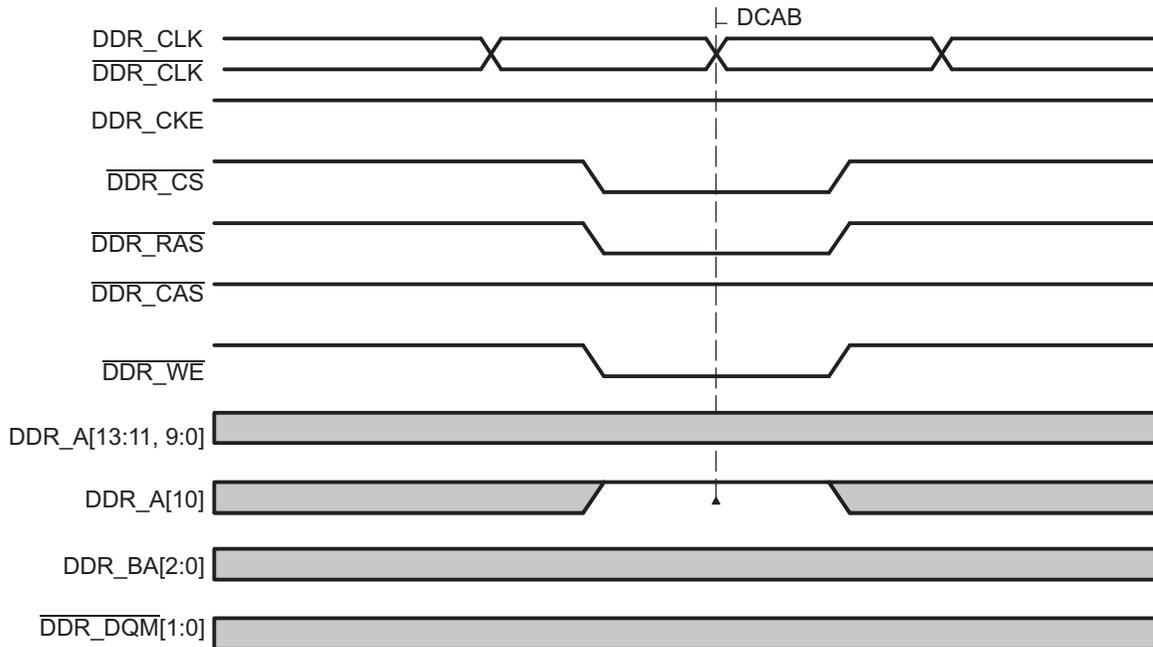
The DEAC command closes a single bank of memory specified by the bank select signals. [Figure 6](#) shows the timings diagram for a DEAC command.
