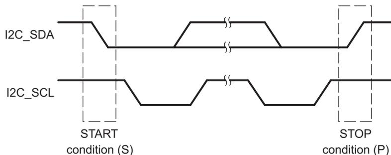
The I2C-bus is considered busy after a START condition and before a subsequent STOP condition. The bus busy (BB) bit of ICSTR is 1. The bus is considered free between a STOP condition and the next START condition. The BB is 0.
