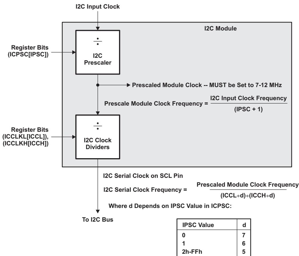
The prescaler (ICPSC [IPSC] ) must only be initialized while the I2C module is in the reset state (ICMDR [IRS] = 0). The prescaled frequency only takes effect when ICMDR [IRS] is changed to 1. Changing the ICPSC [IPSC] value while ICMDR [IRS] = 1 has no effect. Likewise, you must configure the I2C clock dividers (ICCLKH [ICCH] and ICCLKL [ICCL] while the I2C module is still in reset (ICMDR [IRS] = 0).
