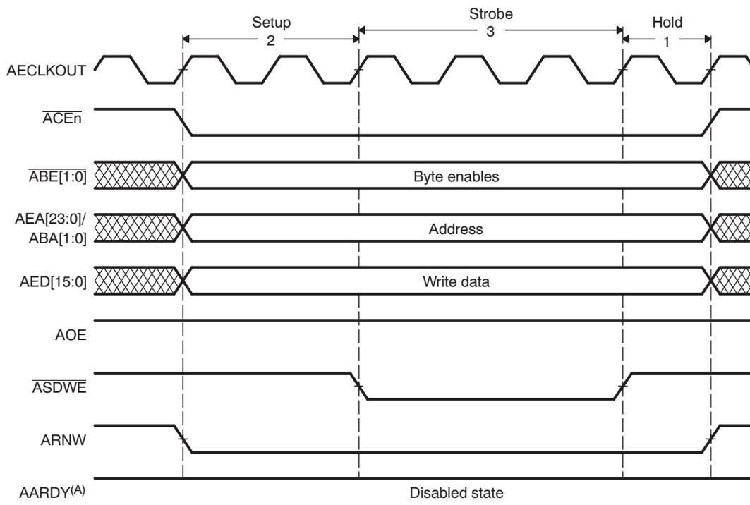
A The disabled state of the AARDY pin depends on the setting of the WP bit in the Asynchronous Wait Cycle Configuration Register.
