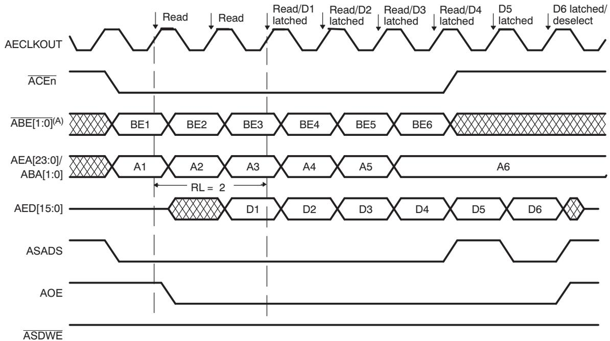
A ABE[1:0] is driven during reads only if the RD\_BE\_EN bit of the CEn Configuration register is set to 1. ABE[1:0] stays high during reads if RD\_BE\_EN = 0.
