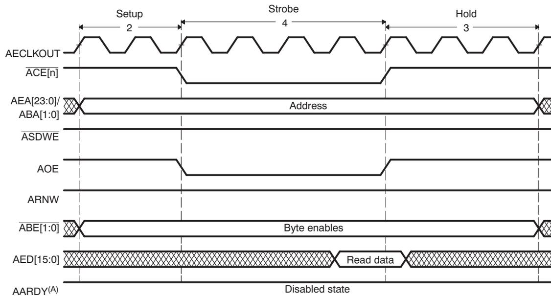
A The disabled state of the AARDY pin depends on the setting of the WP bit in the Asynchronous Wait Cycle Configuration Register.
