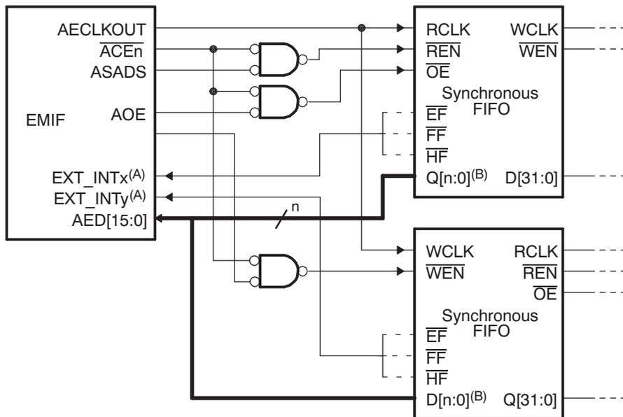
A GPIO pins on the device may be configured as external interrupt sources to the CPU. See the DSP General-Purpose Input/Output (GPIO) User's Guide for more details.
