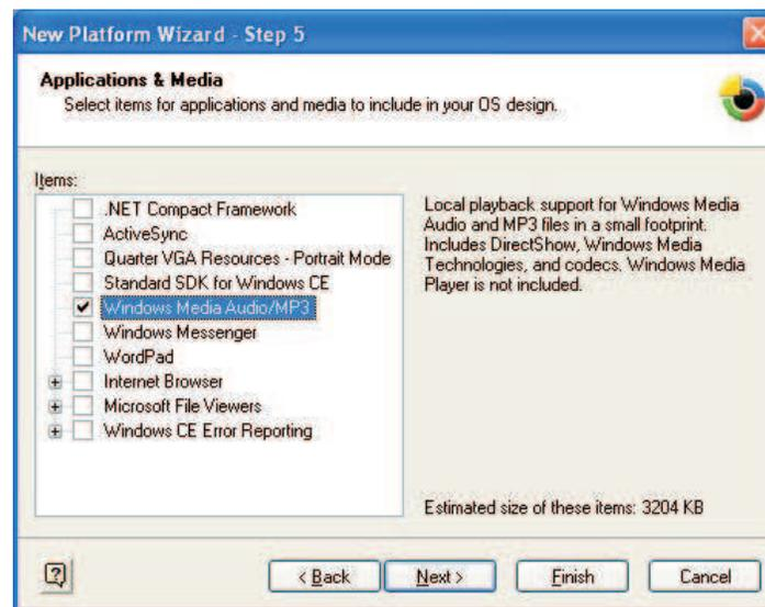
**Figure 5. Application and Media Components Selection**
