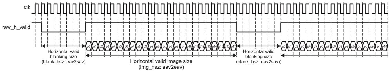
Figure 53. Channel *n* Horizontal Data Size Configuration Register (CH<sub>*n*</sub>\_HSIZE\_CFG)
