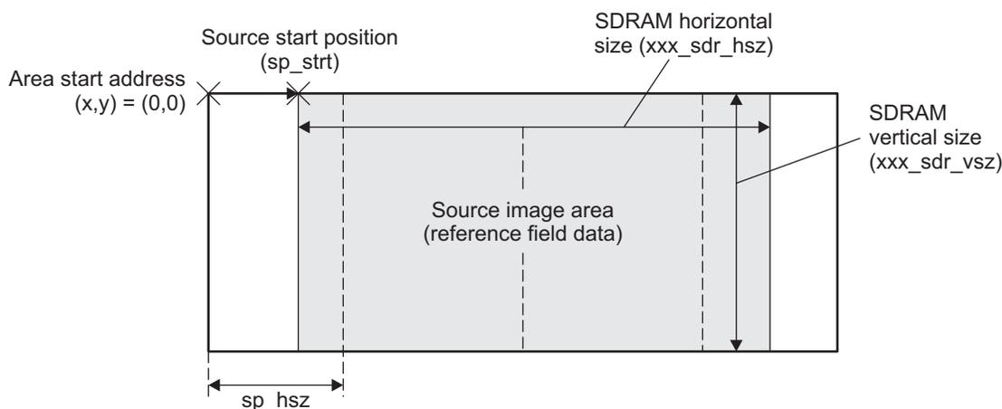
**Figure 38. Image of Storage Format on SDRAM in Raster Scanning Format**
