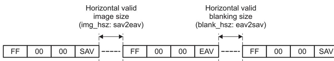
Figure 52. Image of Horizontal Distance in CCD/CMOS Mode
