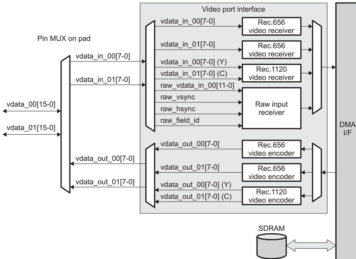
Figure 3. VPIF Architecture Block Diagram
