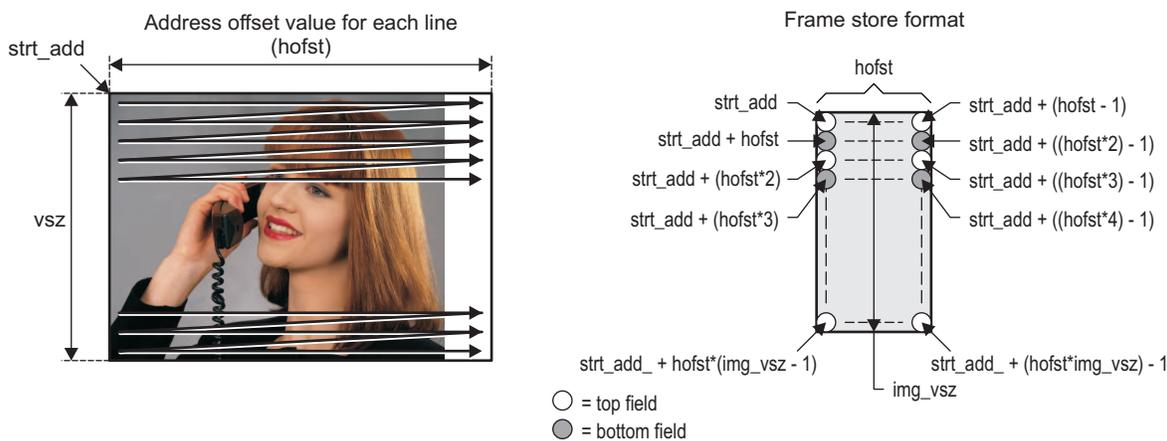
In [Figure 7](#), the upper illustration is a functional image of the SDRAM storage method. With register configuration (horizontal and vertical image size, and horizontal sub-picture size), a detailed address for each pixel is defined. The lower left illustration shows the raster scanning format addressing in field format and the lower right illustration shows the frame format.
