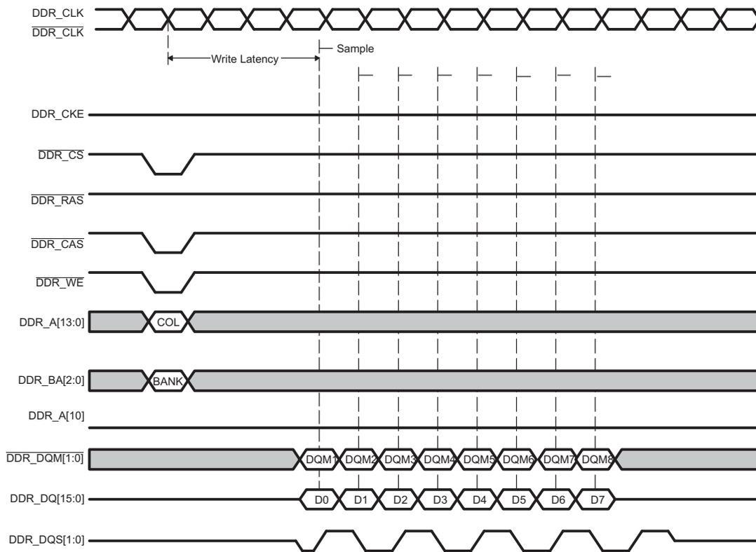
(1) This diagrams shows write latency for DDR2. For mDDR, write latency is always equal to 1 cycle.
