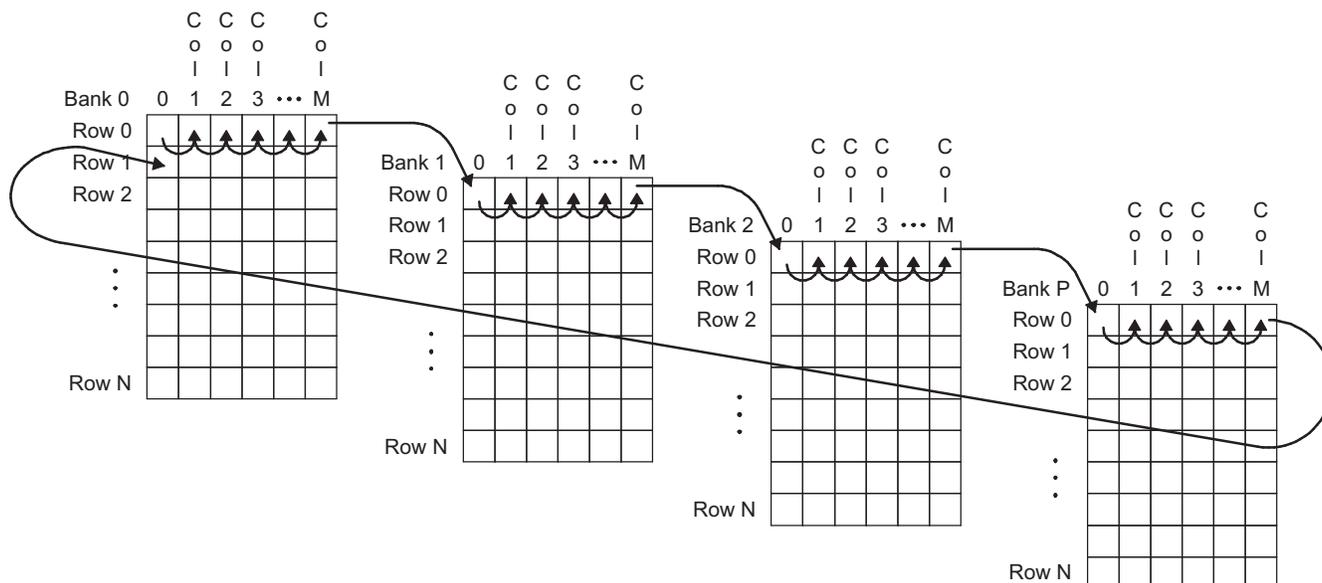
M is number of columns (as determined by PAGESIZE) minus 1, P is number of banks (as determined by IBANK) minus 1, and N is number of rows (as determined by both PAGESIZE and IBANK) minus 1.
