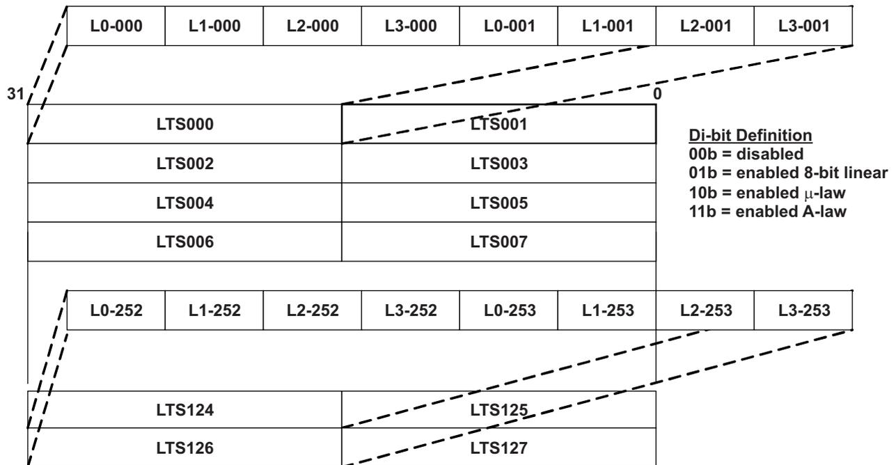
**Figure 6. 32 Mbps Channel Definition (8 Links with 2 Active Links)**
