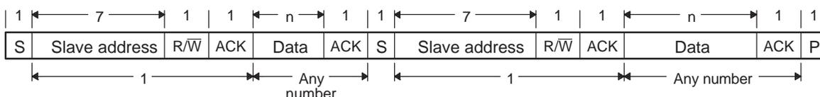
n = The number of data bits (from 1 to 8) specified by the bit count (BC) field of ICMDR.
