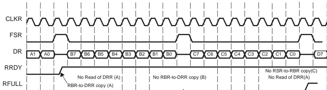
**Figure 21. Serial Port Receive Overrun Avoided**
