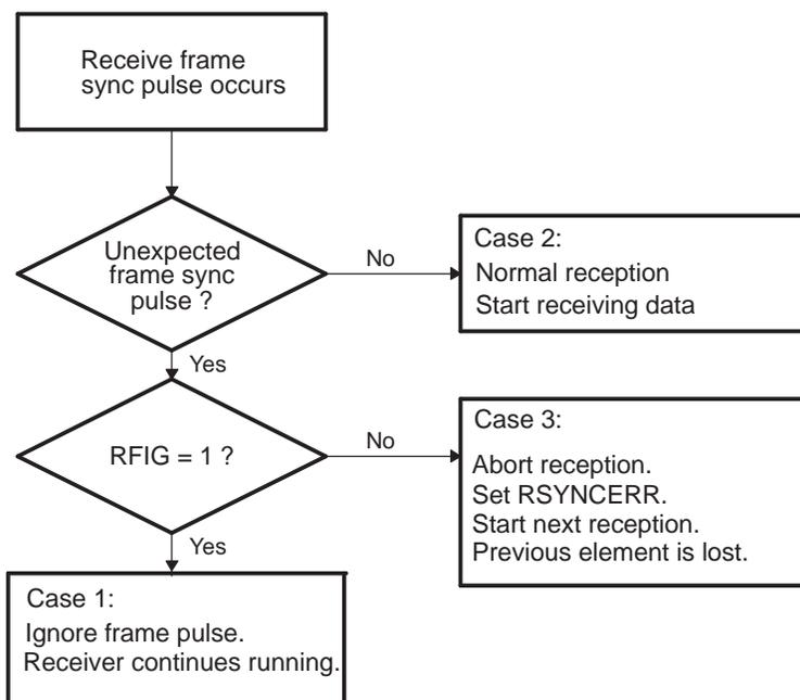
**Figure 23. Unexpected Receive Frame Synchronization Pulse**
