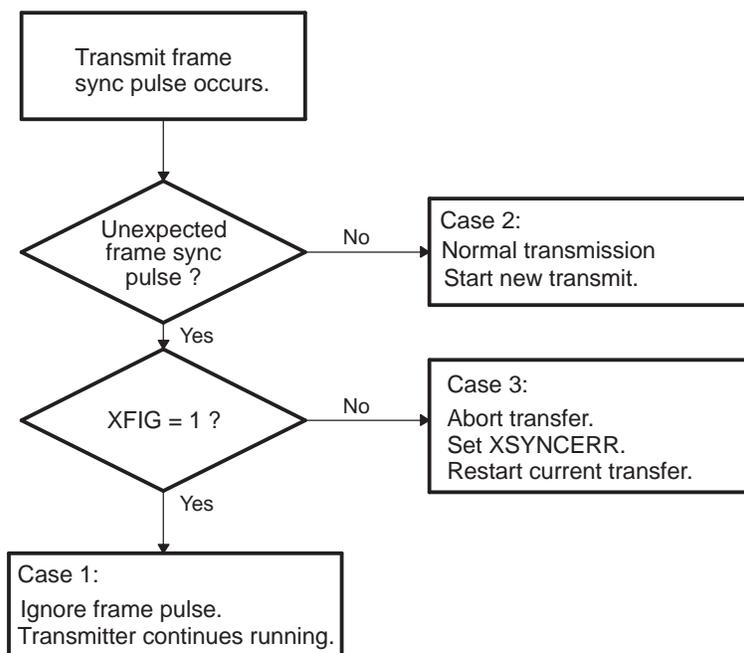
**Figure 28. Unexpected Transmit Frame Synchronization Pulse**
