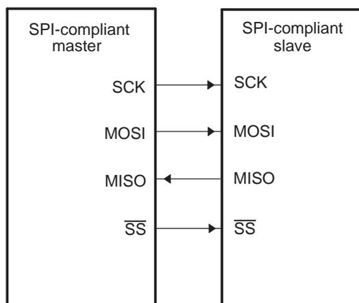
The master device controls the flow of communication by providing shift-clock and slave-enable signals. The slave-enable signal is an optional active-low signal that enables the serial data input and output of the slave device (the device not sending out the clock).
