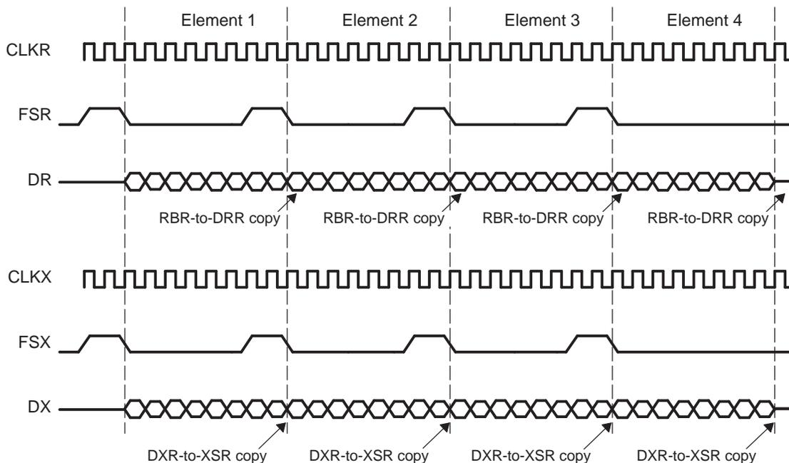
**Figure 19. Data Packing at Maximum Frame Frequency With (R/X)FIG = 1**
