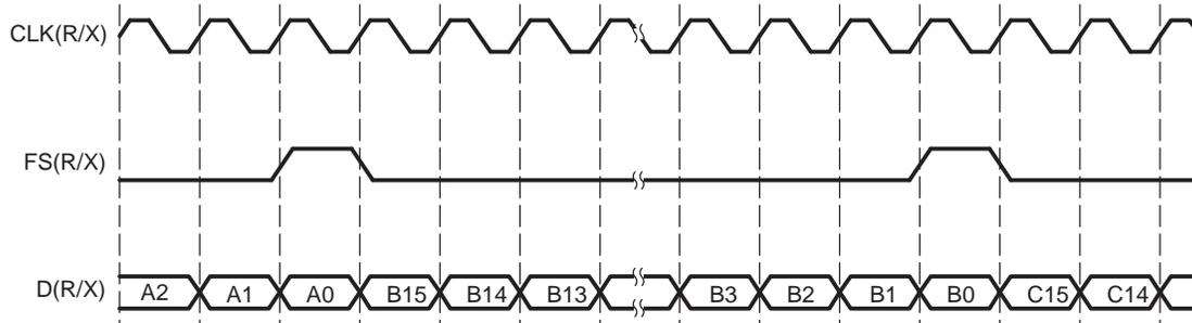
**Note:** For (R/X)DATDLY = 0, the first bit of data transmitted is asynchronous to CLKX, as shown in Figure 11.
