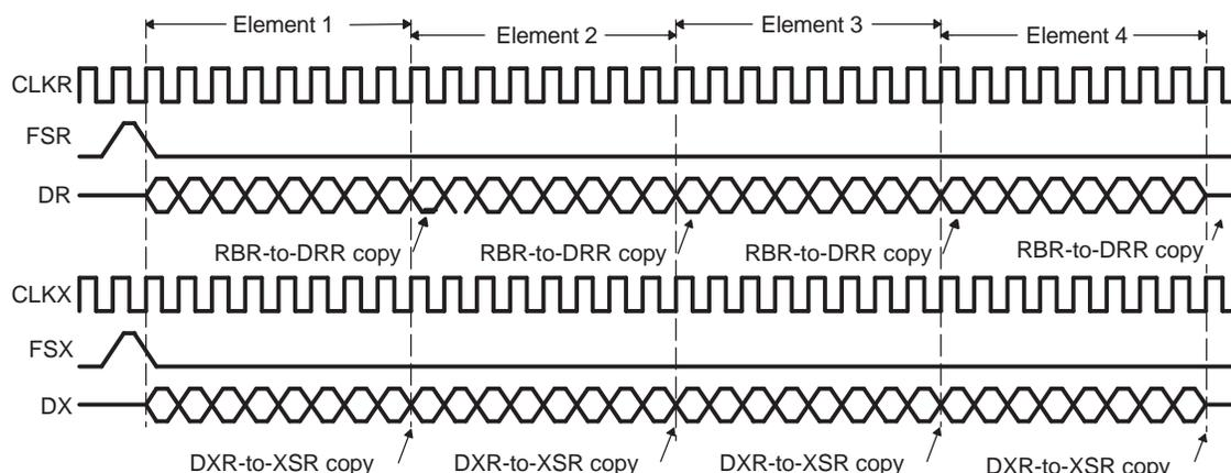
The example in [Figure 9](#) can also be viewed as a data stream of a single-phase frame of one 32-bit data element, as shown in [Figure 10](#). In this case:
