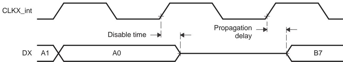
**Figure 4. Receive Data Clocking**
