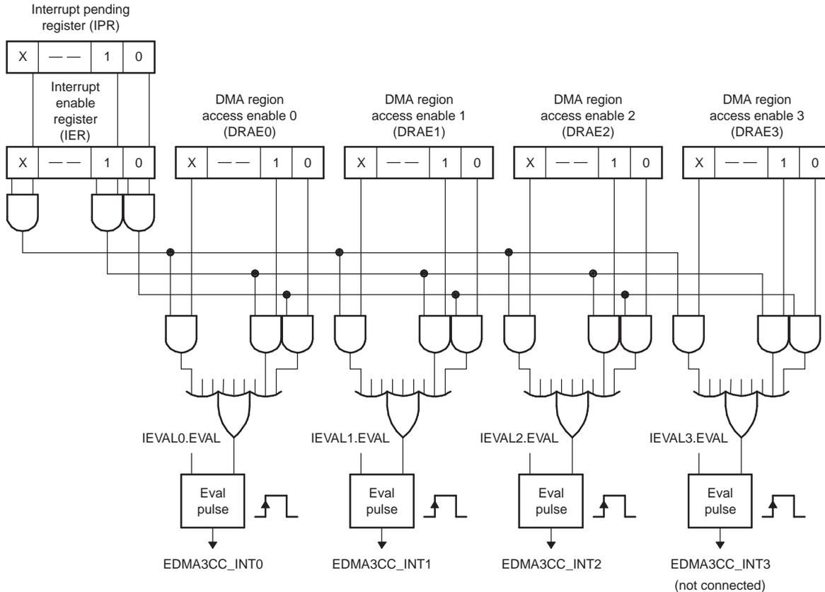
In order for the EDMA3CC to generate the transfer completion interrupts associated with each shadow region, the following conditions need to be true:
