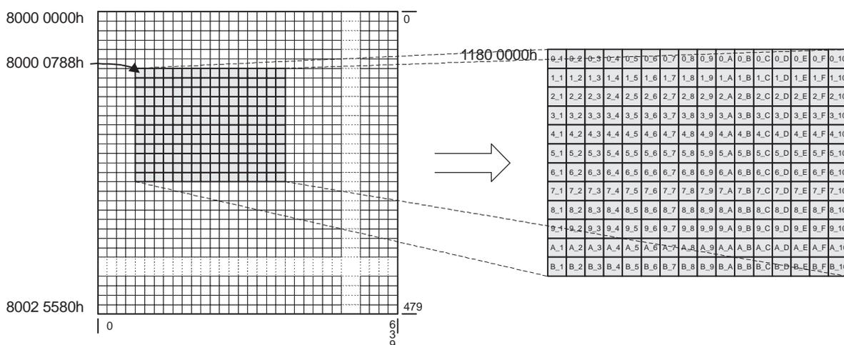
**Figure 3-4. Subframe Extraction Example PaRAM Configuration**
