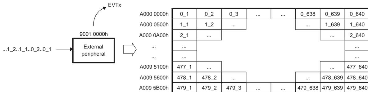
**Figure 3-10. Servicing Peripheral Burst Example PaRAM**
