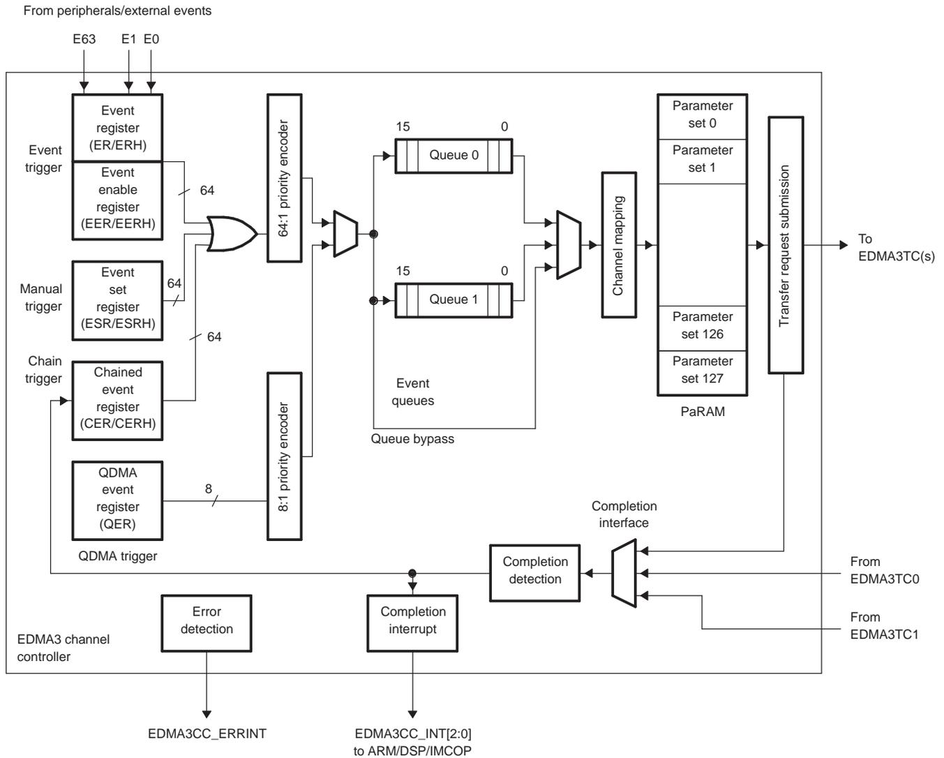
A trigger event is needed to initiate a transfer. For DMA channels, a trigger event may be due to an external event, manual write to the event set register, or chained event. QDMA channels are autotriggered when a write is performed to the user-programmed trigger word. All such trigger events are logged into appropriate registers upon recognition. Refer to DMA channel registers (Section 4.3.5) and QDMA registers (Section 4.3.7).
