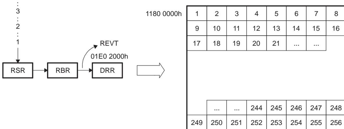
**Figure 3-8. Servicing Incoming ASP Data Example PaRAM**
