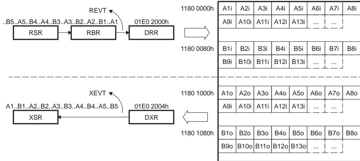
Figure 3-12. Servicing Continuous ASP Data Example PaRAM
