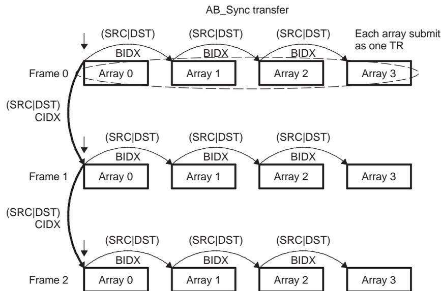
**NOTE:** ABC-synchronized transfers are not directly supported. But can be logically achieved by chaining between multiple AB-synchronized transfers.
