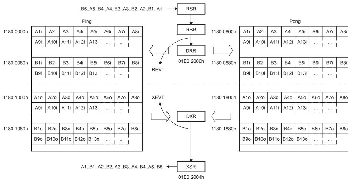
**Figure 3-15. Ping-Pong Buffering for ASP Example PaRAM**
