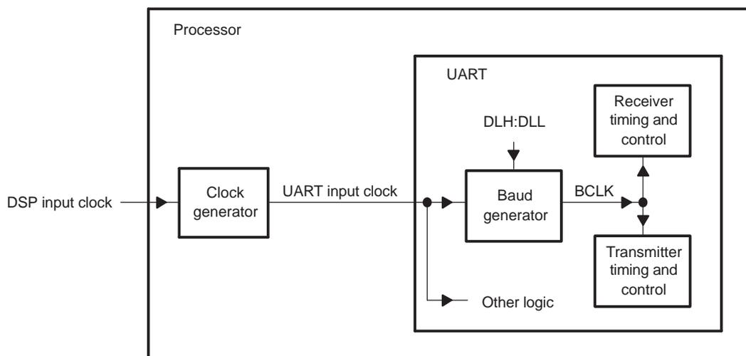
**Figure 3. Relationships Between Data Bit, BCLK, and UART Input Clock**
