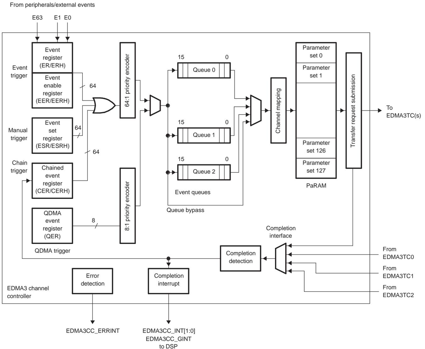
The EDMA3CC includes two channel types: DMA channels (64 channels) and QDMA channels (8 channels).
