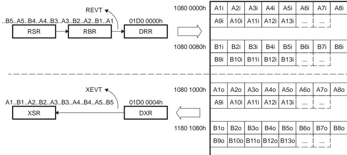
**Figure 3-12. Servicing Continuous McBSP Data Example PaRAM**
