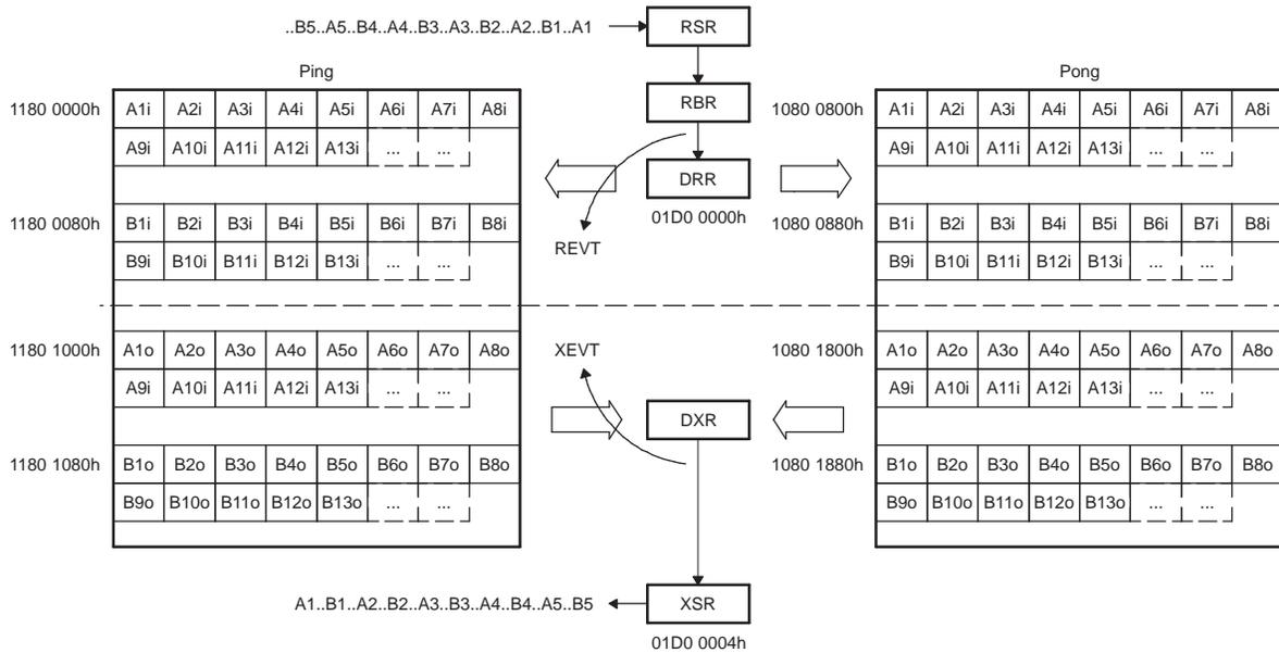
Figure 3-15. Ping-Pong Buffering for McBSP Example PaRAM
