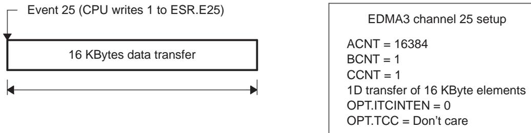
**Figure 3-20. Smaller Packet Data Transfers Example**
