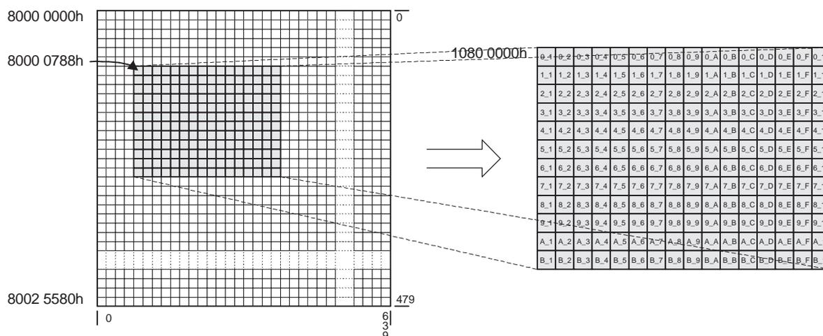
**Figure 3-4. Subframe Extraction Example PaRAM Configuration**
