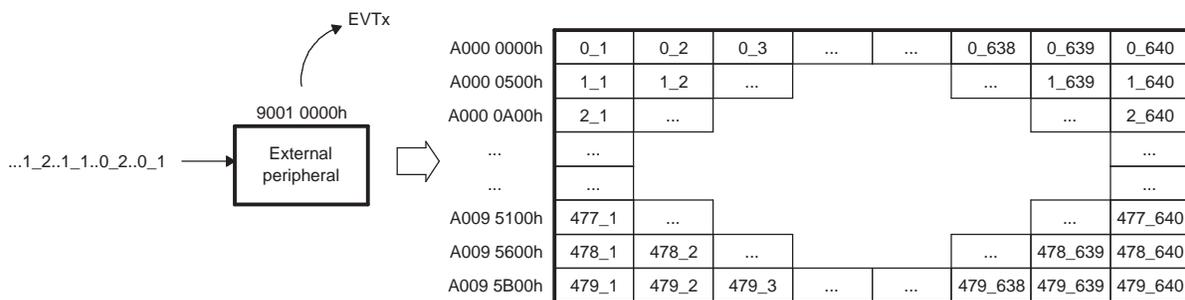
**Figure 3-10. Servicing Peripheral Burst Example PaRAM**
