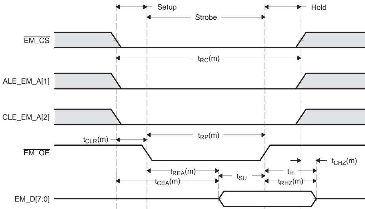
To determine the required EMIF configuration to interface to the NAND Flash for a write operation, [Table 27](#) lists the NAND AC timing parameters for a command latch, address latch, and data input latch that must be considered.
