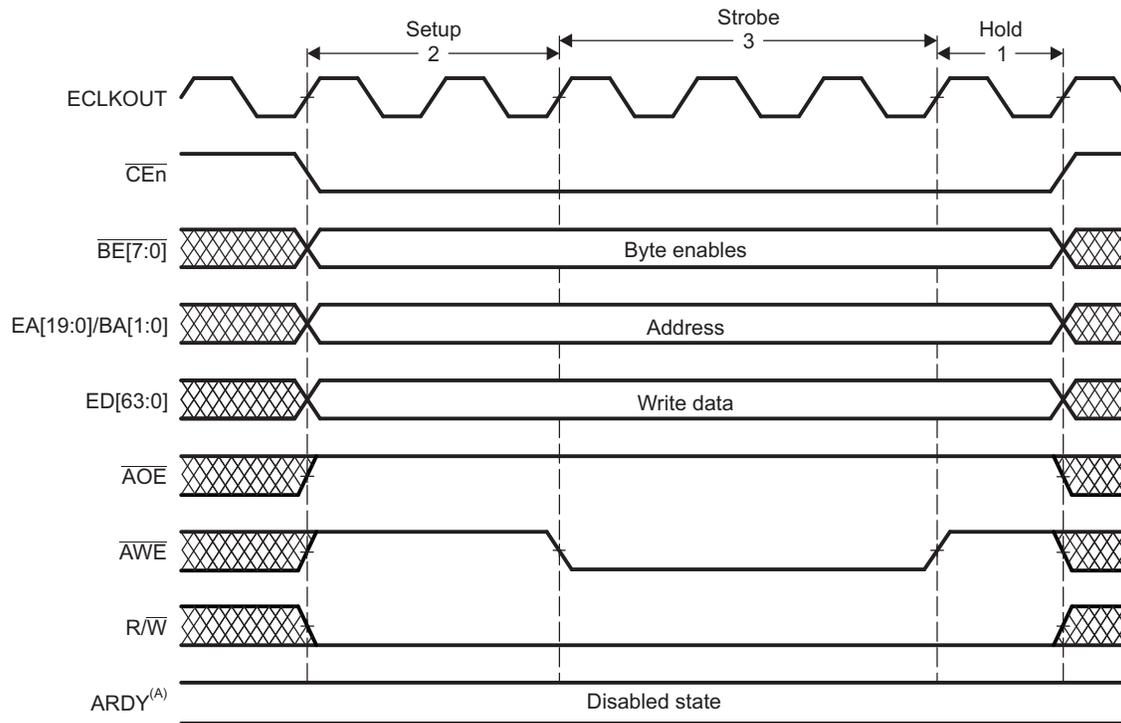
B The disabled state of the ARDY pin depends on the setting of the AP bit in the Asynchronous Wait Cycle Configuration Register.
