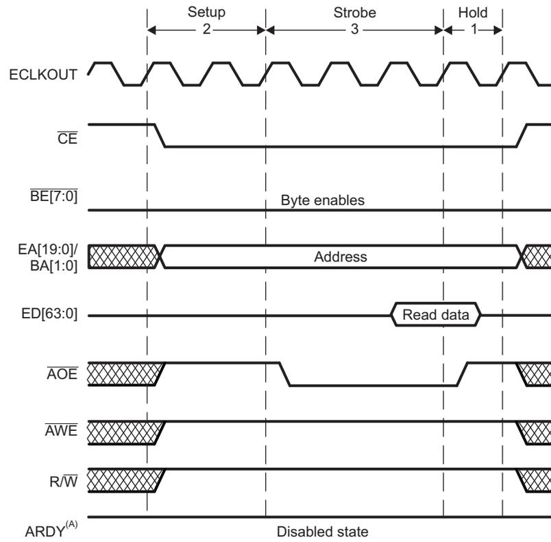
A The disabled state of the ARDY pin depends on the setting of the AP bit in the Asynchronous Wait Cycle Configuration Register.
