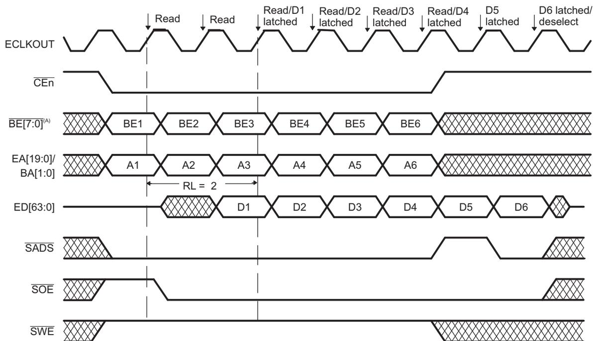
A  $\overline{BE}[7:0]$  is driven during reads only if the RD\_BE\_EN bit of the  $CE_n$  Configuration register is set to 1.  $\overline{BE}[7:0]$  stays high during reads if RD\_BE\_EN = 0.
