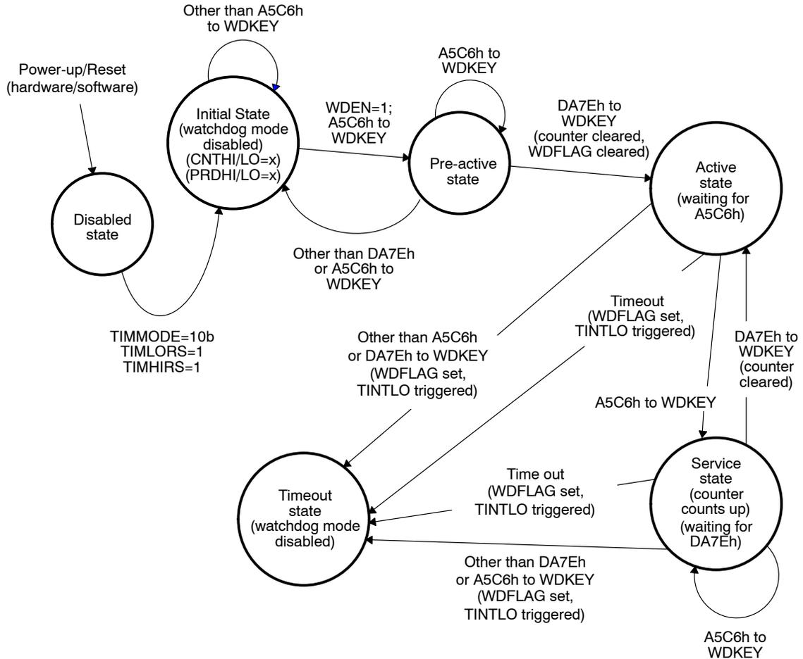
Once the watchdog timer is activated, it can be disabled only by a watchdog timeout event or by a hardware reset. A special key sequence is required to prevent the watchdog timer from being accidentally serviced while the software is trapped in a dead loop or by some other software failure.
