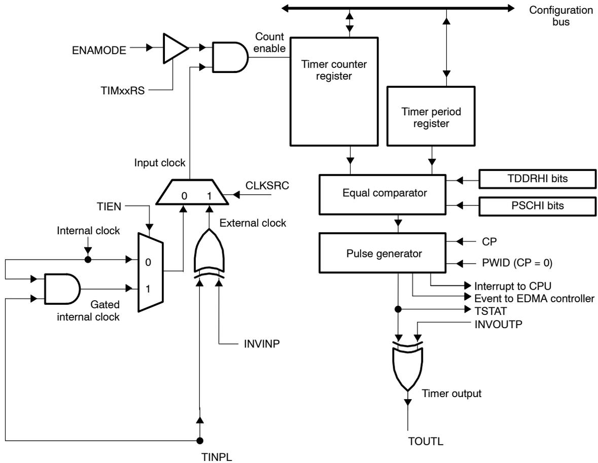
The timer can be driven by an external clock at the timer input pin (TINPL) or by the divide-down clock rate of the internal clock. The internal clock is generated by the PLL1 controller and is a divided-down version of the CPU clock (see the device-specific data manual for more information).
