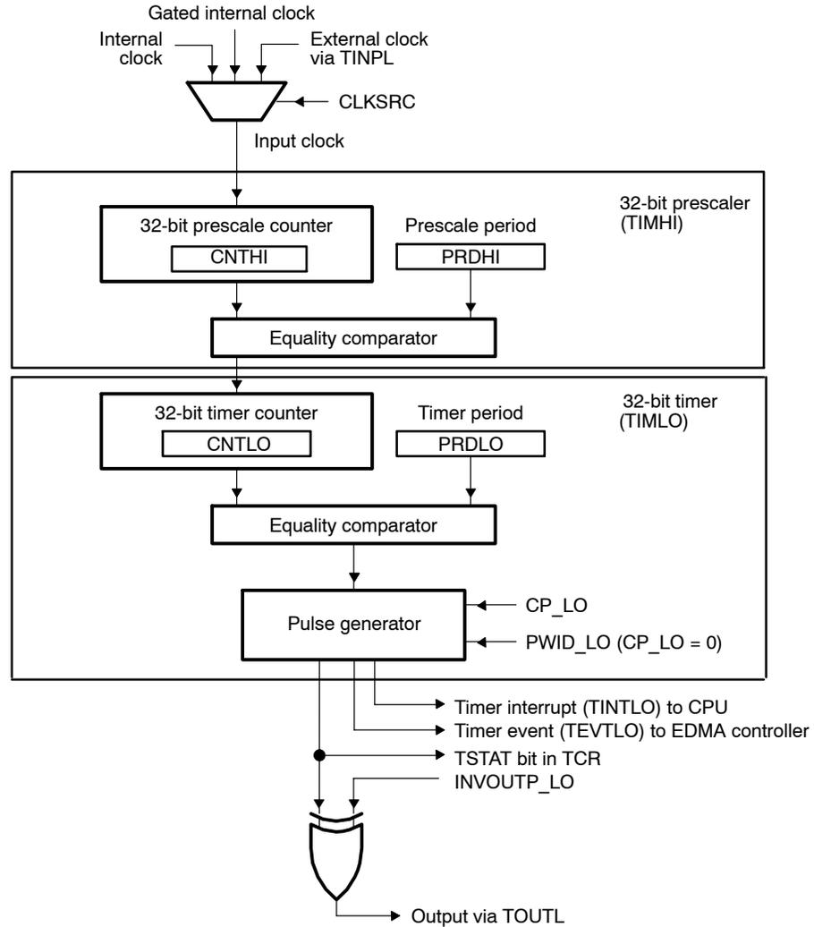
Figure 5. Dual 32-Bit Timers Chained Mode Example
