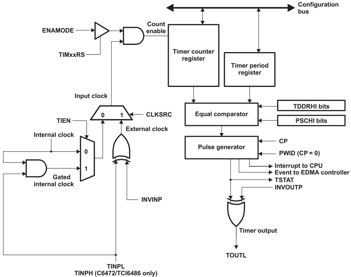
The timer can be driven by an external clock at the timer input pin (TINPL) or by the divide-down clock rate of the internal clock, as shown in Figure 2. For C6472/TCI6486 devices, TINPH can be used to drive the higher 32-bit timer, TIMHI, in unchained mode. The internal clock is generated by the PLL1 controller and is a divided-down version of the CPU clock. For more information, see the device-specific data manual.
