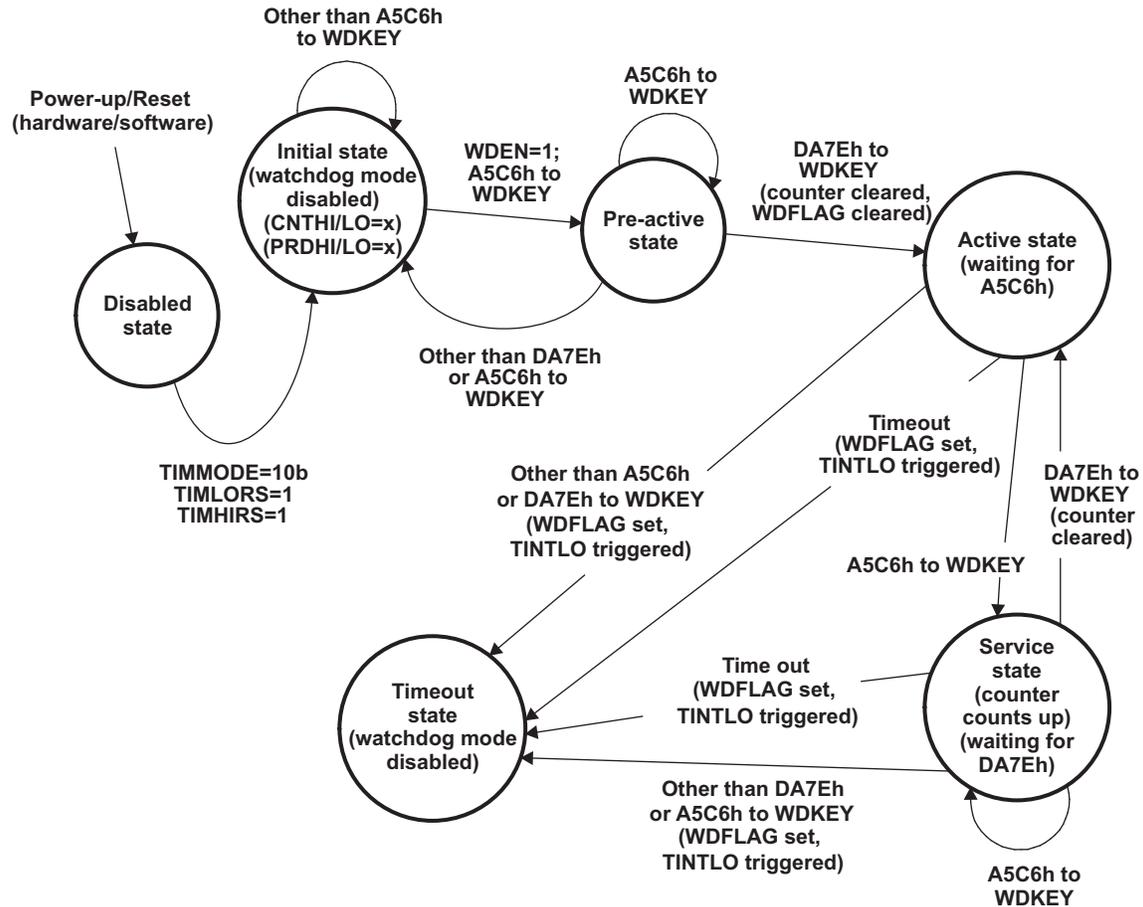
Once the watchdog timer is activated, it can be disabled only by a watchdog timeout event or by a hardware reset. A special key sequence is required to prevent the watchdog timer from being accidentally serviced while the software is trapped in a dead loop or by some other software failure.
