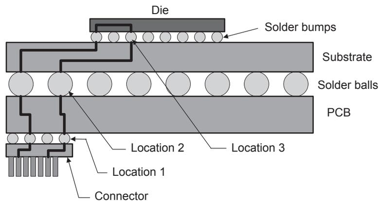
Figure 27. Schematic of TDR Waveforms for a Flip Chip BGA Package.
