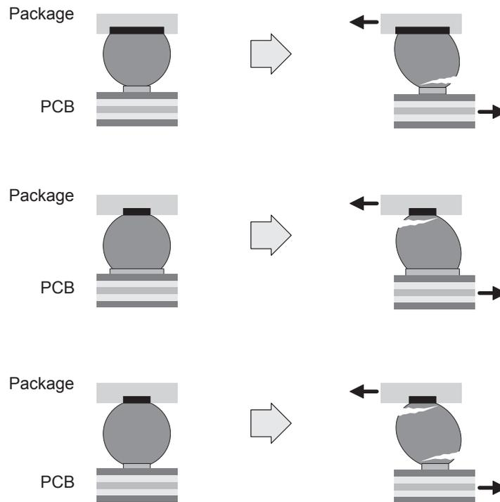
In fact, if the design of the PCB pad diameters are even slightly smaller than the package side BGA pad diameter, the joint stress on the PCB side is emphasized rather than on the typically weaker package BGA side.
