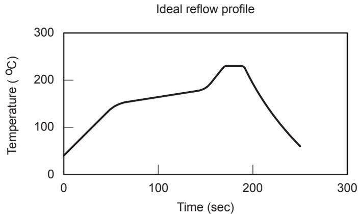
**Note:** This is an ideal profile, and actual conditions obtained in any specific reflow oven will vary. This profile is based on convection or RF plus forced convection heating.
