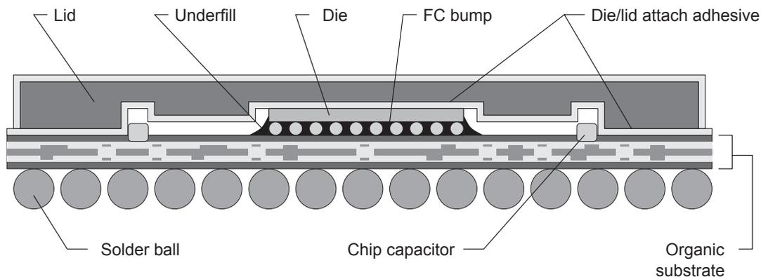
Flip chip components are predominantly semiconductor devices; however, components such as passive filters, detector arrays, and MEMS devices are now used in flip chip form.
