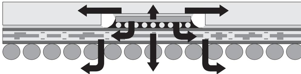
For moderate power dissipation (less than 6 watts), using passive heat sinks and heat spreaders attached with thermally conductive double-sided tapes or retainers, can offer quick thermal solutions in these packages.
