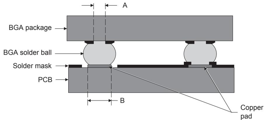
Figure 9 illustrates why the layout and dimensions of the package pads and the board lands are critical. Matching the diameters of the PCB pad to the package side BGA pad helps form a symmetrical interconnect, and prevents one end of the interconnect from exhibiting a higher stress condition than the other.
