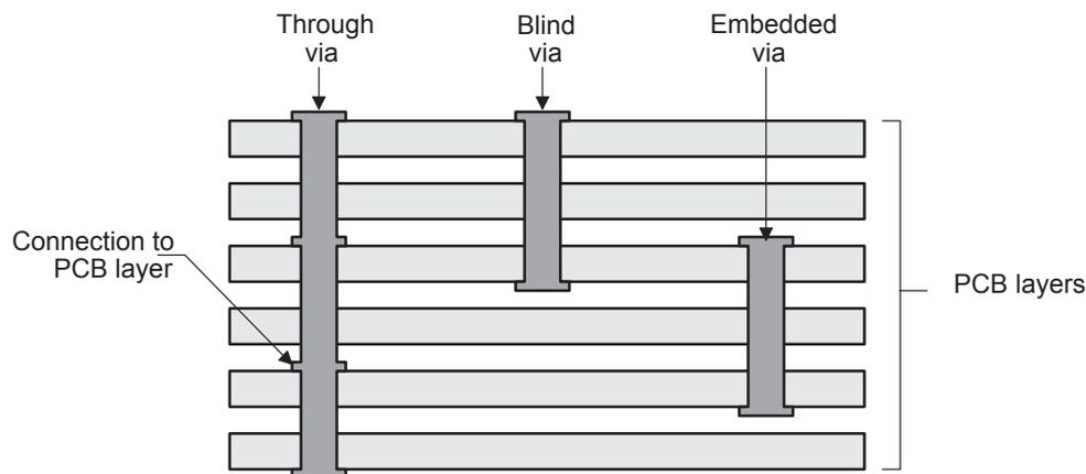
Although blind vias can be more expensive than through vias, overall costs can be reduced because signal traces can be routed under a blind via, which requires fewer PCB layers.
