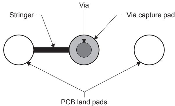
Figure 13 shows the space available between surface land pads for a 0.40 mm (15.75 mil) BGA pad.
