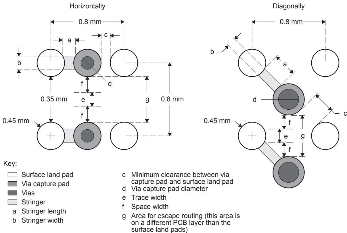
Consider the following factors when deciding to place the via capture pads diagonally or inline with the surface land pads:
