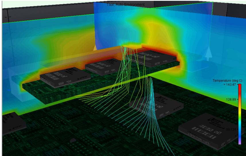
**Note:** Planes show temperature profile. Streamlines show airflow. Graphic by Flomerics, Ltd.™
