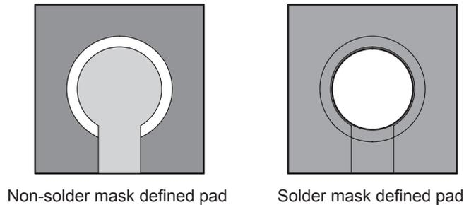
Figure 7. NSMD and SMD Pads – Cross-Sectional View
