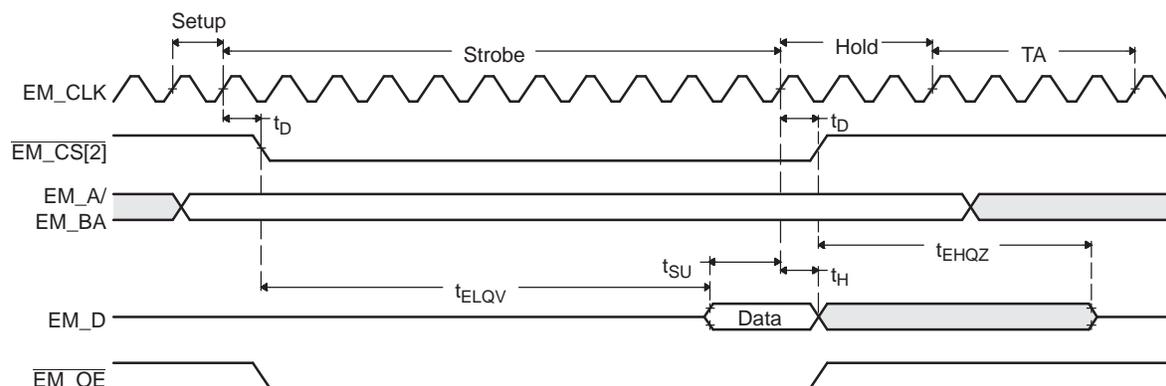
**Figure 4-7. LH28F800BJE-PTTL90 to EMIF Write Timing Waveforms**
