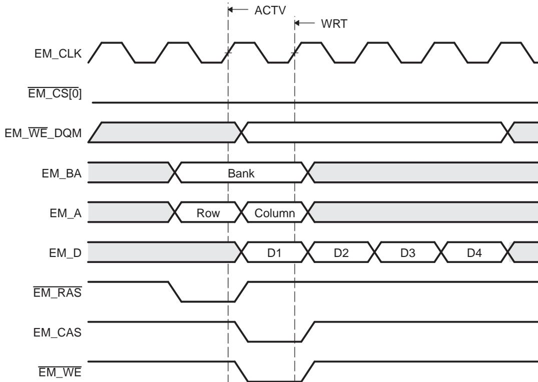
The EMIF will truncate a series of bursting data if the remaining addresses of the burst are not part of the write request. The EMIF can truncate the burst in three ways:
