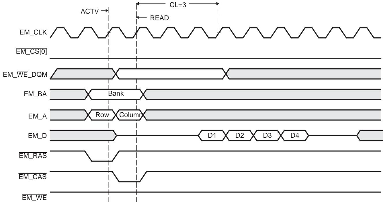
The EMIF will truncate a series of bursting data if the remaining addresses of the burst are not required to complete the request. The EMIF can truncate the burst in three ways:
