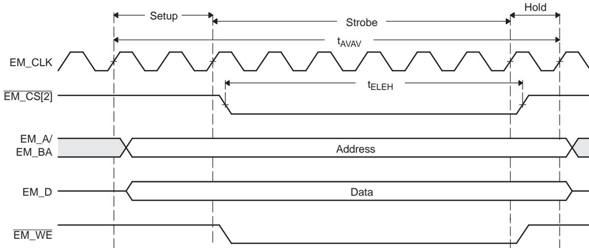
The R\_STROBE field should be set to meet the following equation:
