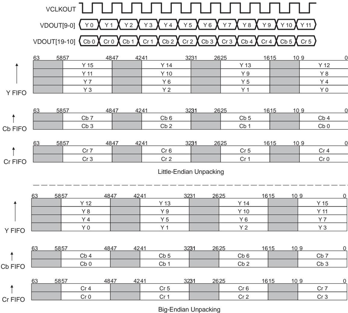
In 10-bit Y/C dense-pack mode, three samples are unpacked from each word in the FIFO as seen in Figure 4-18.
