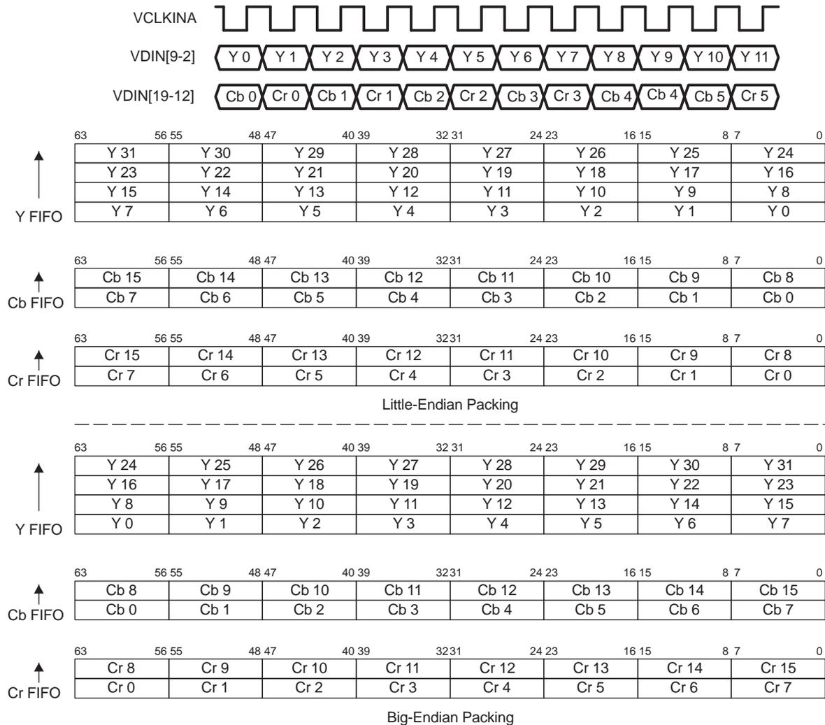
The 10-bit Y/C mode uses three FIFOs for color separation. Two samples are packed into each word with zero or sign extension as shown in [Figure 3-6](#).
