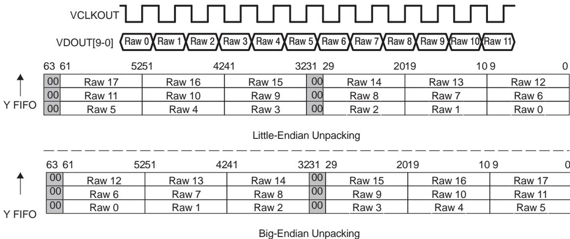
The 16-bit raw data mode stores all data into a single FIFO. Two samples are packed into each word as shown in [Figure 3-20](#).
