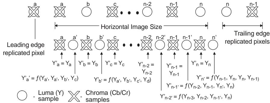
Examples of luma edge replication for 2x interspersed to co-sited output are shown in Figure 4-23 and Figure 4-24, respectively.
