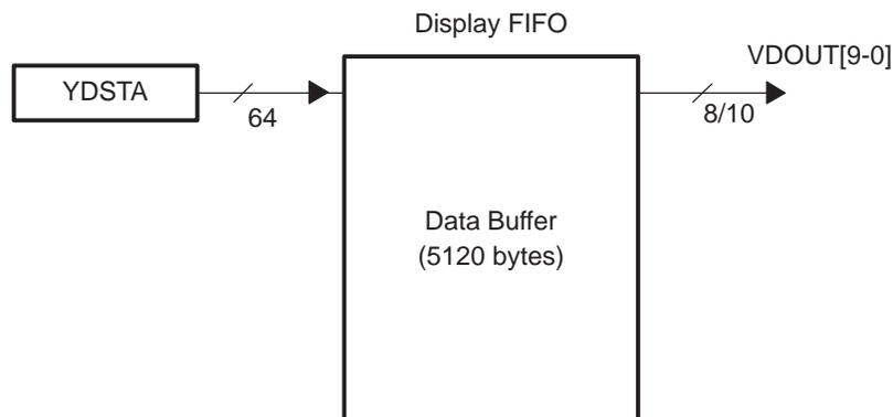
For locked raw video, the FIFO is split into channel A and B. The channels are locked together and use the same clock and control signals. Each channel uses a single buffer and write register (YDSTx) as shown in Figure 1-8.
