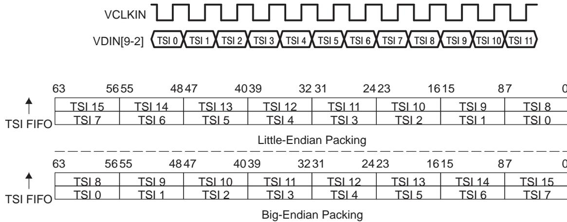
The data capture circuitry signals to the synchronizing circuit when to take a timestamp of the hardware counters. The FIFO write controller keeps track of number of bytes received in a packet. It multiplexes the timestamp data and the packet data onto the FIFO write data bus. The timestamp and packet error information are inserted after each packet in the FIFO and must use the correct endian byte ordering. The format for the timestamp is shown in [Figure 3-26](#) and [Figure 3-27](#).
