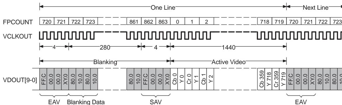
SAV and EAV codes are identified by a 3-byte preamble of FFh, 00h, and 00h. This combination must be avoided in the video data output by the video port to prevent accidental generation of an invalid sync code. The video display module provides programmable maximum and minimum value clipping on the video data to prevent this possibility.
