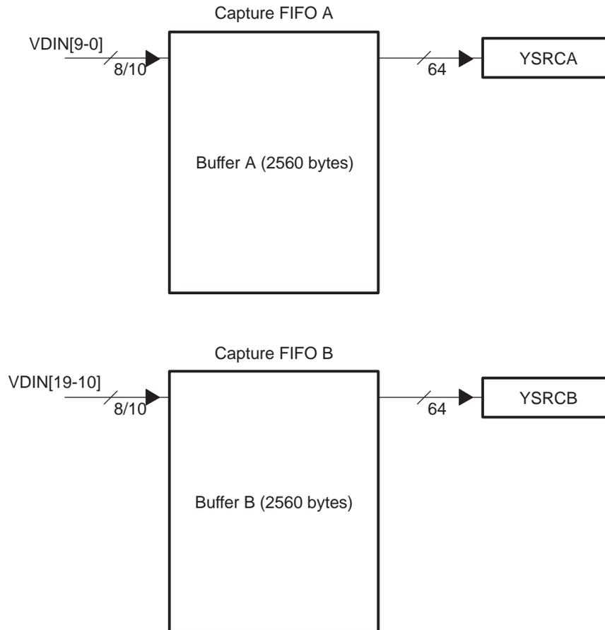
For Y/C video capture, the FIFO is configured as a single channel split into separate Y, Cb, and Cr buffers with separate write pointers and read registers (YSRCA, CBSRCA, and CRSRCA). Figure 1-4 shows how Y data is received on the VDIN[9-0] half of the bus and Cb/Cr data is received on the VDIN[19-10] half of the bus and de-multiplexed into the Cb and Cr buffers.
