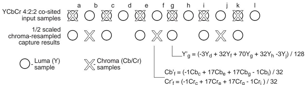
Note that because input scaling is limited to 1/2, true CIF horizontal resolution is not achieved if the full BT.656 horizontal line (720 pixels) is captured. A CIF size line can be captured by selecting a 704 pixel-sized window within the BT.656 line. This window size and location on the line are programmed using the VCXSTART $n$  and VCXSTOP $n$  bits.
