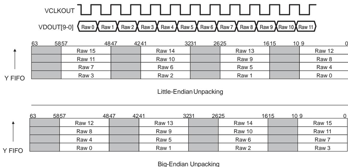
In 10-bit raw dense-pack mode, three samples are unpacked from each word in the FIFO as seen in Figure 4-27.
