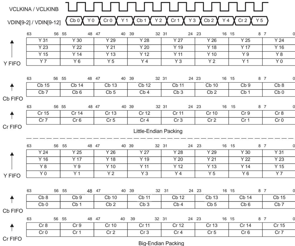
The 10-bit BT.656 mode uses three FIFOs for color separation. Two samples are packed into each word with zero or sign extension as shown in [Figure 3-3](#).
