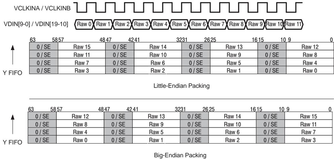
The 10-bit dense raw data mode stores all data into a single FIFO. Three samples are packed into each word with zero extension as shown in Figure 3-19.
