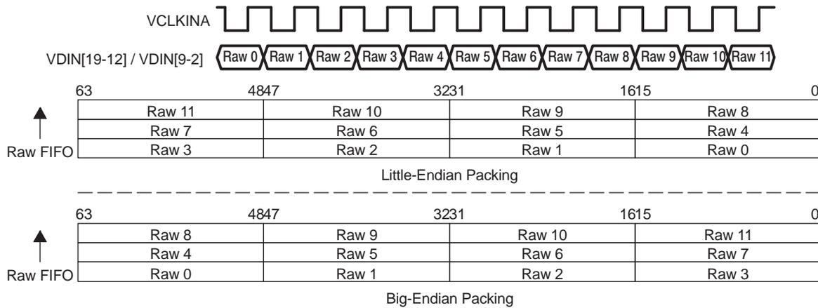
The 20-bit raw data mode stores all data into a single FIFO. One sample is placed right justified in each word and zero or sign extended as shown in [Figure 3-21](#).
