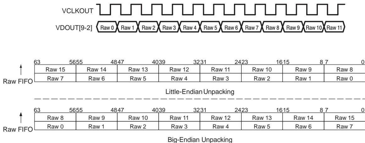
For 10-bit operation, two samples are unpacked from each FIFO word. This is shown in Figure 4-26.
