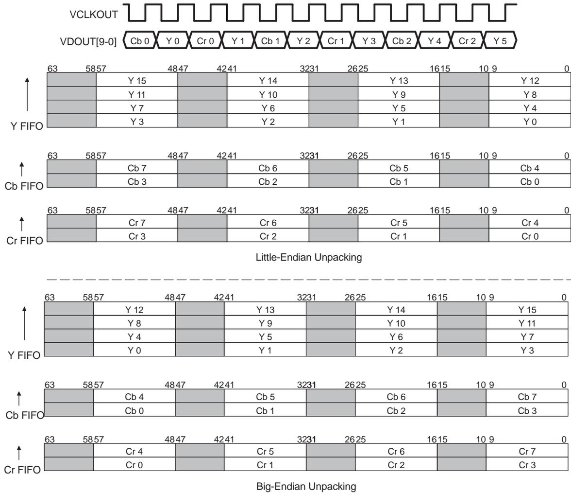
In 10-bit BT.656 dense-pack mode, three samples are unpacked from each word in the FIFO as seen in Figure 4-14.
