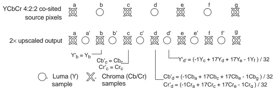
Figure 4-21. 2x Interspersed Scaling
