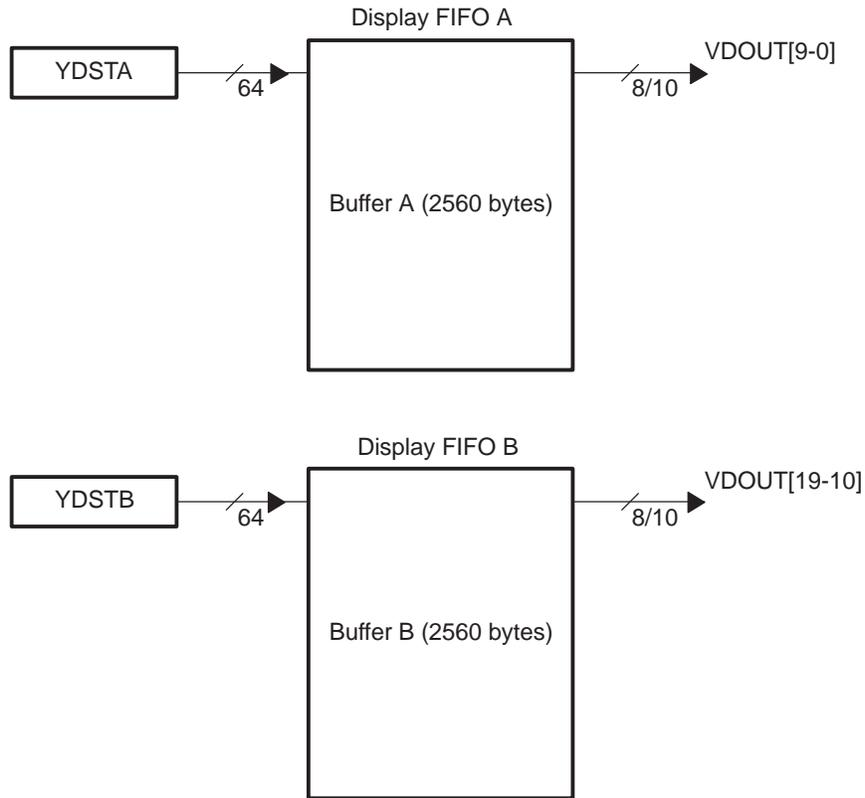
**Figure 1-9. 16/20-Bit Raw Video Display FIFO Configuration**
