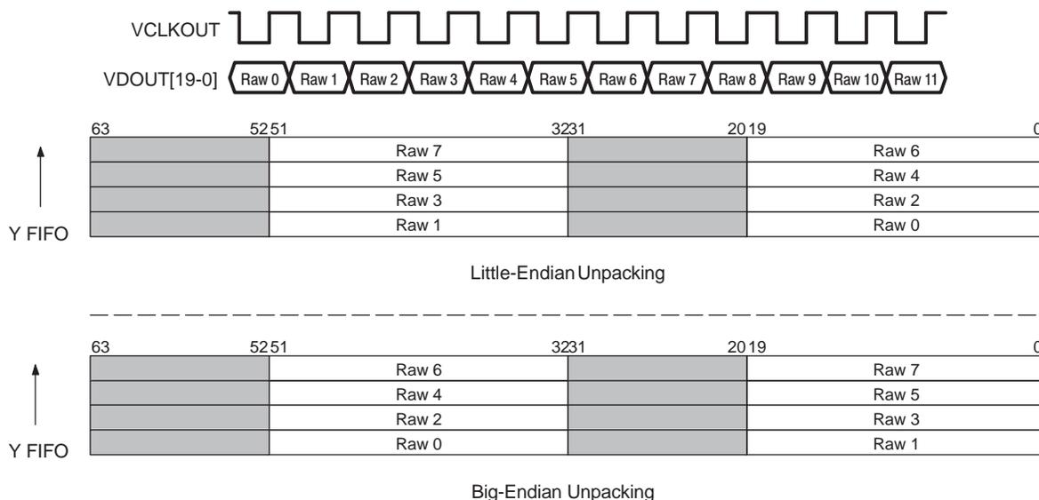
In 8-bit raw  $\frac{3}{4}$  mode, three samples are unpacked from the FIFO and the remaining byte is ignored. This is shown in Figure 4-30.
