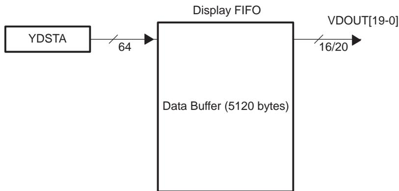
For Y/C video display, the FIFO is configured as a single channel split into separate Y, Cb, and Cr buffers with separate read pointers and write registers (YDSTA, CBDST, and CRDST). Figure 1-10 shows how Y data is output on the VDOOUT[9-0] half of the bus and Cb/Cr data is multiplexed and output on the VDOOUT[19-10] half of the bus.
