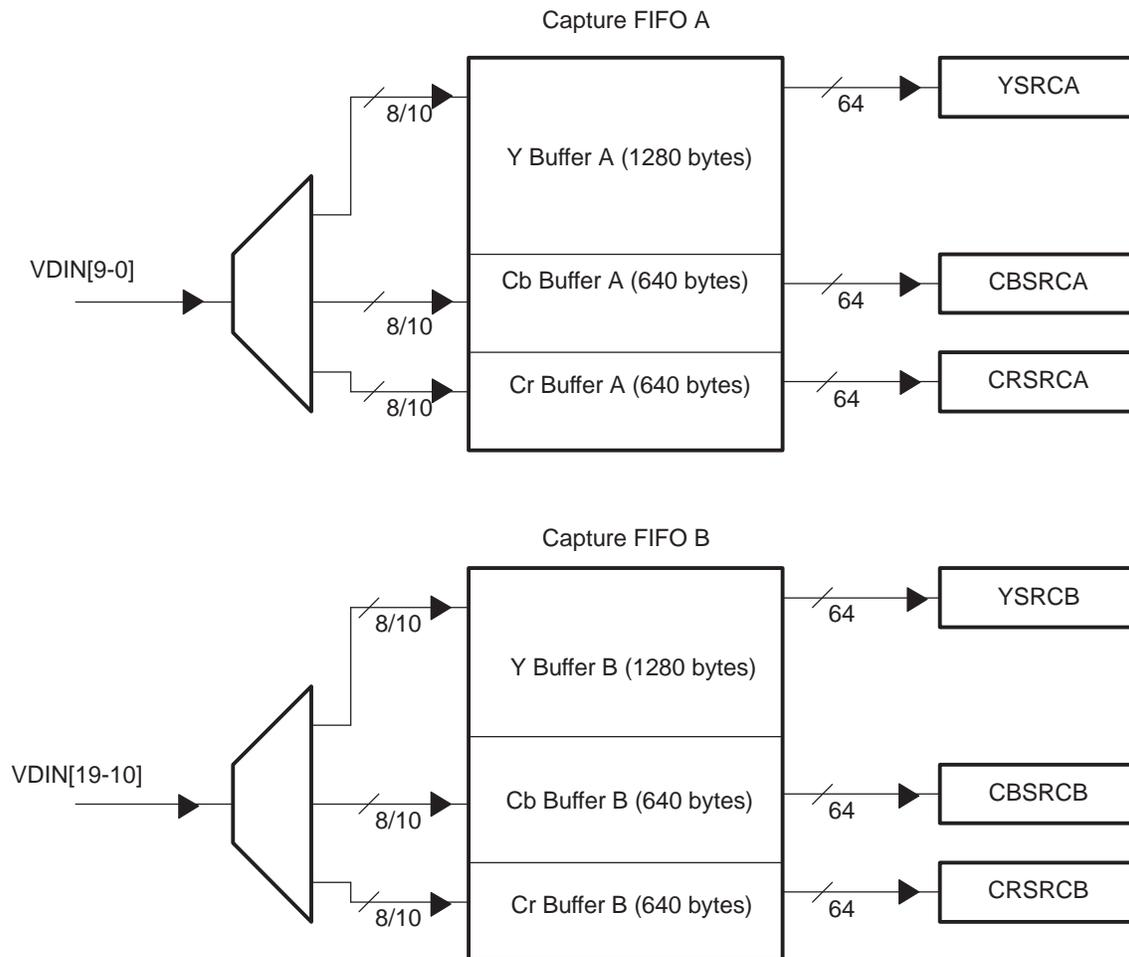
For 8/10-bit raw video, the FIFO is split into channel A and B, as shown in [Figure 1-3](#). Each FIFO is clocked independently with the channel A FIFO receiving data from the VDIN[9-0] half of the bus and the channel B FIFO receiving data from the VDIN[19-10] half of the bus. Each channel's FIFO has a separate write pointer and read register (YSRCx). The FIFO configuration is identical for TSI capture, but channel B is disabled.
