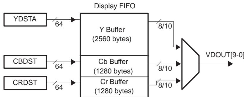
For 8/10-bit raw video, the FIFO is configured as a single buffer as shown in [Figure 1-7](#). The FIFO outputs data on the VDOOUT[9-0] half of the bus. The FIFO has a single read pointer and write register (YDSTA).
