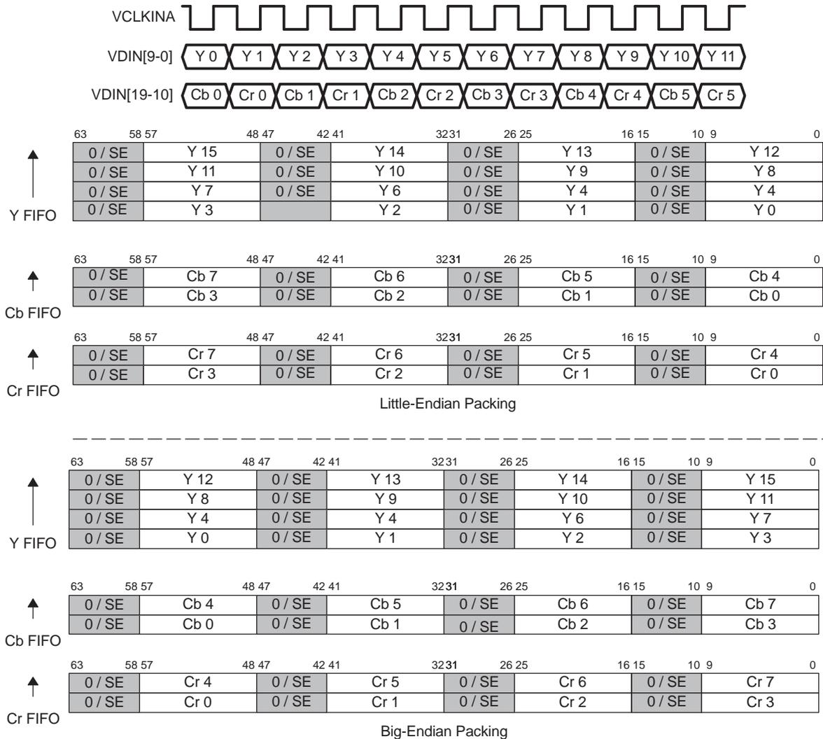
The 10-bit Y/C dense mode uses three FIFOs for color separation. Three samples are packed into each word with zero extension to provide increased DMA bandwidth as shown in Figure 3-7.
