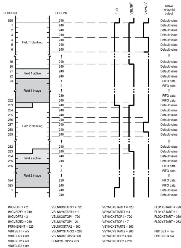
A Assumes VCT1P bit in VPCTL is set to 1 (active-low output). VSYNC output when VCTL1S bit in VDCTL is set to 00, VBLNK output when VCTL1S bit is set 01.
