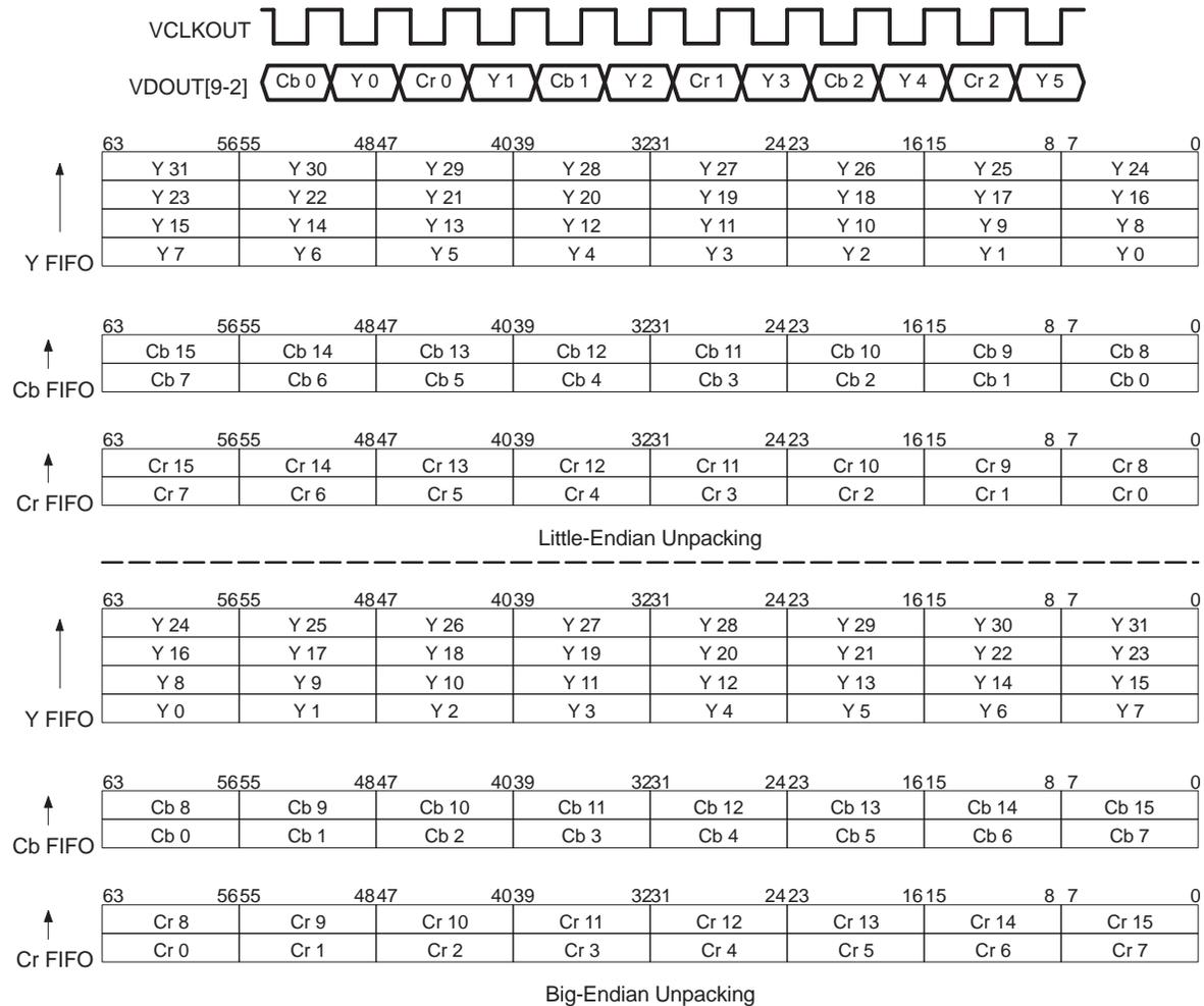
For 10-bit BT.656 operation, two samples are unpacked from each word as shown in [Figure 4-13](#).
