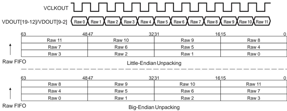
The FIFO unpacking for 20-bit raw format is shown in Figure 4-29. One sample is unpacked from each word of the FIFO.
