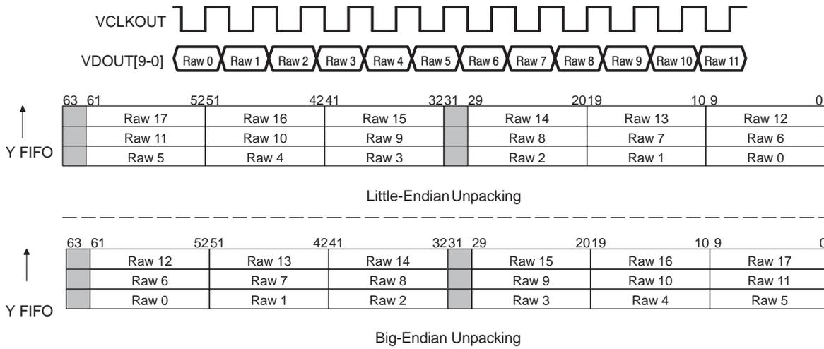
Figure 4-28 shows the 16-bit raw mode. Two samples are unpacked from each word of the FIFO.
