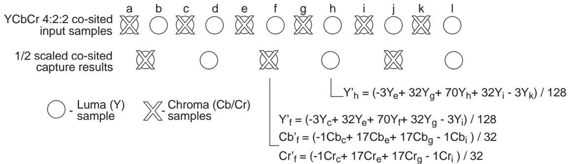
Figure 3-14. 1/2 Scaled Chrominance Re-sampled Filtering
