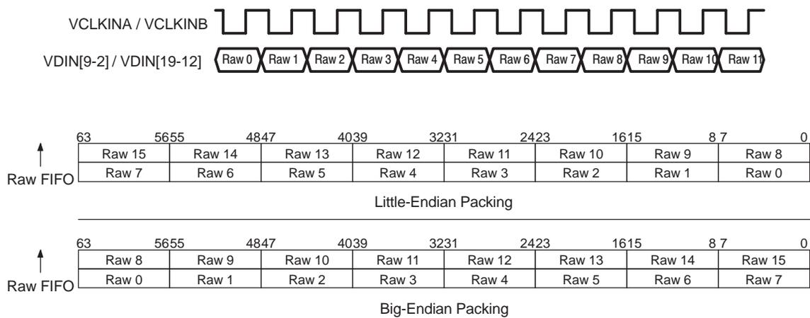
The 10-bit raw data mode stores all data into a single FIFO. Two samples are packed into each word with zero or sign extension as shown in Figure 3-18.
