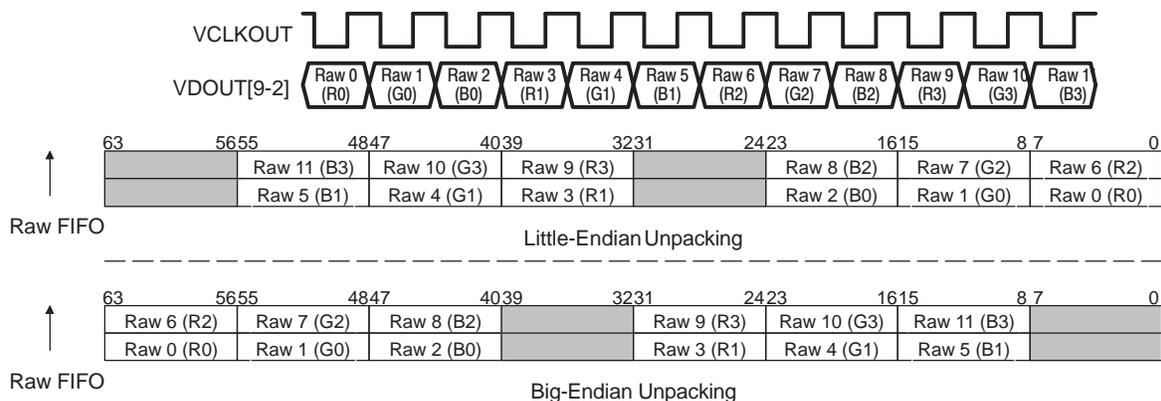
In 10-bit raw  $\frac{3}{4}$  mode, three samples are unpacked from every double word of the FIFO and the remaining halfword is ignored. This is shown in Figure 4-31.
