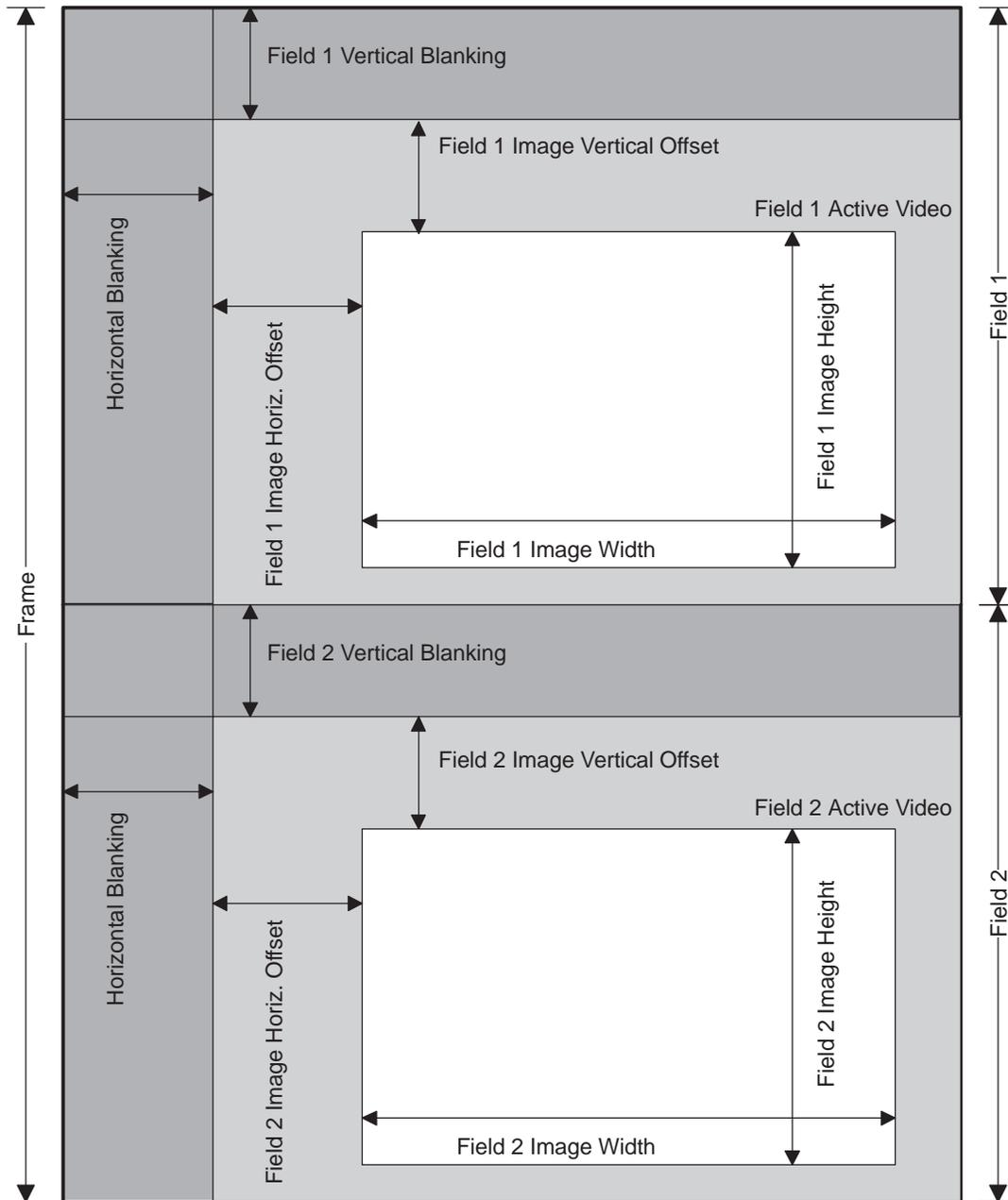
**Figure 4-4. Progressive Blanking Intervals and Video Area**
