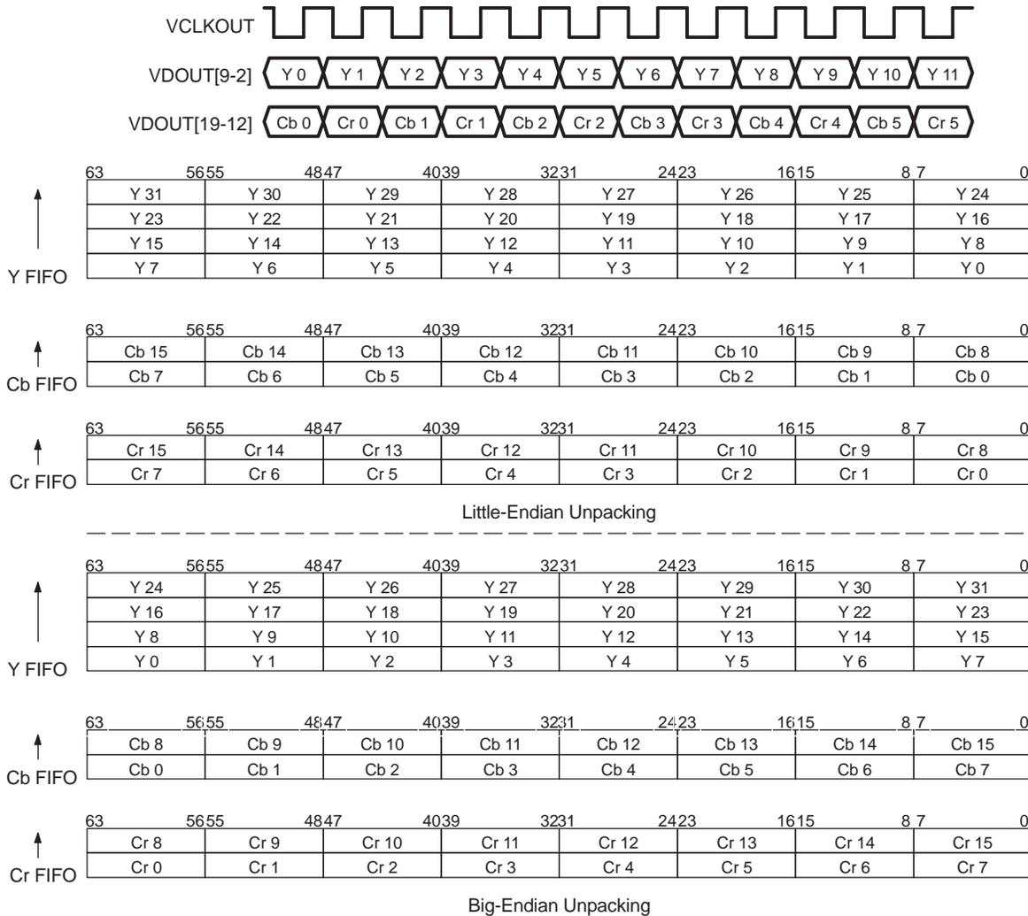
For 10-bit operation, two samples are unpacked from each FIFO word. This is shown in [Figure 4-17](#).
