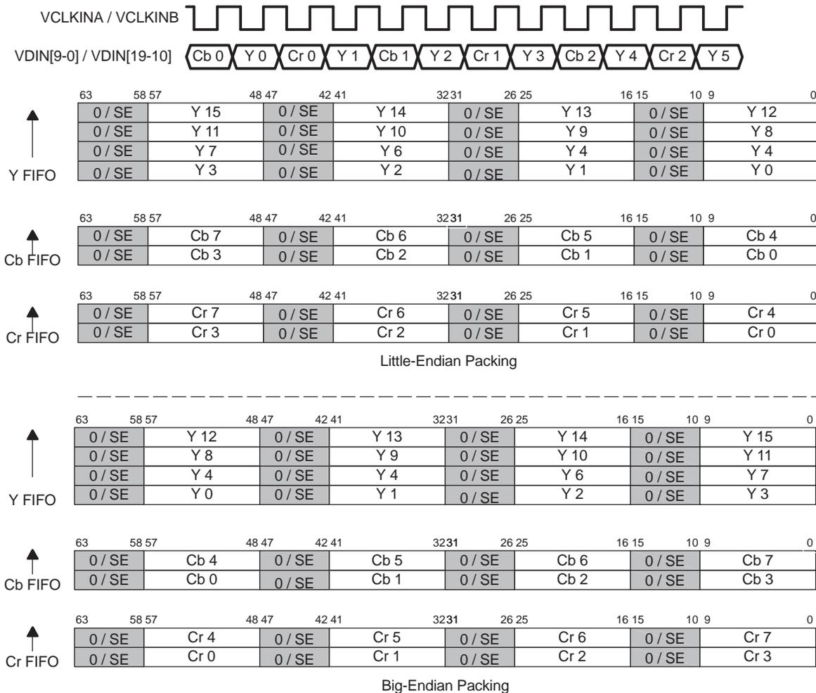
The 10-bit BT.656 dense mode uses three FIFOs for color separation. Three samples are packed into each word with zero extension to provide increased DMA bandwidth as shown in Figure 3-4.
