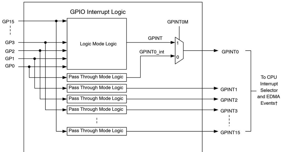
† All GPINT $n$  are synchronization events to the EDMA. Only GPINT0 and GPINT[4–7] are available as interrupts to the CPU.
