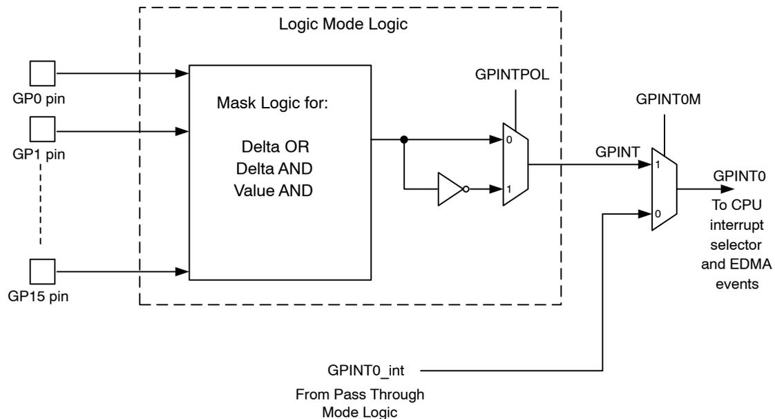
The GPINT generation operates in one of three modes: Delta OR, Delta AND, or Value AND. The GPINT generation is configured via two control bits in GPGC, GPINTDV and LOGIC, in addition to the mask bits in GPHM and GPLM. The GPINTDV bit in GPGC divides the logic mode into either Delta or Value mode as follows:
