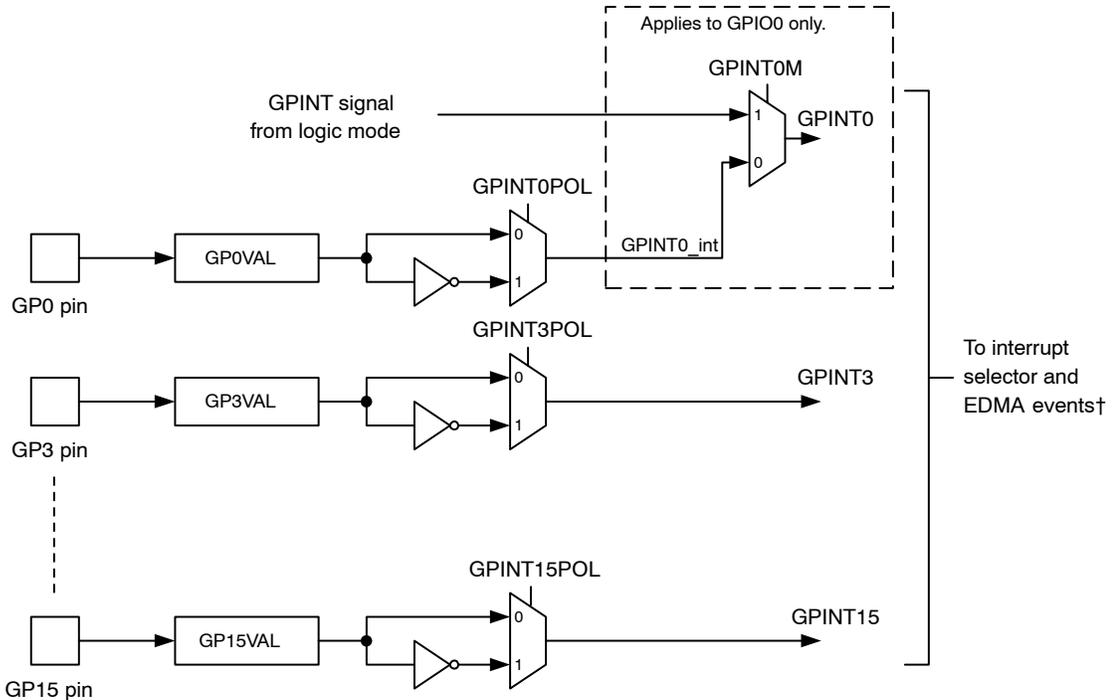
† All GPINTn are synchronization events to the EDMA. Only GPINT0 and GPINT[4–7] are available as interrupts to the CPU.
