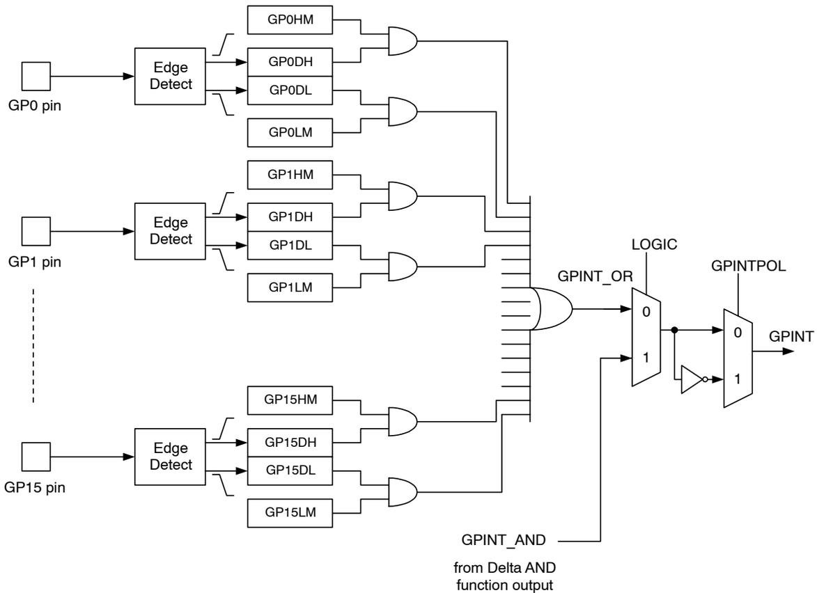
In addition, GPHM and GPLM must be configured properly to enable the corresponding GPDH and GPDH bits to be inputs to the logic function. The following examples show the GPHM and GPLM setup. All the given GPIO pins in these examples are enabled as inputs (GPXEN bit = 1, GPXDIR bit = 0).
