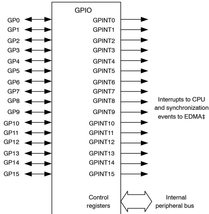
† Some of the GP $n$  pins are MUXed with other device signals. The number of available GP $n$  pins is device specific. Refer to the device-specific datasheet for details.
