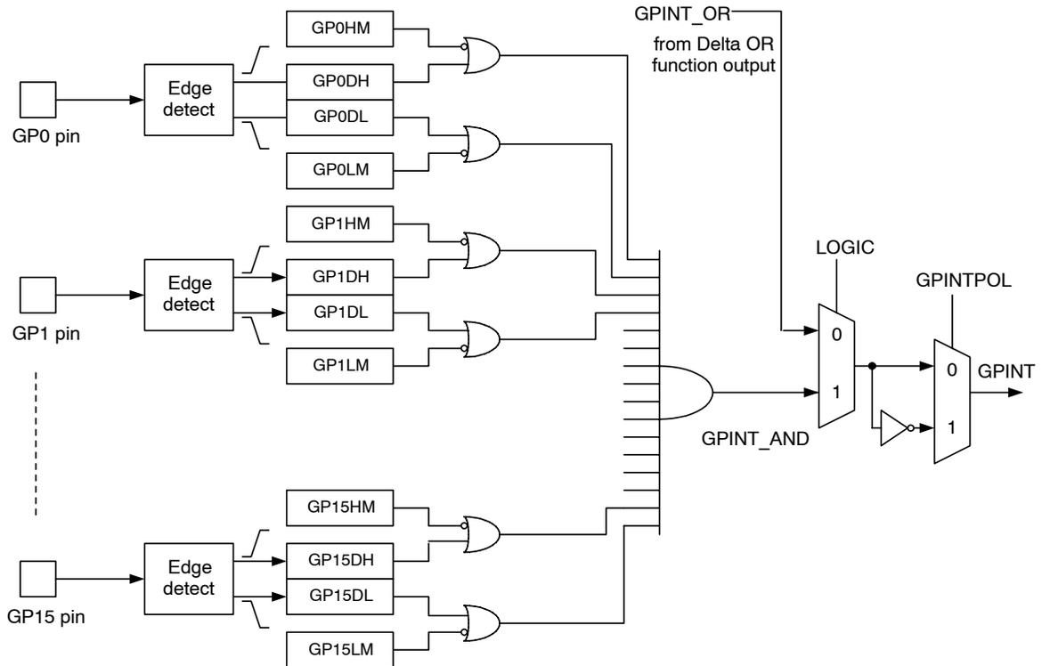
**Note:** The functional block diagram shows the mask logic as an OR with an inverter on the mask bit. This forces the OR to evaluate true when the mask bit is disabled. This is strictly a functional block diagram. The actual implementation prevents the GPINT from being asserted in the case that all of the mask bits are disabled.
