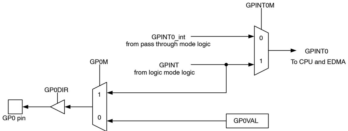
When GP0 is configured as an output (GP0DIR = 1), the GP0M bit controls whether the GP0 signal operates in GPIO mode or in logic mode. In GPIO mode (GP0M = 0), the value of the GP0VAL bit is driven out on GP0. In logic mode (GP0M = 1), GPINT is driven out on GP0. When GP0 is configured as an input, GP0M has no effect.
