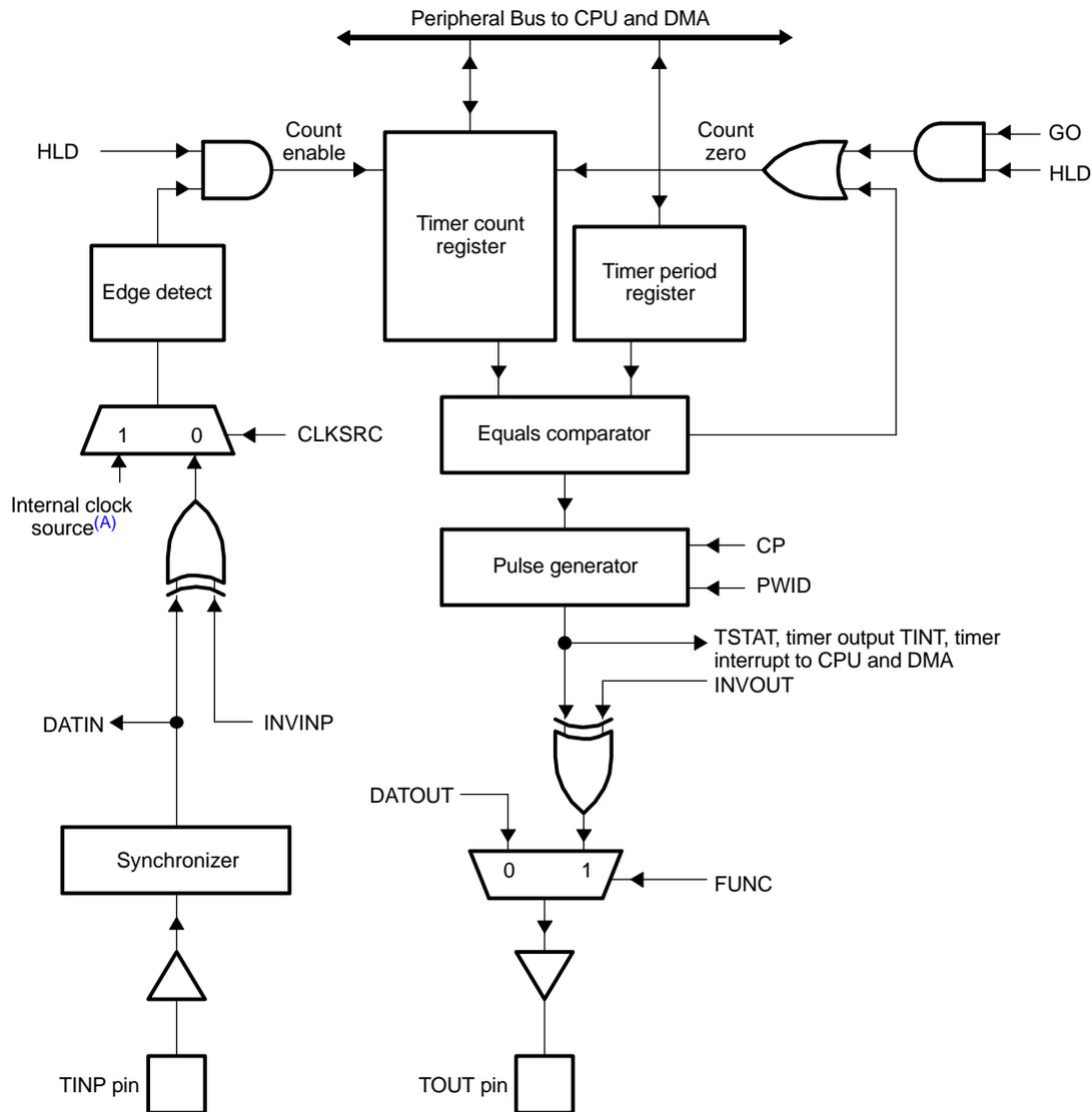
A C62x/C67x DSP uses CPU/4 clock as the internal clock source to the timer. C64x DSP uses CPU/8 clock as the internal clock source to the timer.
