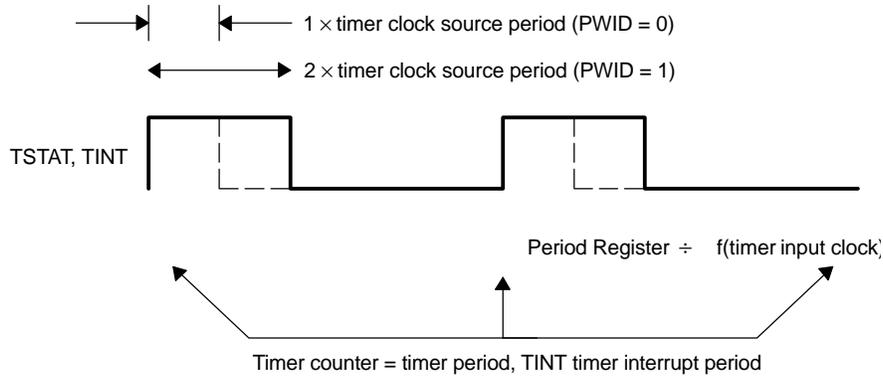
**Figure 3. Timer Operation in Clock Mode (CP = 1)**
