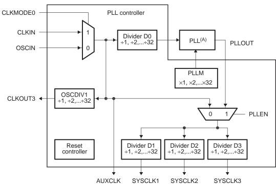
Figure 1. PLL Controller Block Diagram
