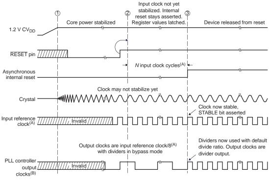
Figure 2. Reset Controller Lengthening the Internal Reset Signal
