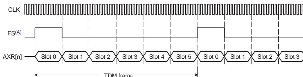
A FS duration of slot is shown. FS duration of single bit is also supported.
