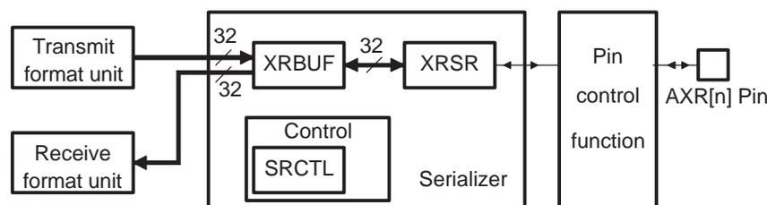
For receive, data is shifted in through the AXR[n] pin to the shift register XRSR. Once the entire slot of data is collected in the XRSR, the data is copied to the data buffer XRBUF. The data is now ready to be read by the DSP through the RBUF register, which is an alias of the XRBUF for receive. When the DSP reads from the RBUF, the McASP passes the data from RBUF through the receive format unit and returns the formatted data to the DSP.
