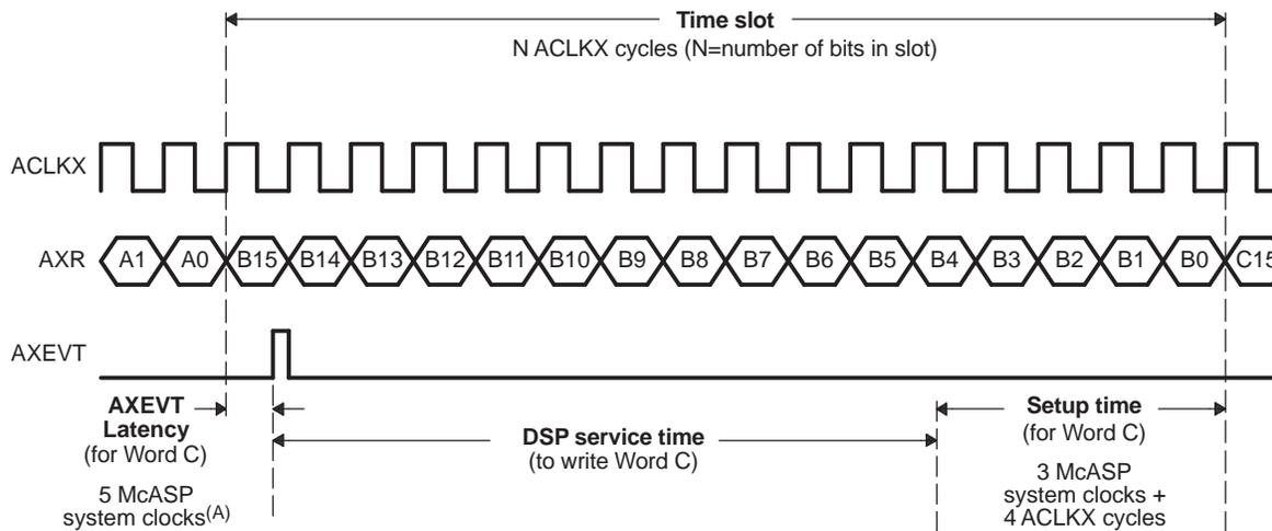
A Refer to the device-specific data manual for the McASP system clock source. This is not the same as AUXCLK. For example, the C6713 DSP uses SYSCLK2 as the McASP system clock source.
