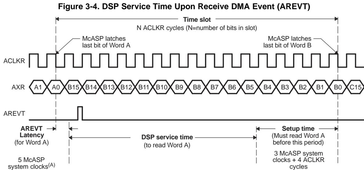
A Refer to the device-specific data manual for the McASP system clock source. This is not the same as AUXCLK. For example, the C6713 DSP uses SYSCLK2 as the McASP system clock source.
