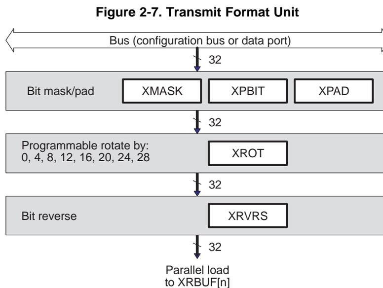
The bit mask and pad stage includes a full 32-bit mask register, allowing selected individual bits to either pass through the stage unchanged, or be masked off. The bit mask and pad then pad the value of the masked off bits by inserting either a 0, a 1, or one of the original 32 bits as the pad value. The last option allows for sign-extension when the sign bit is selected to pad the remaining bits.
