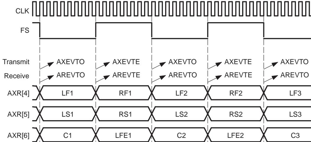
You can either use the DMA to service the McASP upon events AXEVT and AREVT (Figure 3-5) or upon events AXEVTO, AREVTO, AXEVTE, and AREVTE (Figure 3-6).
