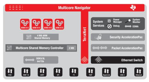
▲ Figure 3 – TI's AM5K2E04 SoC with four Cortex-A15 processors
