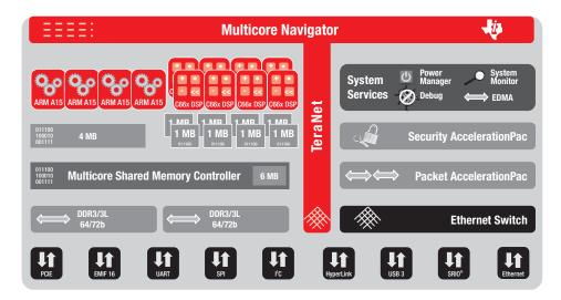
▲ Figure 2 – TI's 66AK2H12 SoC with four Cortex-A15 processors and eight C66x DSP cores
