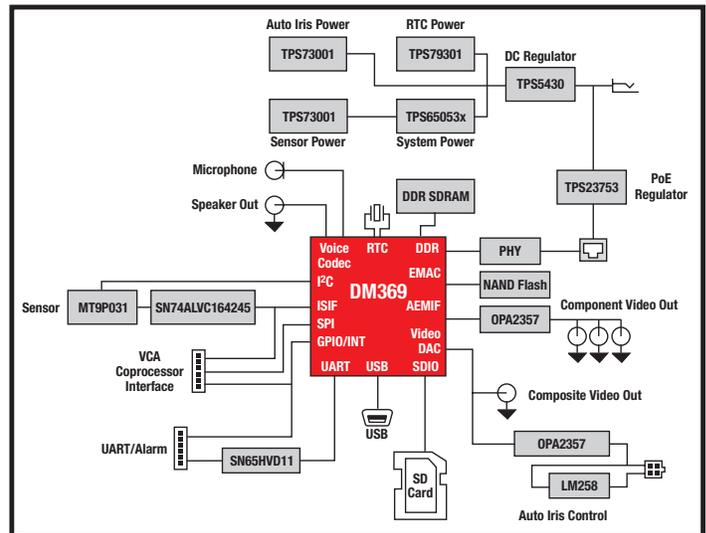
▲ IP camera reference design block diagram: TMSIPCAM369X104
