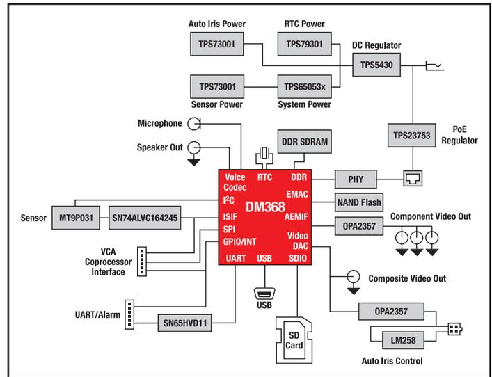
▲ IP camera reference design block diagram: DM368IPNC-MT5
