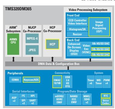
The boxes highlighted in yellow show differences with the TMS320DM355 processor.
