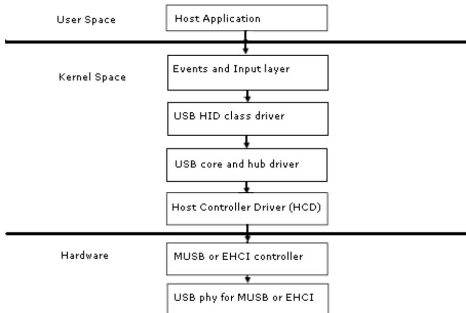
**Figure 10.4. USB Driver: Illustration of HID Driver**
