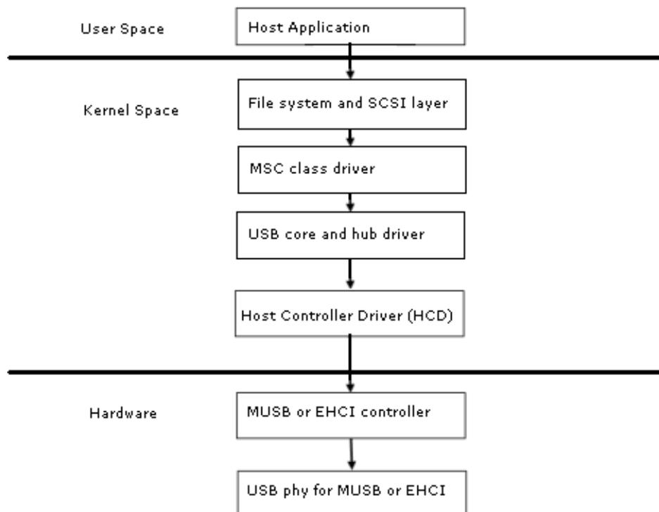
**Figure 10.1. USB Driver: Illustration of Mass Storage Class**
