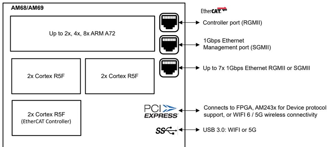
Figure 4-2. Programmable Logic Controller Block Diagram
