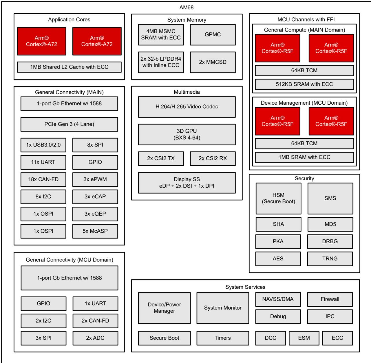
**Figure 2-1. AM68 Block Diagram with Subsystems**
