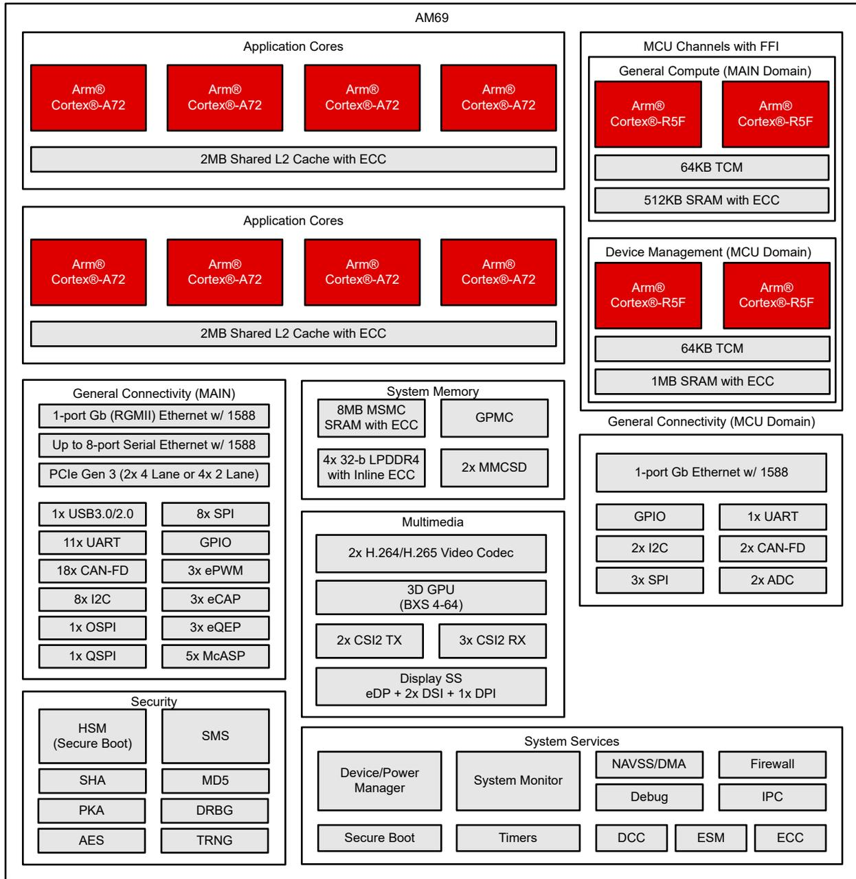
Figure 3-1. AM69 Block Diagram with Subsystems
