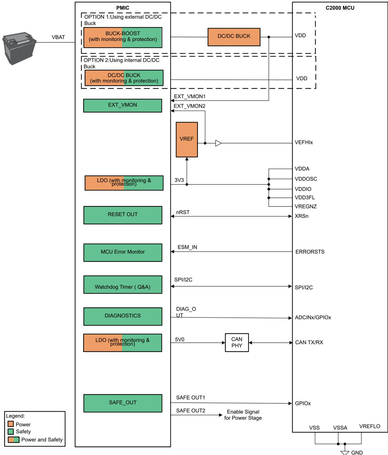
Figure 2-1. ASILD: MCU With External VREFHI and External VREG
