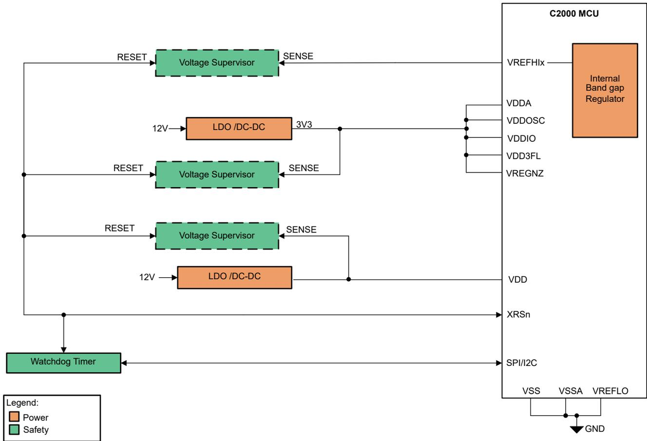
Figure 3-2. Non-Safety: MCU With Internal VREFHI and External VREG
