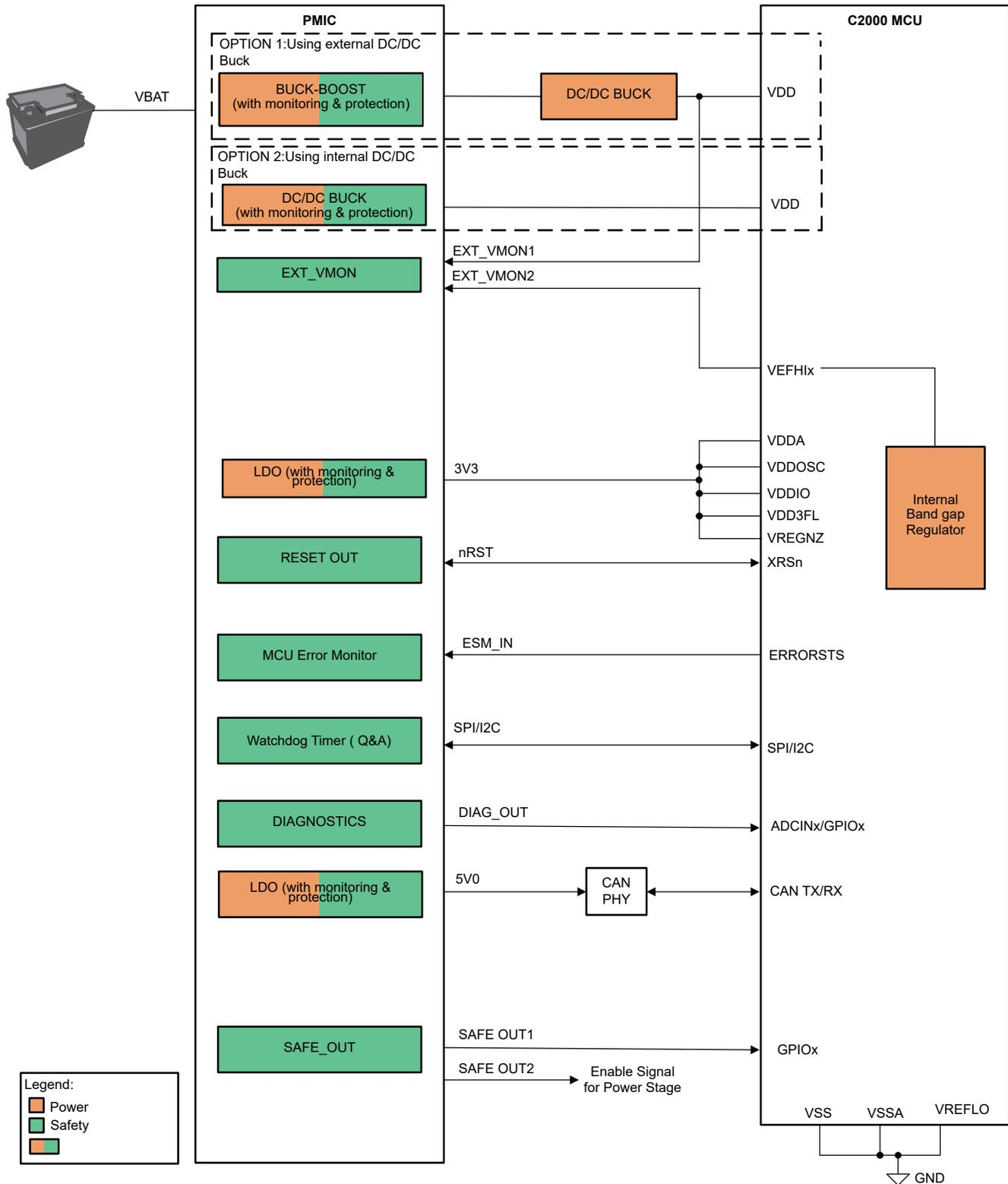
Figure 2-2. ASIL-B: MCU With Internal VREFHI and External VREG
