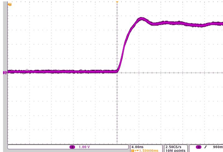
**Figure 4-8. Magnified View of Beginning of TX\_EN Signal for EST Shaped Codesys EtherCAT Main - 1.5 ms Cycle Time, Oscilloscope in Persistence Mode**
