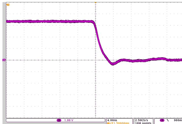
**Figure 4-9. Magnified View of Ending of TX\_EN Signal for EST Shaped Codesys EtherCAT Main - 1.5 ms Cycle Time, Oscilloscope in Persistence Mode**
