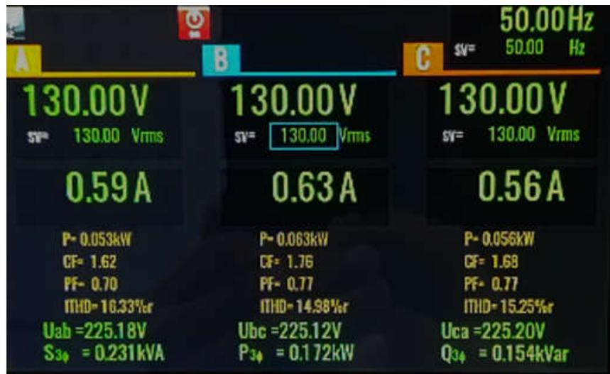
Figure 5-21. ITHD and PF Values at 130-V AC Input With a Constant Bus Voltage Reference Value
