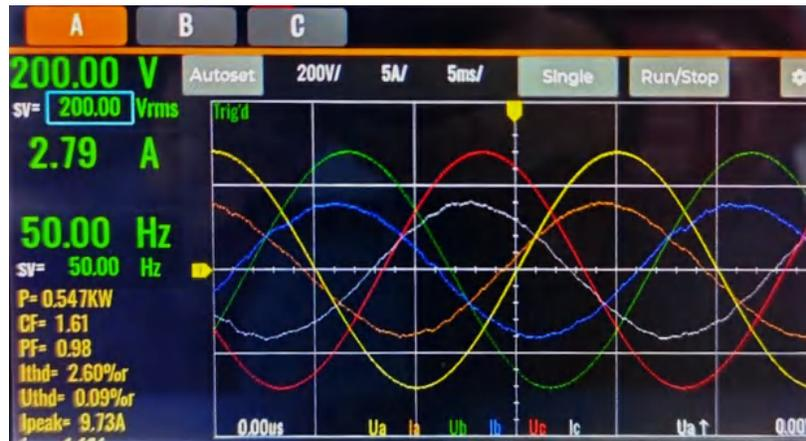
**Figure 5-16.  $I_a$ ,  $I_b$ ,  $I_c$  Waveforms on the Grid-side of TIDA Hardware in PFC Mode for 200-V AC Input**
