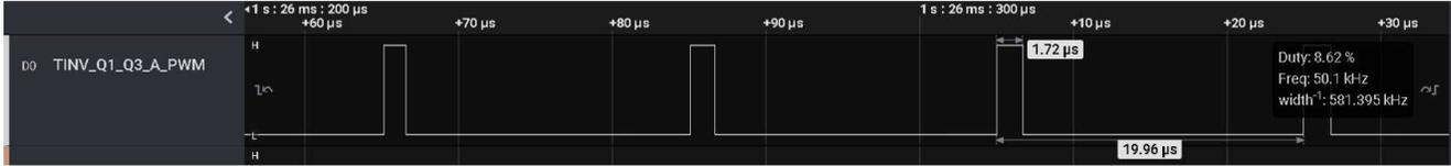
**Figure 3-10. CMPA Value Alters the Duty Cycle of the EPWM0 Waveform**
