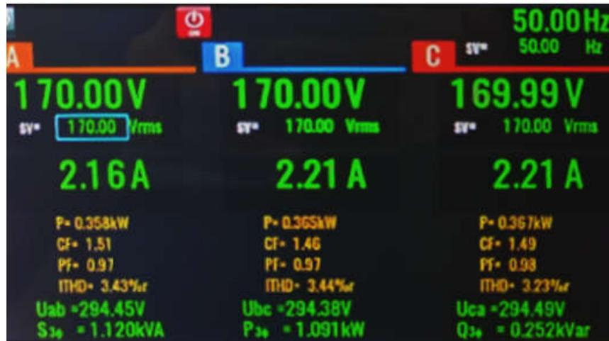
Figure 5-20. ITHD and PF Values at 200-V AC Input With a Constant Bus Voltage Reference Value
