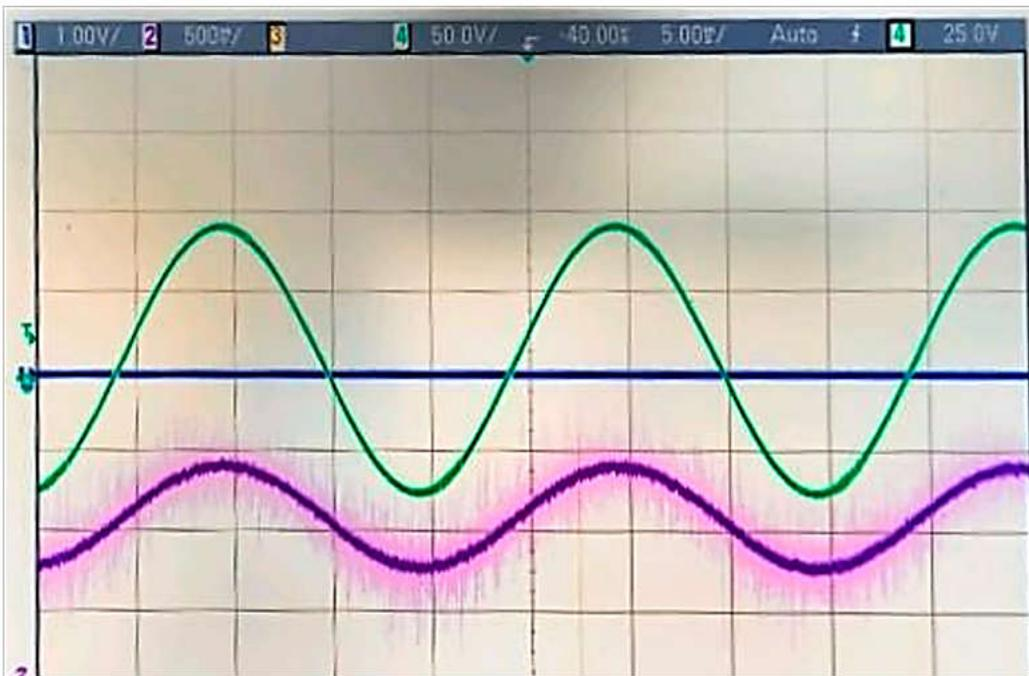
Figure 5-2. SDFM Channel A Sensed Signal Plotted on Oscilloscope Using DAC
