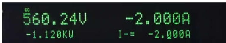
Figure 5-19. Output Bus Voltage of PFC Hardware for 130-V AC Input
