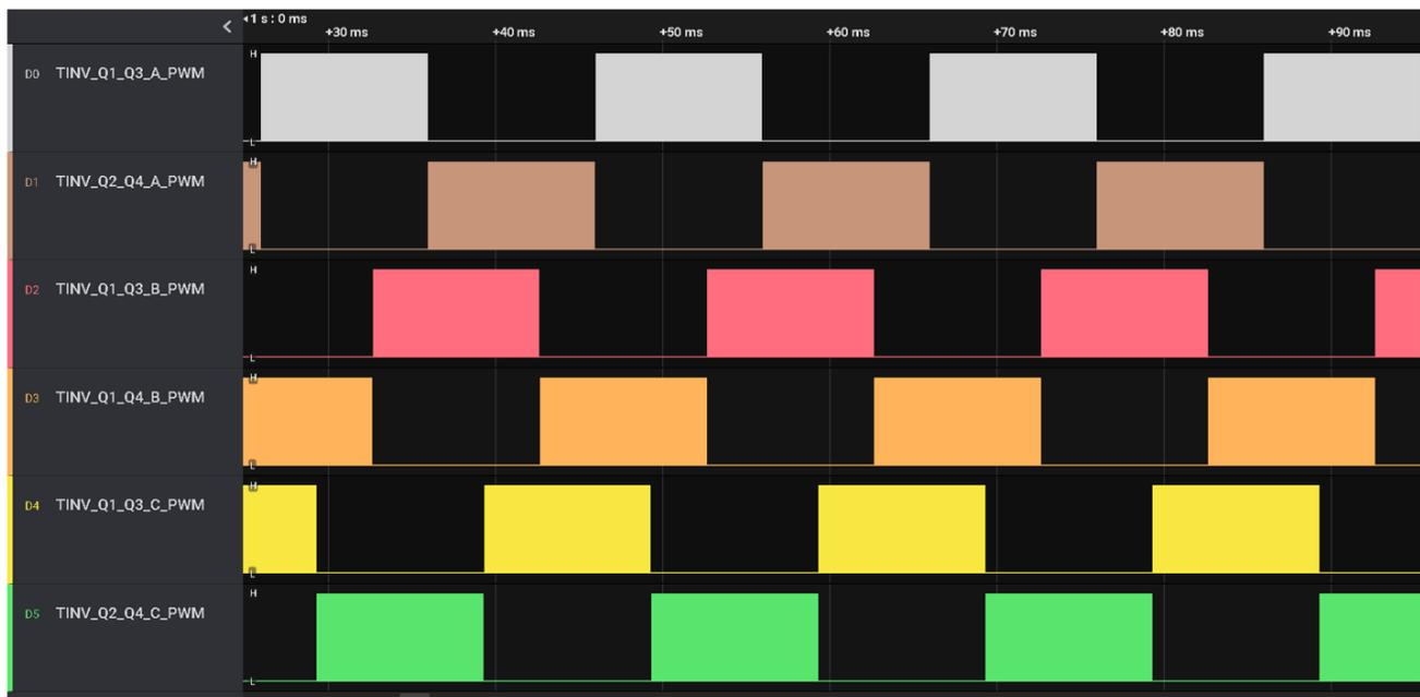
**Figure 5-1. Lab 1 EPWM Output Waveforms**
