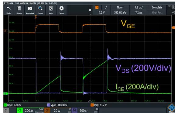
Figure 5-6. Strong Drive With a 0.5-Ω Gate Resistor
