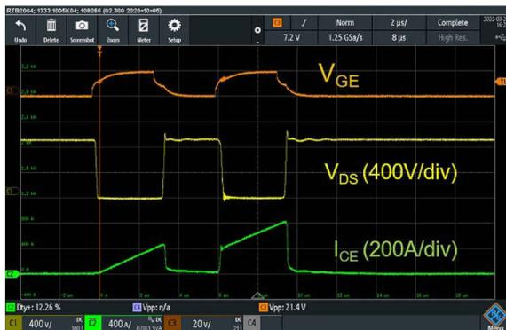
Figure 5-5. Weak Drive With a 5.5-Ω Gate Resistor
