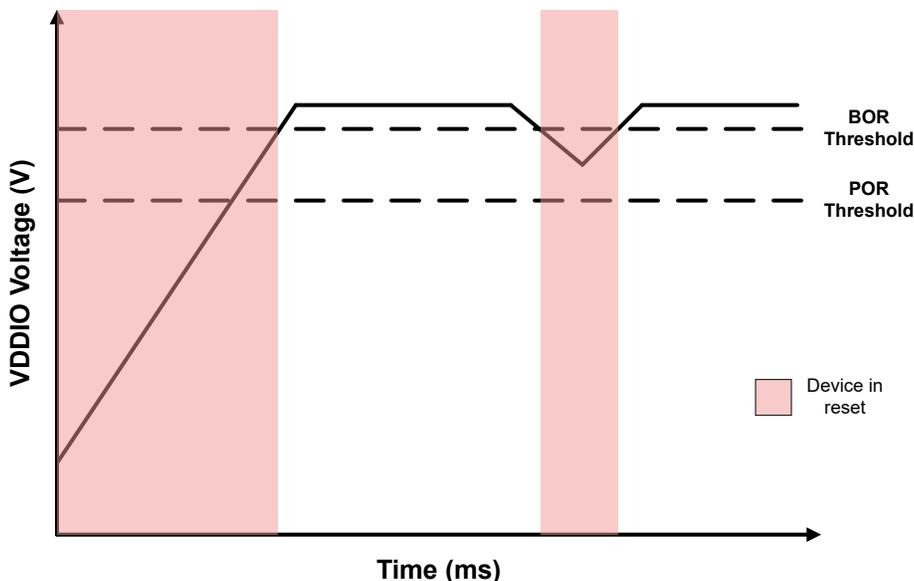
Figure 3-11. Device Boot Reset Thresholds
