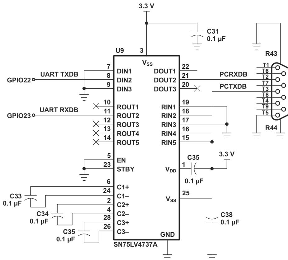
Figure 3-6. Typical RS-232 Transceiver
