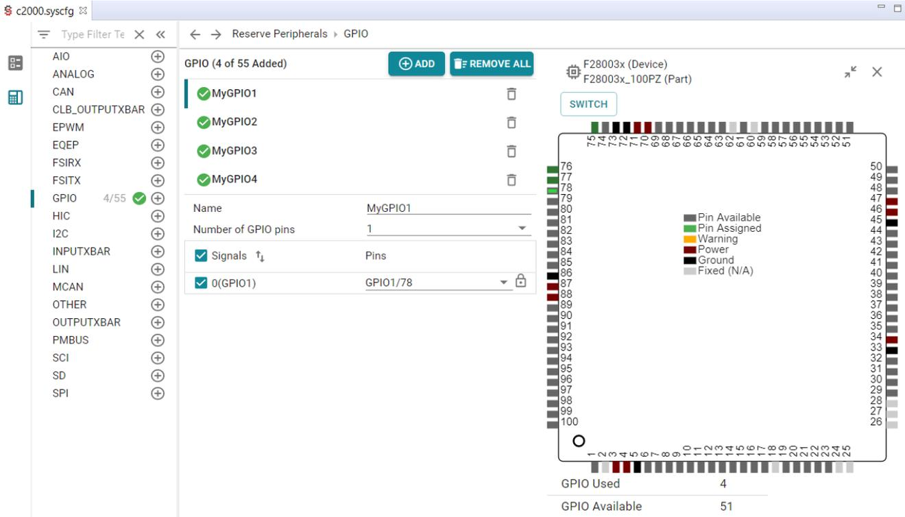
Figure 3-3. PinMux Tool Within SysConfig
