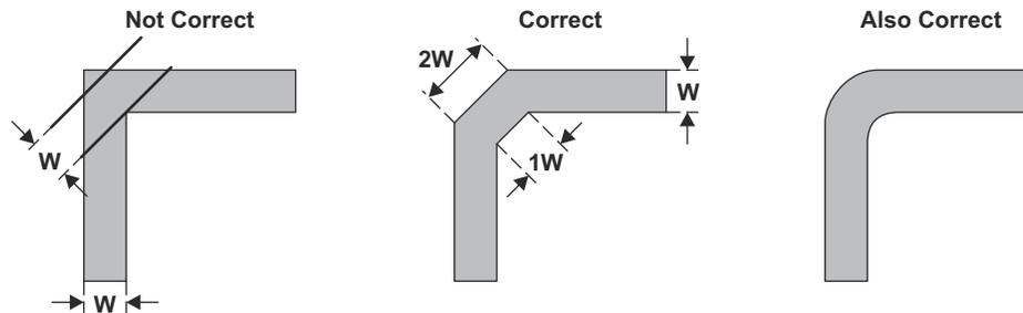
**Figure 4-10. Proper Trace Signal Routing**
