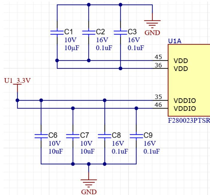
Figure 3-9. Decoupling Capacitors on VDD Pins
