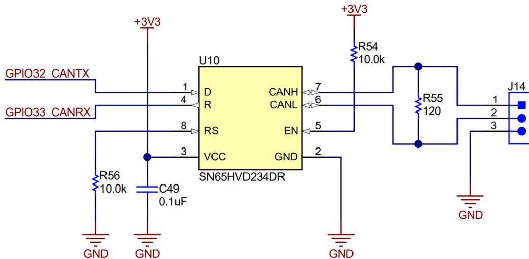
Figure 3-5. CAN Transceiver in LAUNCHXL-F280049C
