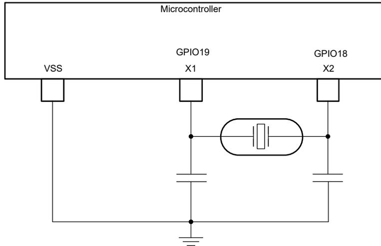
**Figure 3-13. External Crystal Circuit**
