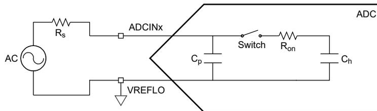
Figure 3-8. ADC Input Model
