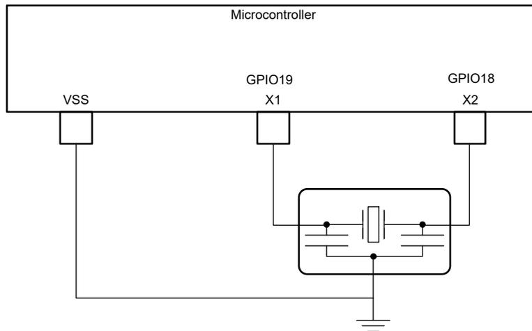
**Figure 3-14. External Resonator Circuit**
