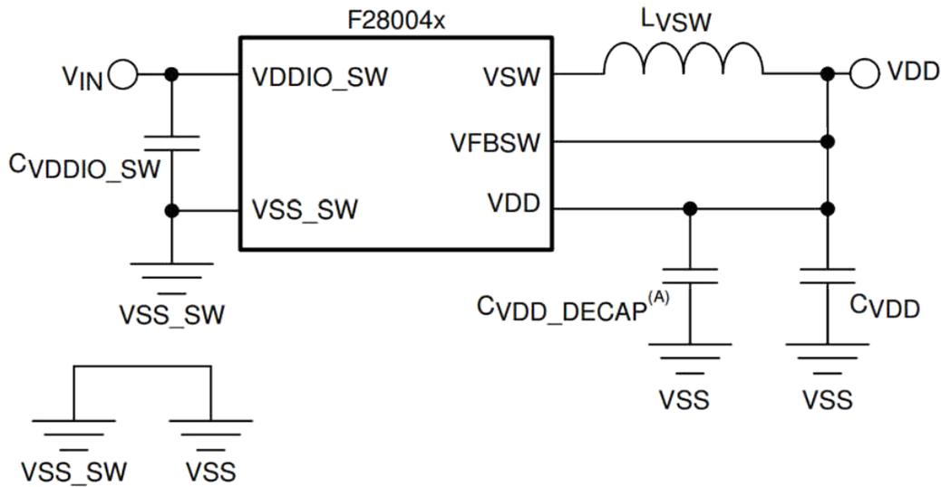
Figure 3-10. DC-DC Regulator Circuit Schematic
