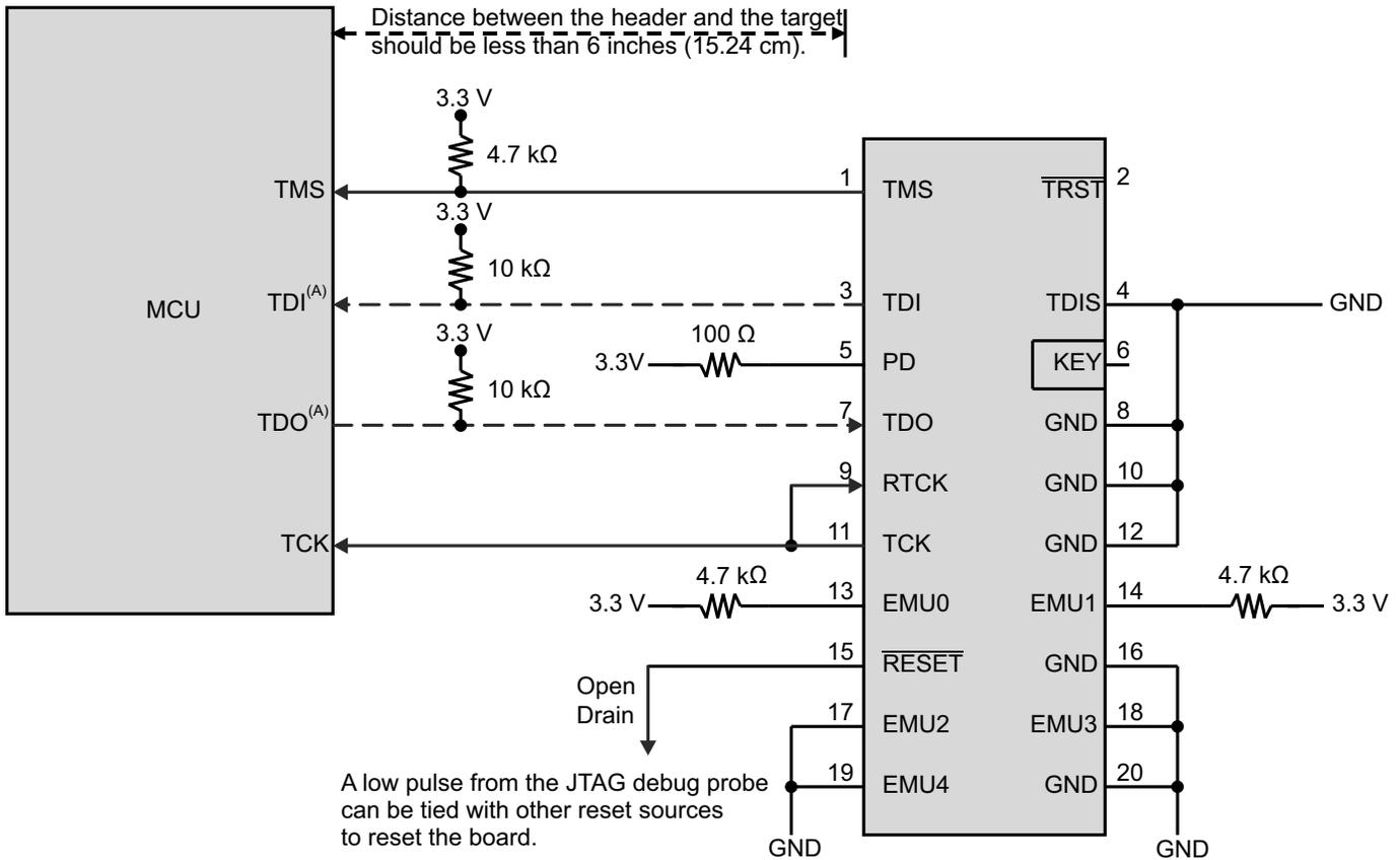
Figure 3-16. Typical JTAG Probe Connections
