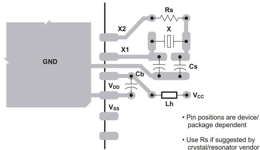
**Figure 4-4. Recommended Oscillator Layout**
