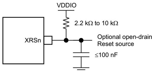
Figure 3-12. External Reset Circuit
