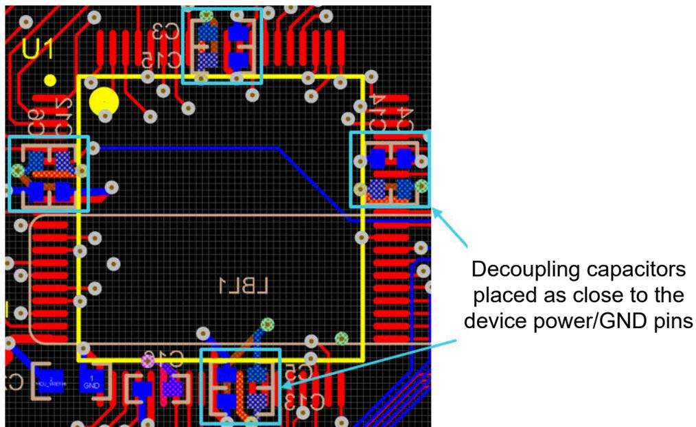
**Figure 4-5. Decoupling Capacitors on Board Layout**
