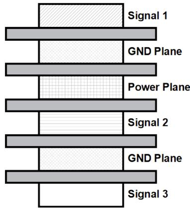
Figure 4-2. Layer Stack-Up for 6-Layer Board
