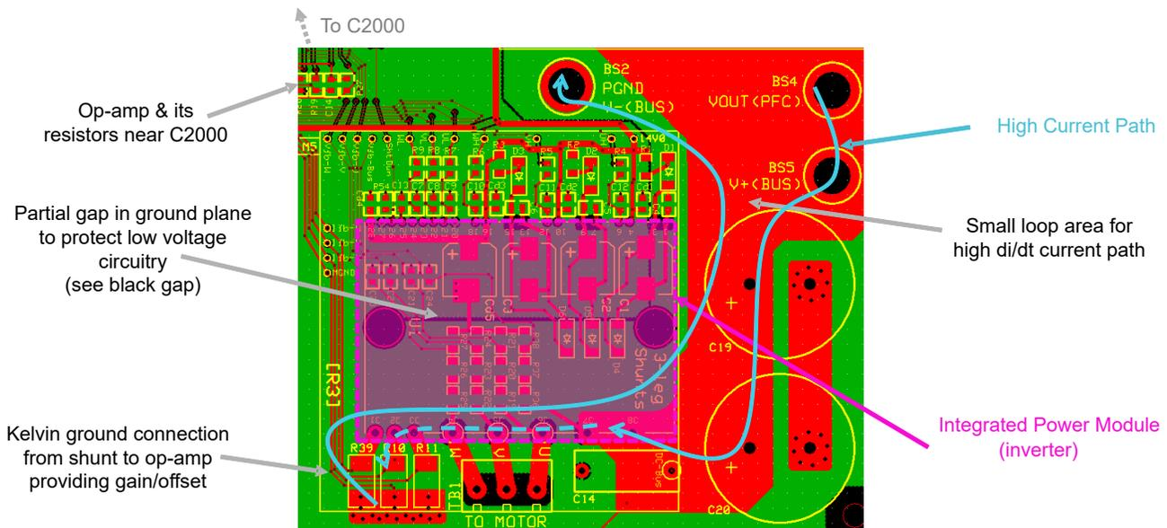
Figure 4-6. Power Electronics on Board Layout
