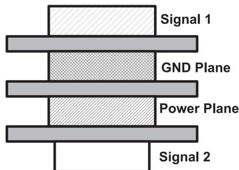
**Figure 4-1. Layer Stack-Up for 4-Layer Board**
