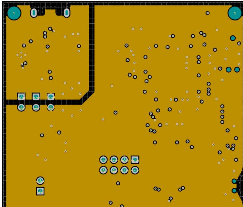
**Figure 4-7. Ground Plane on LaunchPad**
