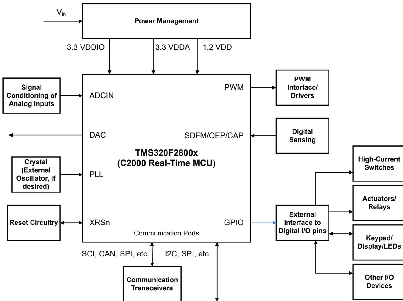
Figure 2-1. Typical TMS320F2800x System
