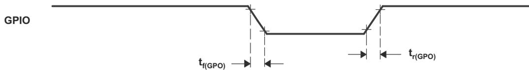
**Figure 3-4. GPIO Output Timing**
