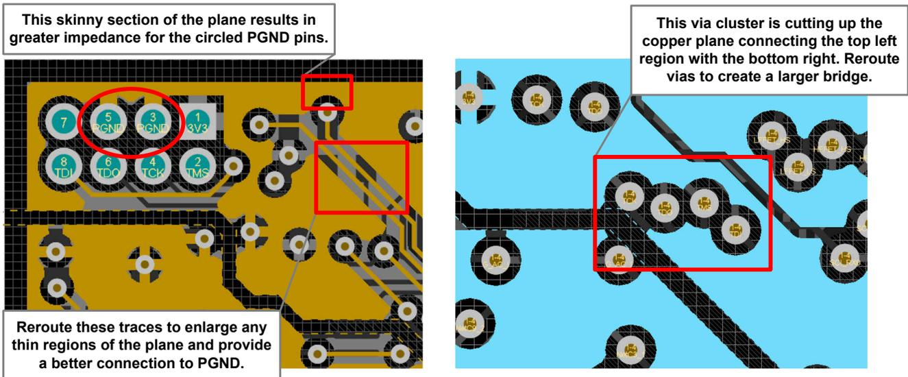
**Figure 4-8. Examples of Cut-Up Ground Planes**
