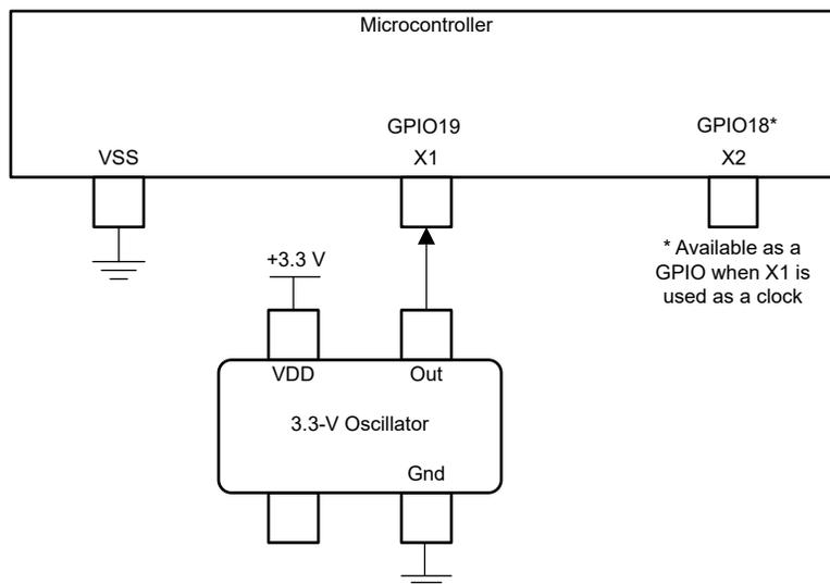
**Figure 3-15. External Oscillator Circuit**
