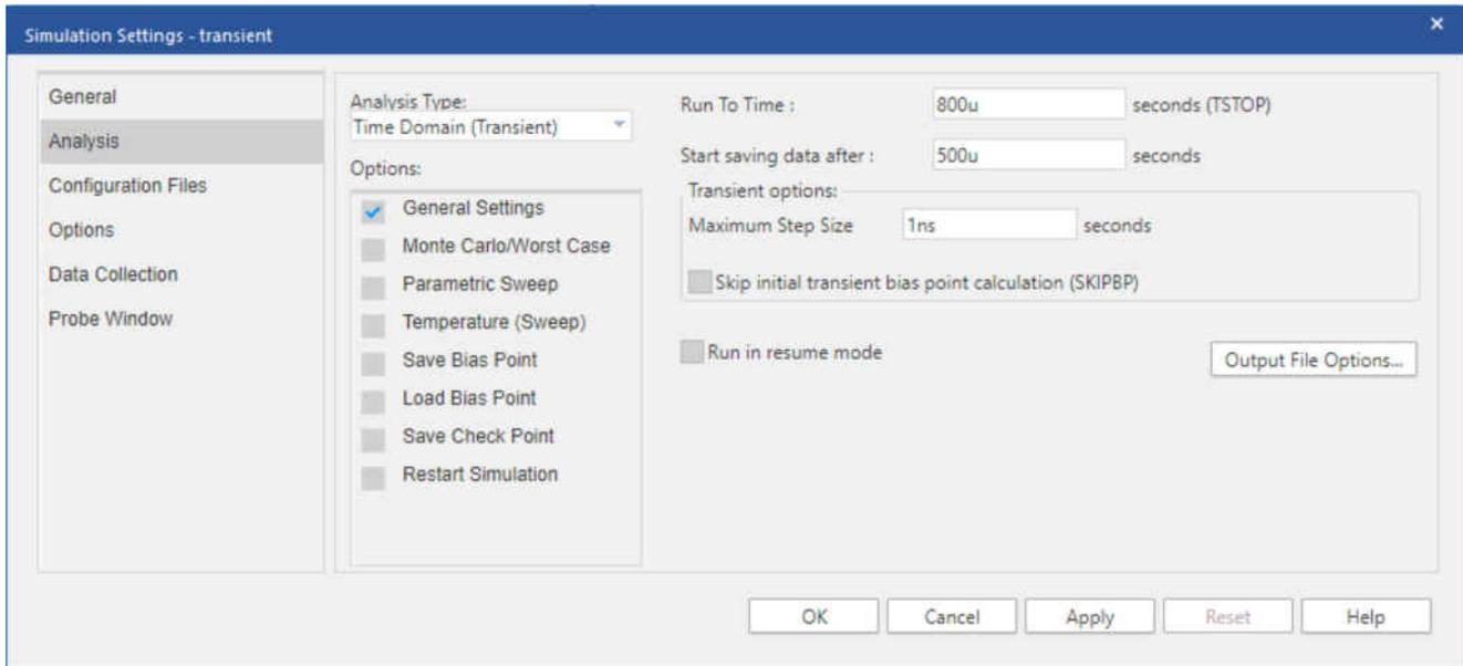
Figure 5-11. Example 3: Simulation Profile
