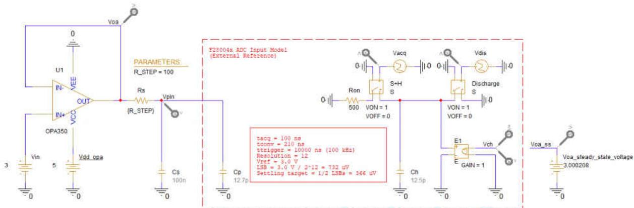
Figure 4-8. Transient Analysis Circuit
