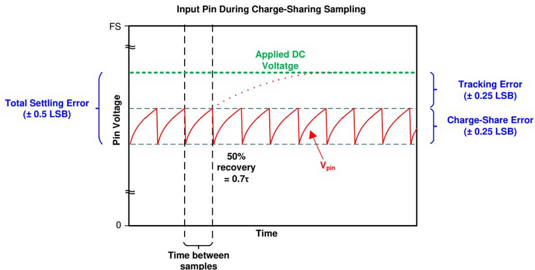
**Figure 2-7. Charge Sharing Steady State With DC Input**
