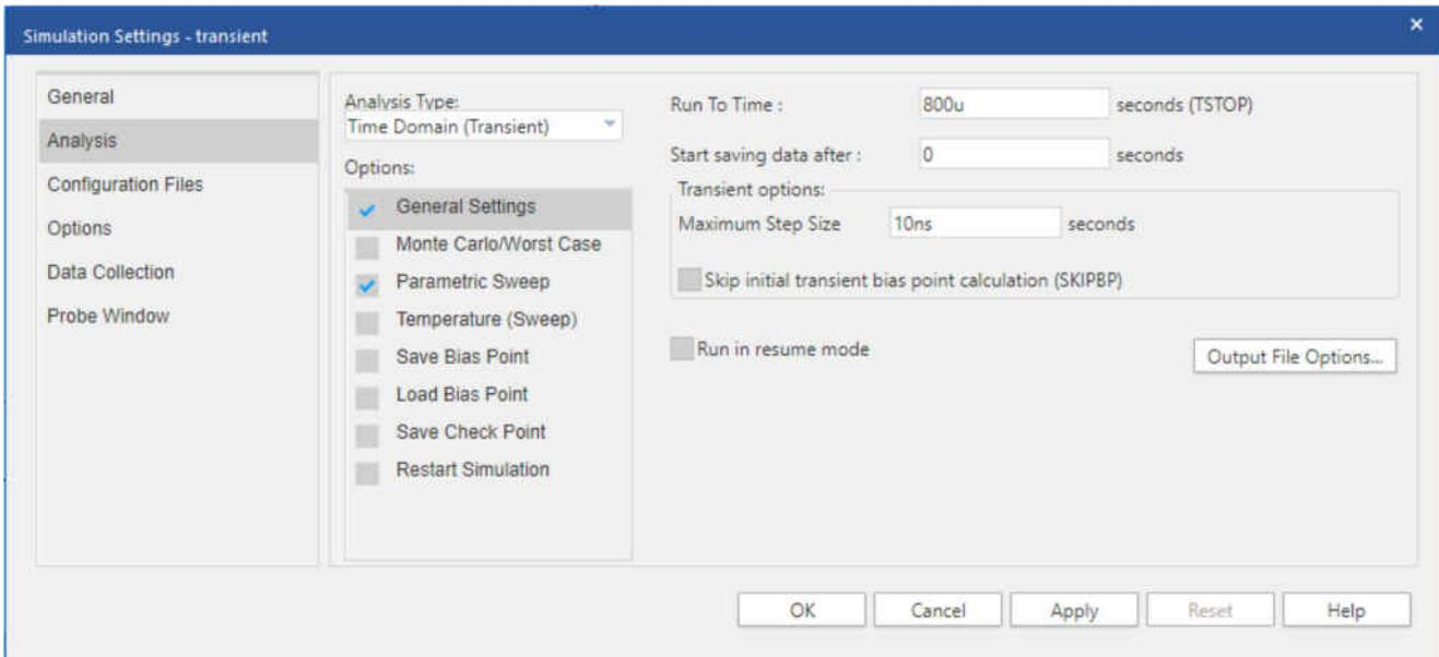
Figure 4-15. Transient Analysis Simulation Profile General Settings
