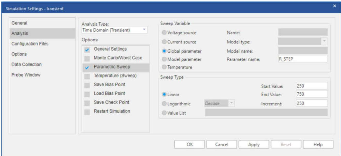
**Figure 4-16. Transient Analysis Simulation Profile Parametric Sweep**
