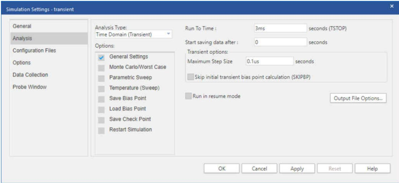
Figure 5-2. Example 1: Simulation Profile
