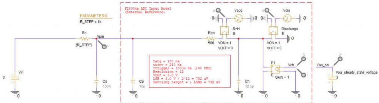
Figure 2-3. ADC Input Circuit With 1 k $\Omega$   $R_s$  and 100 kHz Sample Rate
