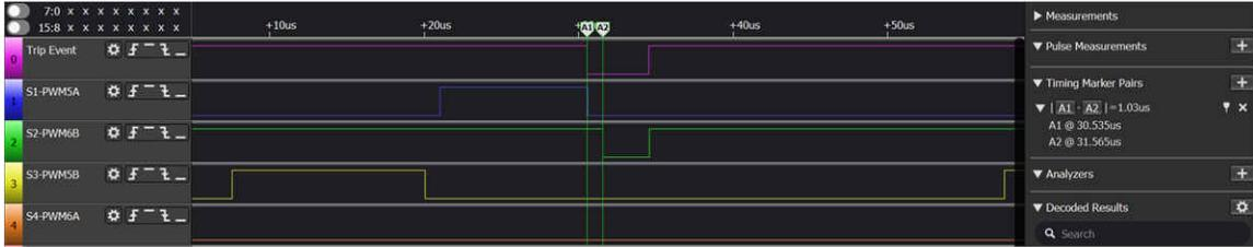
Figure 6-5. PWM5 and PWM6 With Trip Signal During Positive Cycle
