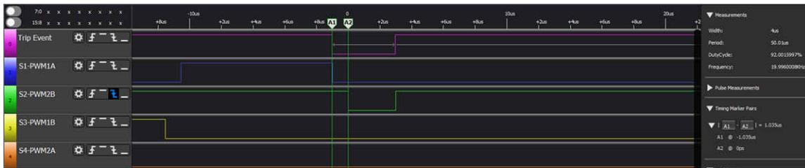
**Figure 6-2. Trip Signal During Positive Cycle**
