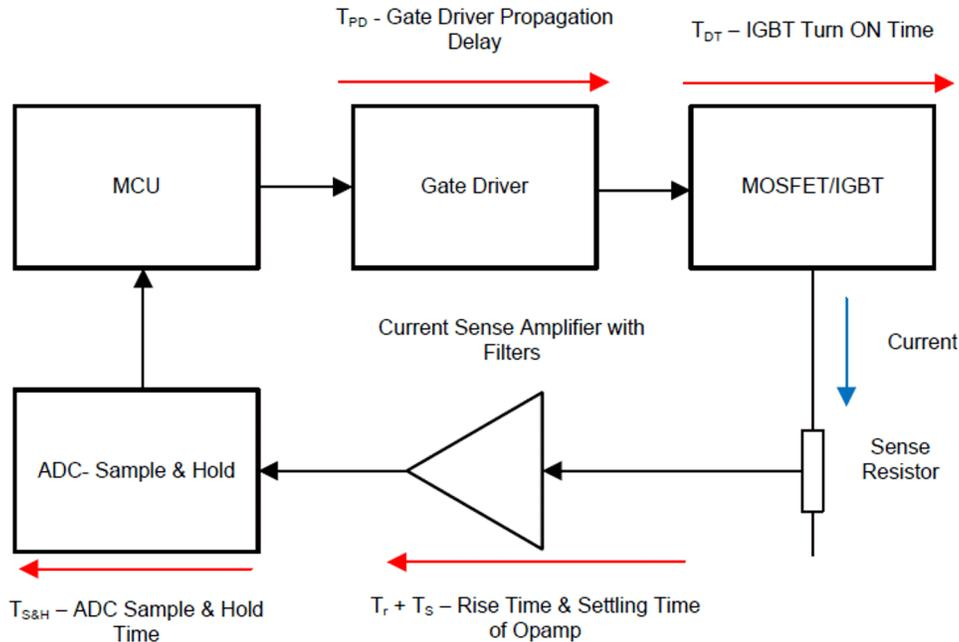
Figure 2-11. Delay in the Current Sensing Loop
