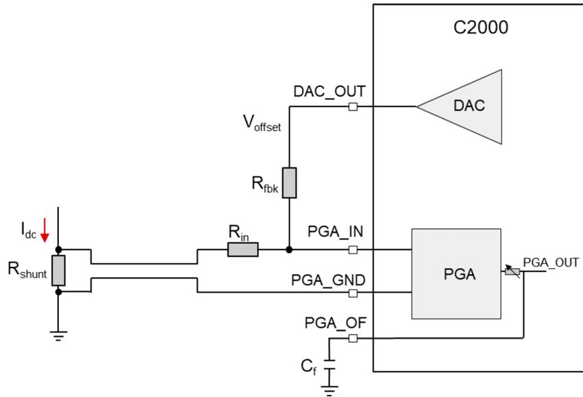
Figure 5-1. Current Sensing Circuit for F2804x With Internal Op-Amp
