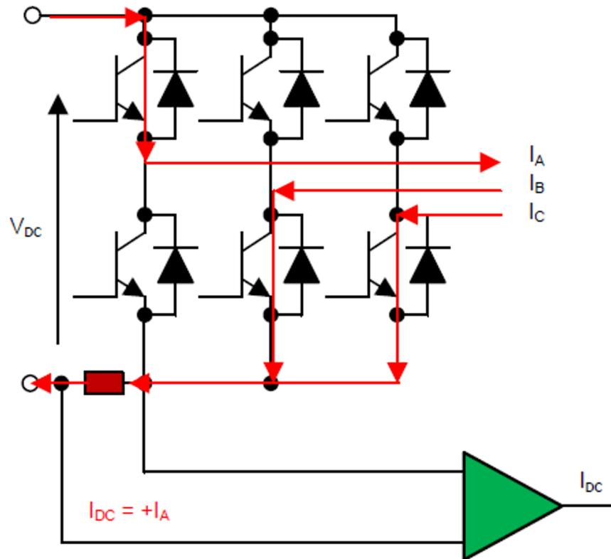
Figure 2-8. Switching State  $S_a, S_b, S_c$ : 100
