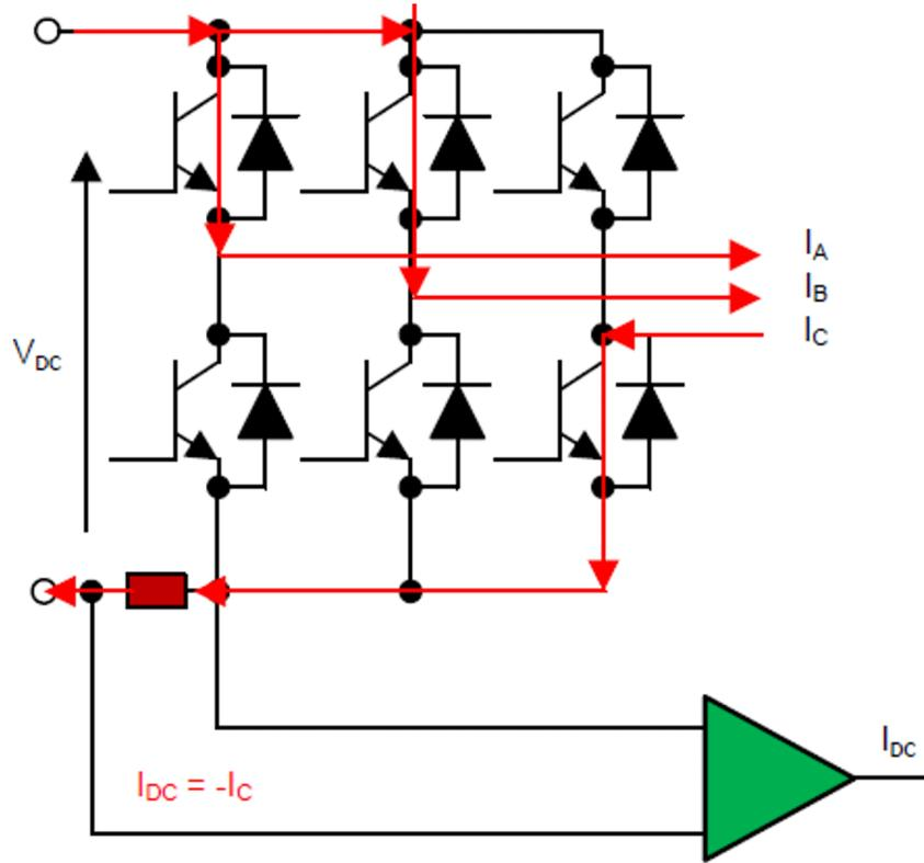
**Figure 2-9. Switching State Sa, Sb, Sc: 110**
