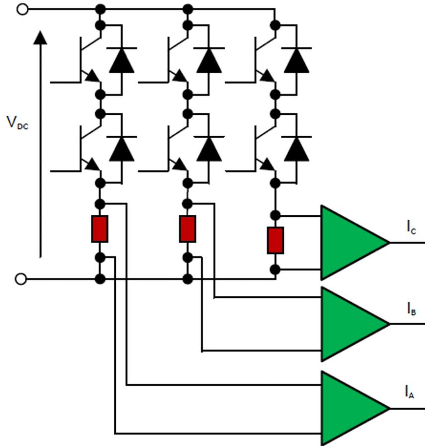
Figure 2-3. Three-Shunt Current Measurement Circuit With Inverter
