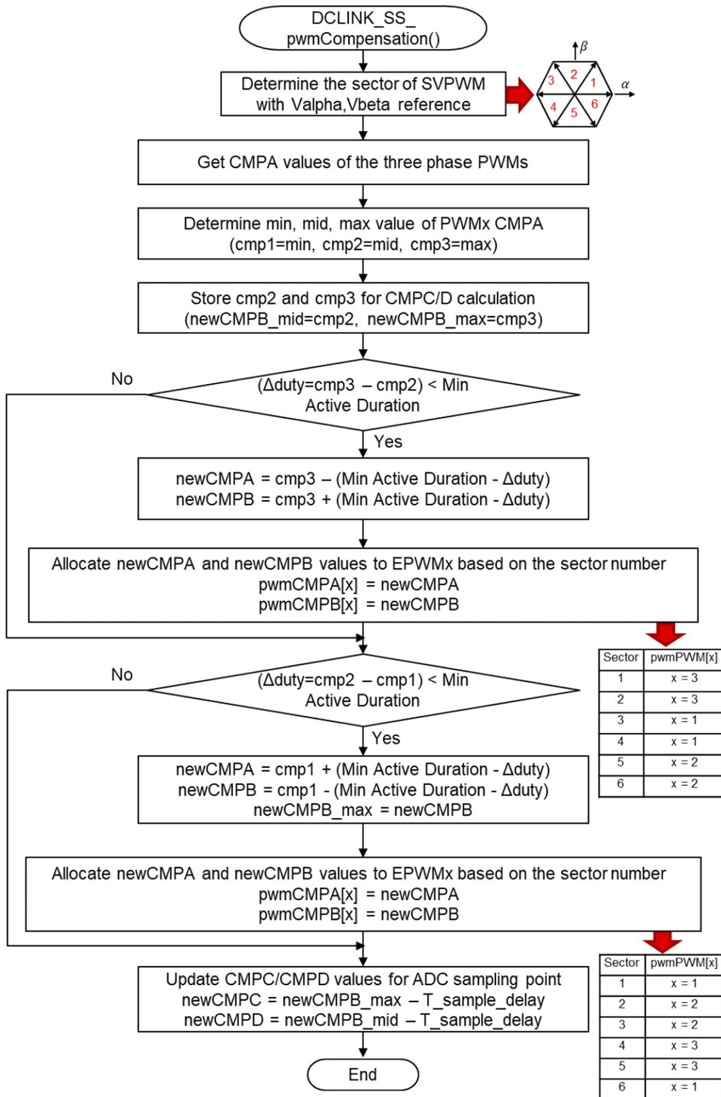
Figure 3-4. Flowchart of PWM Phase Shift Compensation
