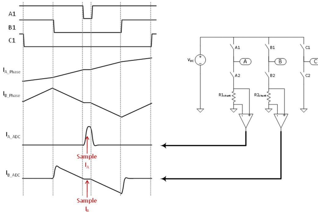
**Figure 2-6. Sampling Current When Using Two-Shunt Measurement Technique**
