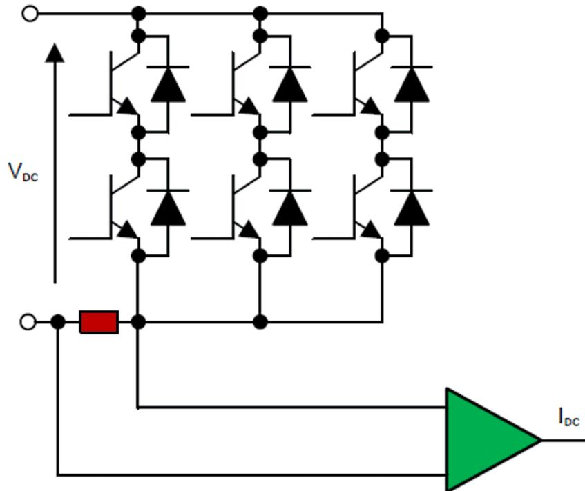
**Figure 2-7. Single-Shunt Current Measurement Circuit With Inverter**
