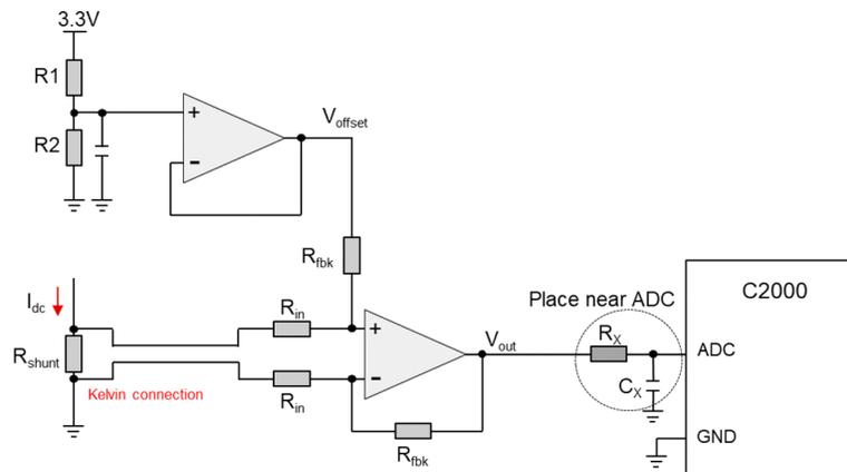
Figure 5-2. Current Sensing Circuit for F2802x With External Op-Amp
