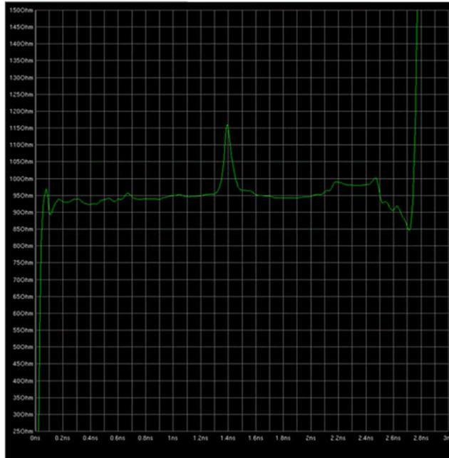
**Figure 3-1. TDR Plot Example With Impedance Mismatch**
