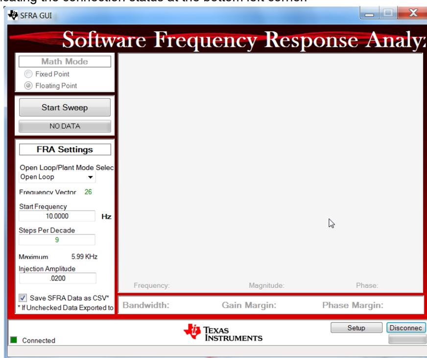
**Figure 11-5. SFRA GUI Connected to the C2000 MCU**
