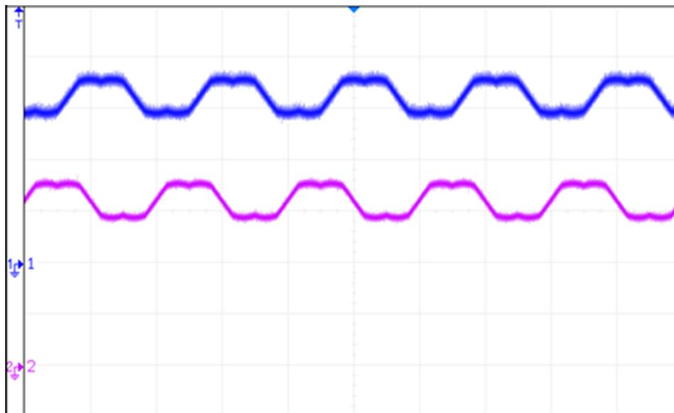
**Figure 6-4. DAC Outputs Showing Ta, Tb Waveforms**
