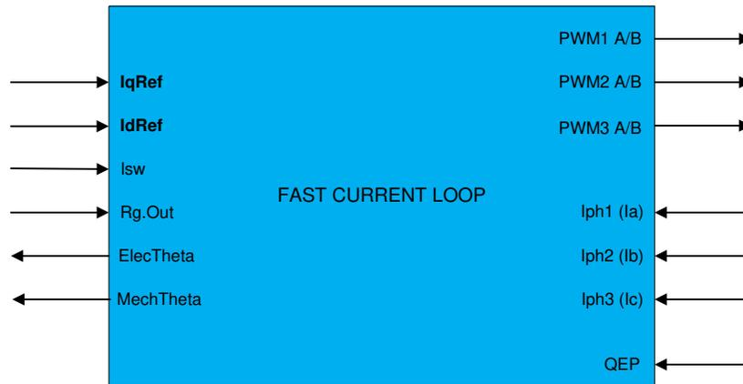
**Figure 4-2. Fast Current Loop Library Block Diagram**
