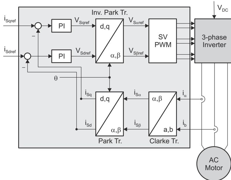
**Figure 3-1. Basic Scheme of FOC for AC Motor**
